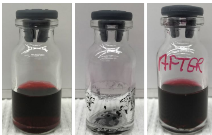
Fig. 10. Visual observation of Au-PEI@NIST at each step of lyophilization-reconstitution cycle; (left) original suspension (before cycle), (middle) lyophilized material, and (right) reconstituted suspension after full cycle (resuspended in DI water). The reconstituted material shows similar characteristic translucent red color implying stable unaggregated AuNPs in this size range.
