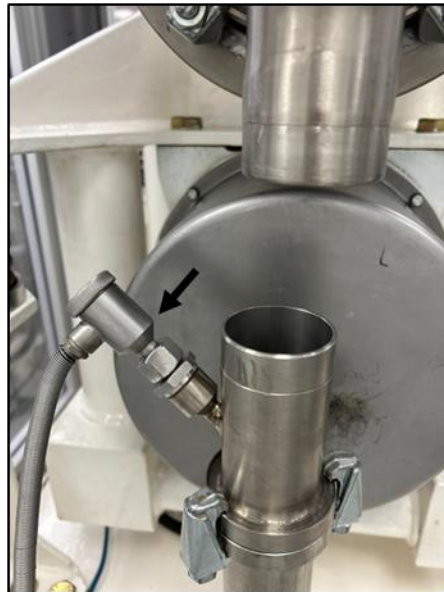
Figure 15. Temperature probe (indicated by the arrow) secured to the Temperature Pick-Up
