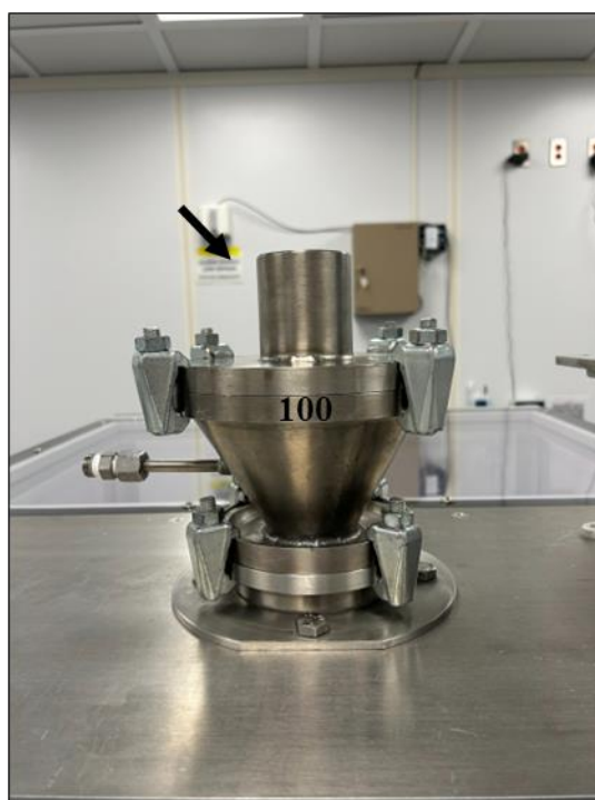
Figure 22. Inlet socket cover (indicated by the arrow)
