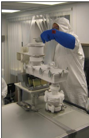
Figure 35. Cryomilling with the Vibrating Trough Conveyor
