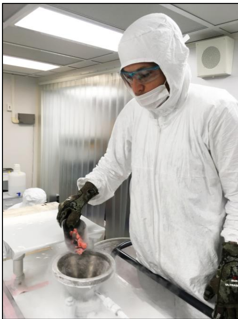
Figure 34. Cryomilling without the Vibrating Trough Conveyor
