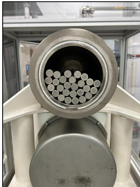
Figure 11. Titanium rods in the Material Grinding Chamber
