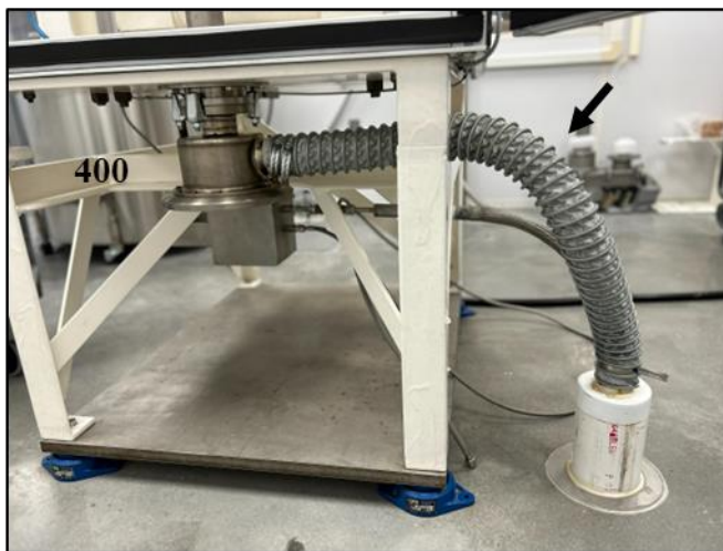
Figure 18. Exhaust hose (indicated by the arrow) connected to the Outlet Tube
