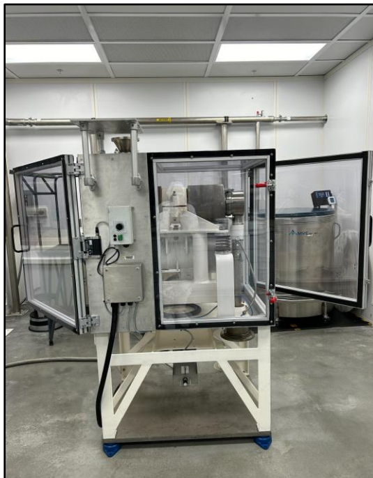
Figure 9. Cryomill with safety enclosure doors open
