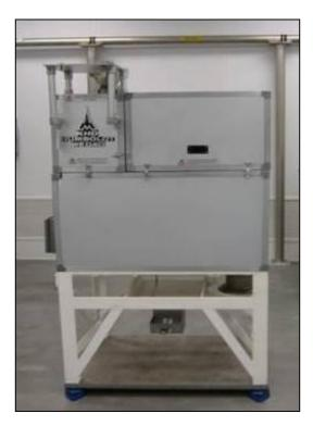
Figure 1. Palla VM-KT Vibrating Cryomill
