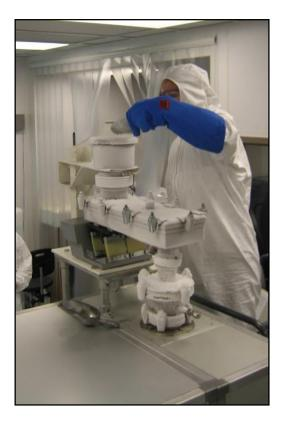
Figure 30. Cryomilling with the Vibrating Trough Conveyor
