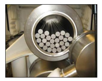
Figure 3. Titanium Rods contained inside Material Grinding Chamber
