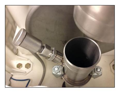
Figure 12. Outlet Tube and Temperature Pick-up
