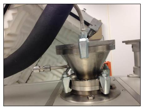
Figure 26. Flexible LN<sub>2</sub> Supply Line Attached to Inlet Socket
