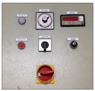
Figure 29. Cryomill Electrical Control Panel
