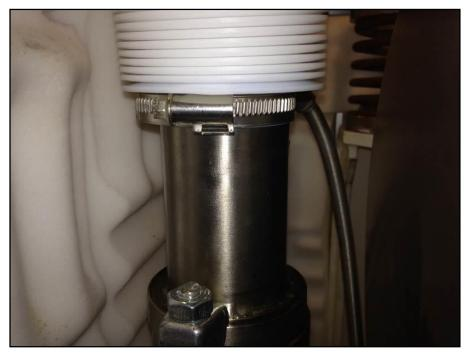
Figure 14. Outlet Bellow Lower Metal Band
