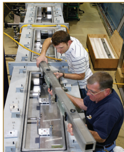
Mike Rinehart (bottom) and Doug Ogg of the NCNR carefully remove the neutron guides from the NG3 SANS instrument in preparation for its move to NGB.
