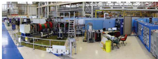
FIGURE 1: The Neutron Spin Echo spectrometer in its new location on NG-A in the guide hall extension. (Photo credit: Yiming Qiu)
