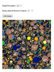
Backscattered Electron Contrast: Selecting yes from the pull-down menu will display a gray-scale image of the microstructure in which the relative brightness of each phase corresponds approximately to what would be observed in a backscattered electron image of a polished section using a scanning electron microscope.
