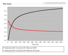
**Note**: When plotting multiple properties on the same graph, the properties must all have commensurate units. For example, both the degree of hydration and the total porosity are dimensionless quantities, so they can be plotted together. However, the degree of hydration and isothermal heat release have different units, so they cannot be plotted simultaneously. The pull-down menu selectors automatically exclude incommensurate properties.
