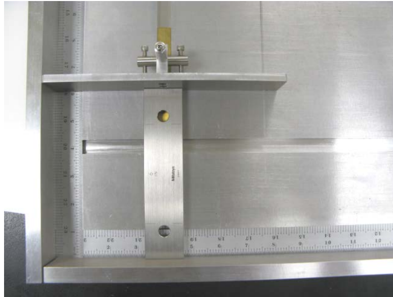
Figure 2: Vertical slide calibration check
