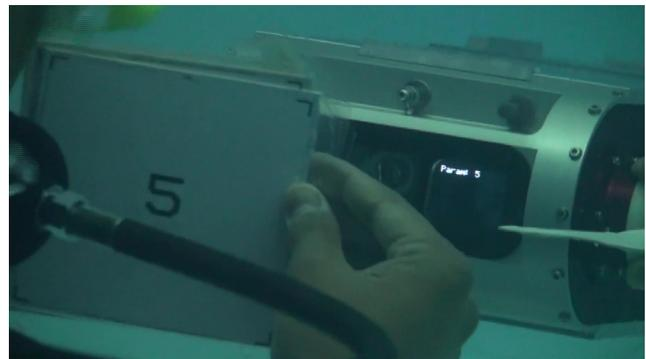
(b) Example of command acknowledgement given on the LED screen of the the Aqua robot during field trials.
