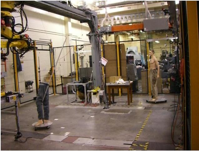
**Figure 8. Robot testbed with mannequins moved into places selected randomly by computer.**
