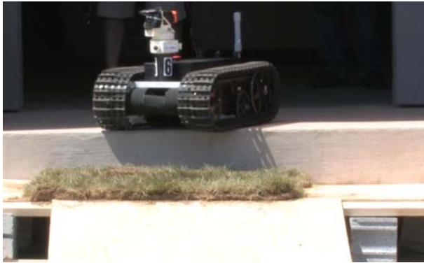
**Figure 20. Talon approaches a drop-off to sod.**
