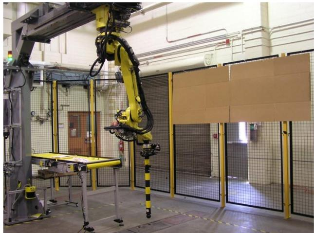
Figure 1 Under-slung Robot under Rail
