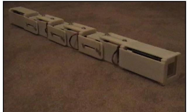
**Figure 15. FDM Fabricated MSIR Prototype**
