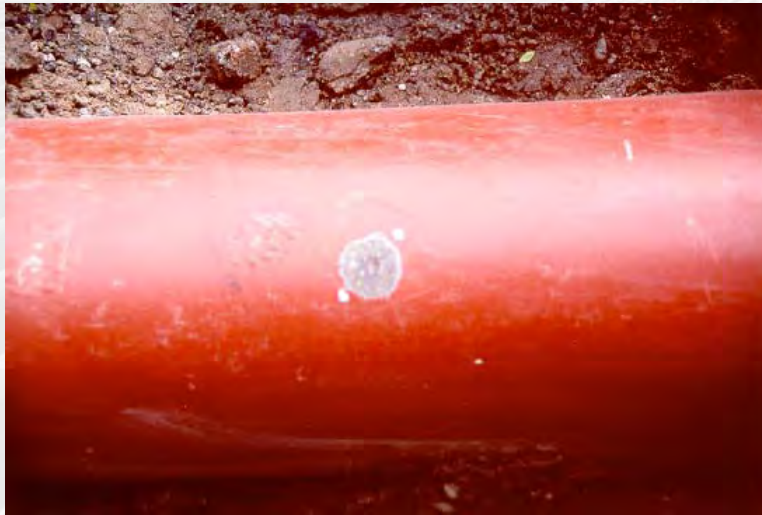
Photograph 3: Disbonded coating around holiday.
