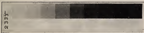
FIG. 18.—Test strip (slightly reduced) showing the nine densities due to exposure and the fog strip
