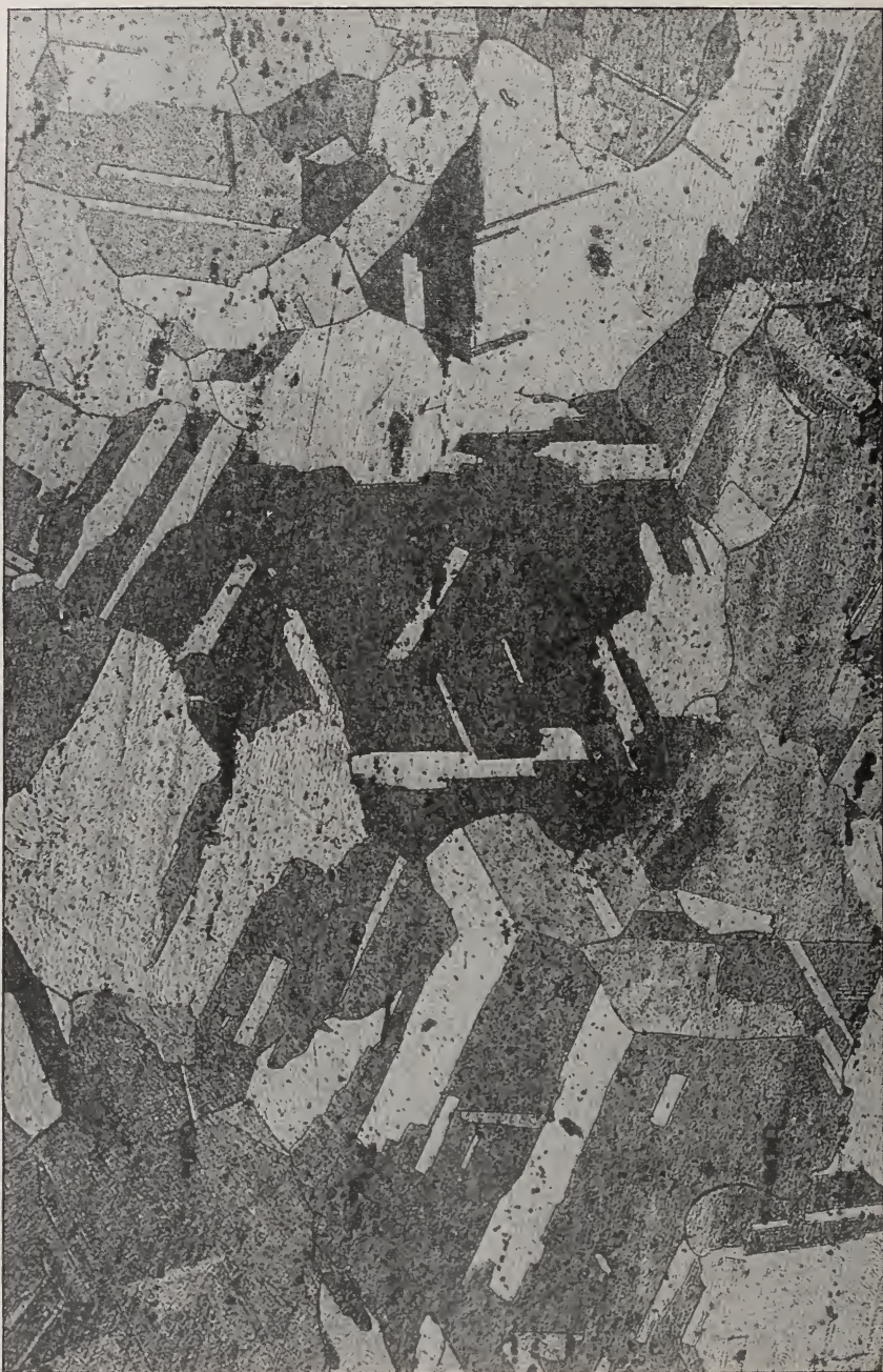
FIG. 1.—Structure of hot-rolled copper as revealed by etching with an ammoniacal solution of copper ammonium chloride. \times 250
