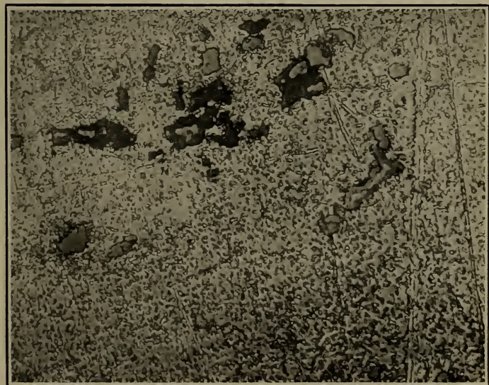
FIG. 23.—Sample of duralumin E 3-F, after annealing 20 hours at 500^{\circ} \text{C} ., quenching and aging at room temperature. \times 1000
