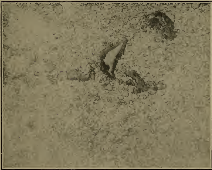
FIG. 19.— Rolled duralumin, N 34 (E4). Etched with 0.1 per cent NaOH. \times 1000
