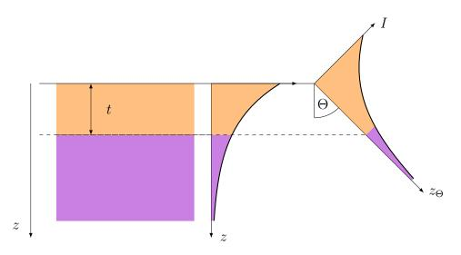
Figure 7.4: Visualization of the established model for layered specimens for two different emission angles  $\Theta$ . From the detector's point of view, the overlayer thickness *t* increases with the emission angle  $\Theta$ , which results in a higher fraction of detected overlayer electrons in direction  $z_{\Theta}$  than *z*.
