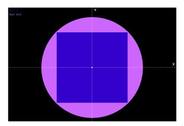
Figure 8.8: View of the xy plane at height z = 0 of the limiting body 600 for geometries with the single option. The substrate ranges from  $-7 \times 10^6$  Å to  $+7 \times 10^6$  Å in the x and y directions. The limiting body with the material specifier 600 is depicted in purple, while the substrate is depicted in blue. The circular shape of the circumference of the limiting body is given due to the nature of the PENGEOM implementation.
