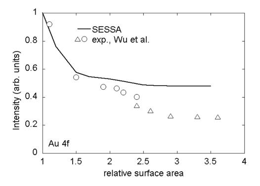
Figure 7.7: Au 4f intensity as a function of the relative surface area. Data points: experimental results from Wu *et al* [78, 79]; solid line: SESSA
