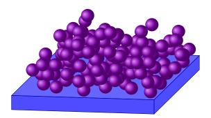
Figure 8.5: Schematic representation of a dispersed powder of core-shell particles. Nanostructures such as these can be generated by the scripts explained within this chapter
