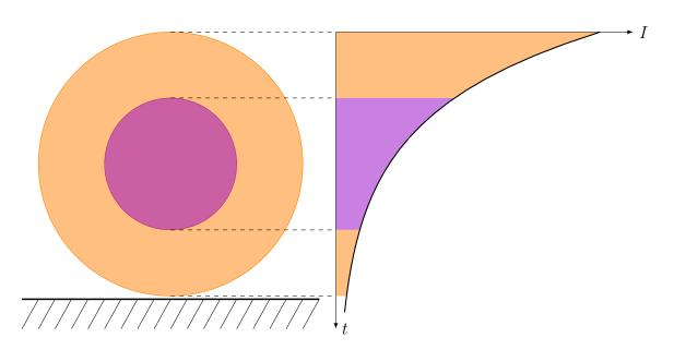
Figure 8.1: Cross-sectional visualization of the selected model for core-shell cylinders. Depending on the lateral position, the shell and the core or only the shell contribute to the signal I. The graph on the right schematically illustrates the contributions of the core and shell signals as a function of the depth t for vertical photoemission on a line through the center of the cylinder.
