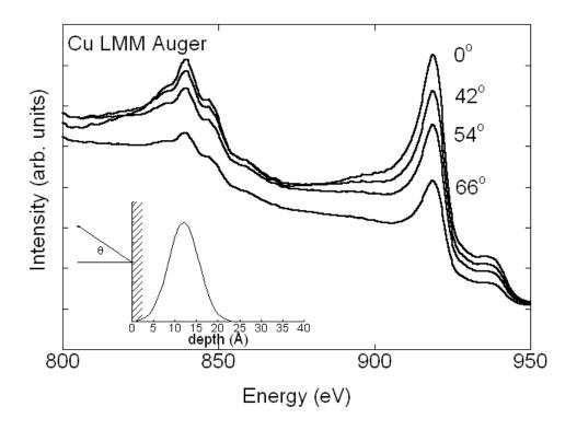
Figure 7.13: Cu LMM Auger spectra for different emission angles (with respect to the surface normal) and for the source depth distribution shown in the inset. These results simulate ion-induced Auger electron spectra.
