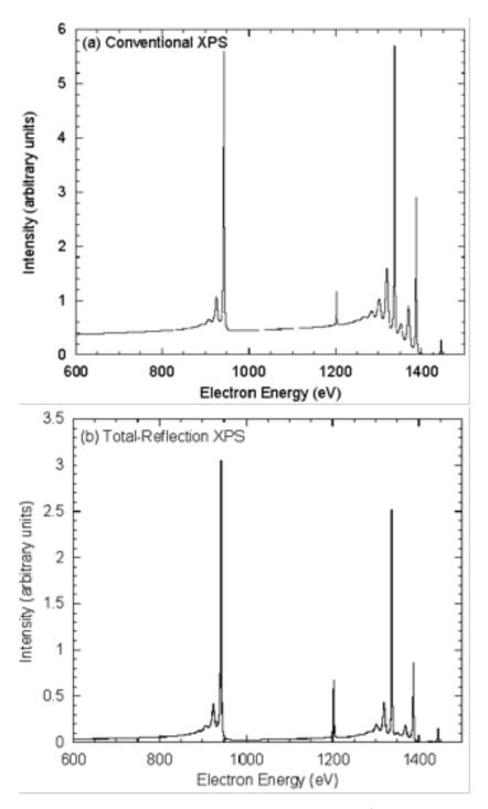
Figure 7.12: Simulated spectra of a sample consisting of a 0.5 Å thick C-contamination layer on top of a 10 Å thick SiO<sub>2</sub> layer on a Si substrate. The top panel shows the simulated conventional XPS spectrum, the bottom panel shows the simulated Total Reflection XPS spectrum, where the angle of incidence of the X-rays is close to the angle of total reflection. These spectra were simulated as described in the text.
