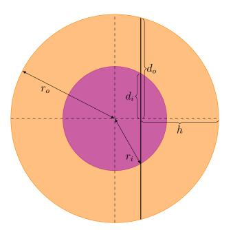
Figure 8.2: Illustration of the variables used to calculate the core and shell intensities for an infinite cylinder.  $r_i$  is the inner radius (core radius),  $r_o$  is the outer radius (total radius), h is the distance from the outer edge from the cylinder and is used as the integration variable and  $d_i$  and  $d_o$  are the local core and shell thicknesses along the source-analyzer-axis, respectively, as functions of h.
