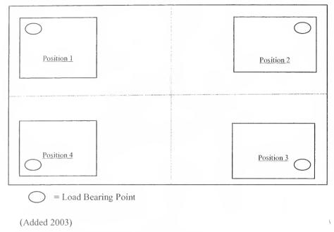
(a) A one-half nominal capacity test load centered as nearly as possible, successively at the center of each quarter of the load-receiving element as shown in the diagram below.
