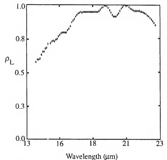
**Figure 10.** Relative spectral response  $\rho_L(\lambda)$  or “instrument function” for the extended-area source absolute calibration.
