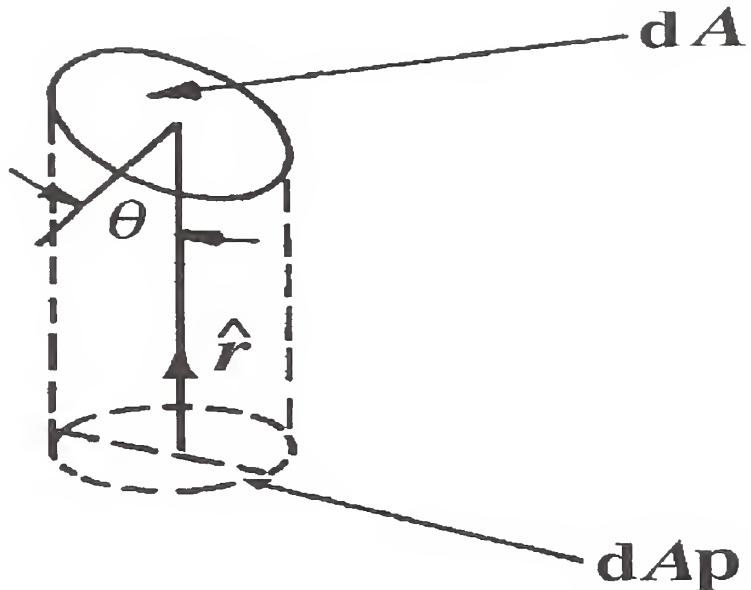
Figure 1. Illustration of the projected area.
