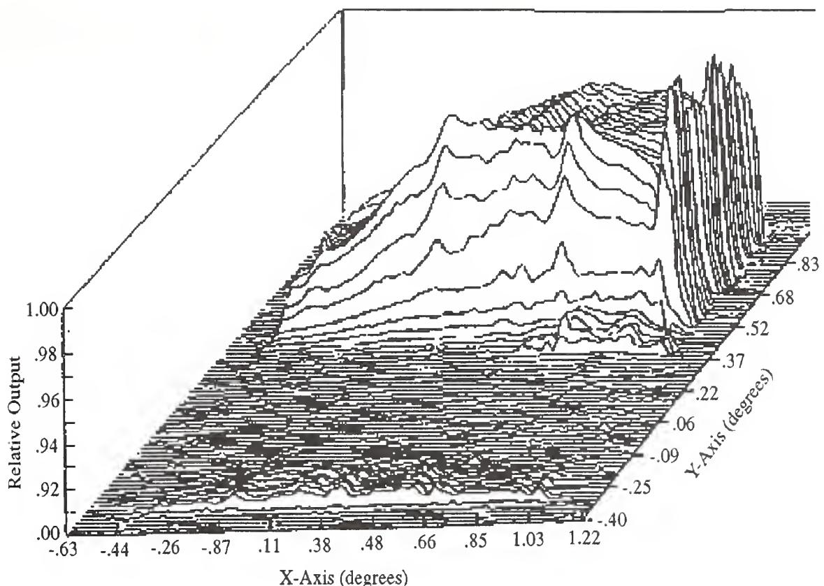
**Figure 6. Isometric 3 dimensional view of the spatial response of an infrared detector.**
