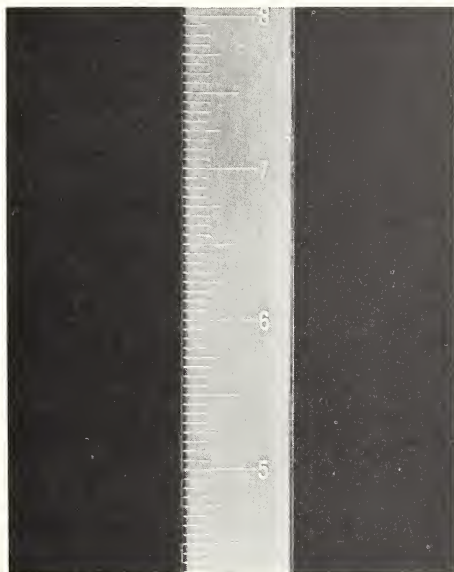
FIGURE 5. Gage rod with \frac{1}{16} -inch graduation.
