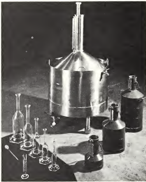
FIGURE 11. Volumetric standards—100, 10, 5, and 1-gallon gage-glass; ½-gallon, 1-quart, 1-pint, ½-pint, and 1-gill glass flasks, and 2-ounce graduated cylinder.
