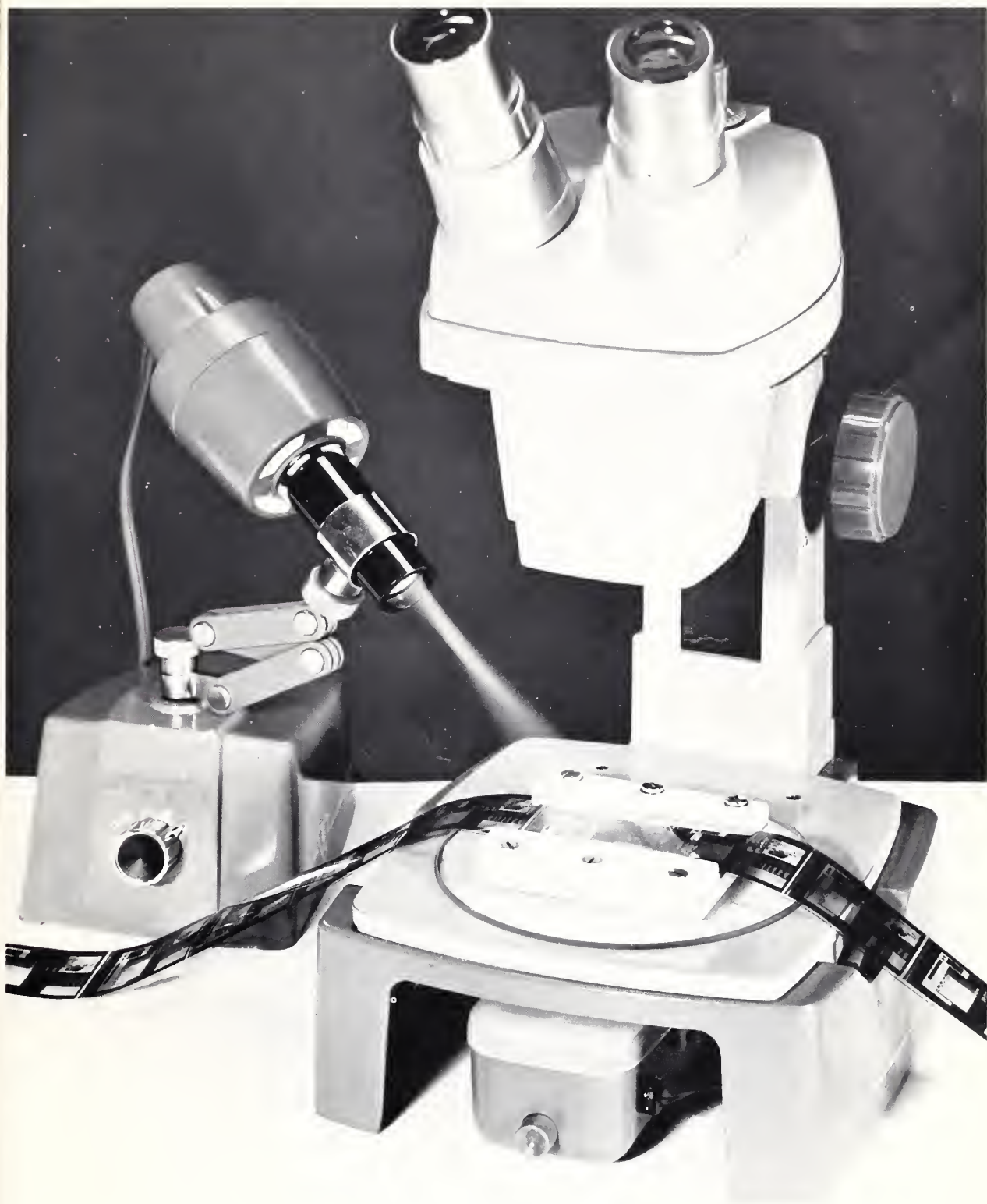
FIGURE 10. Microscope with illumination for viewing by reflected light.
