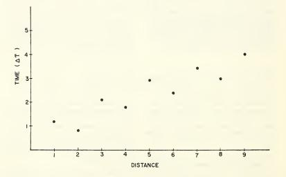
Figure 5-1. Time required for a drop of dye to travel between distance markers.
