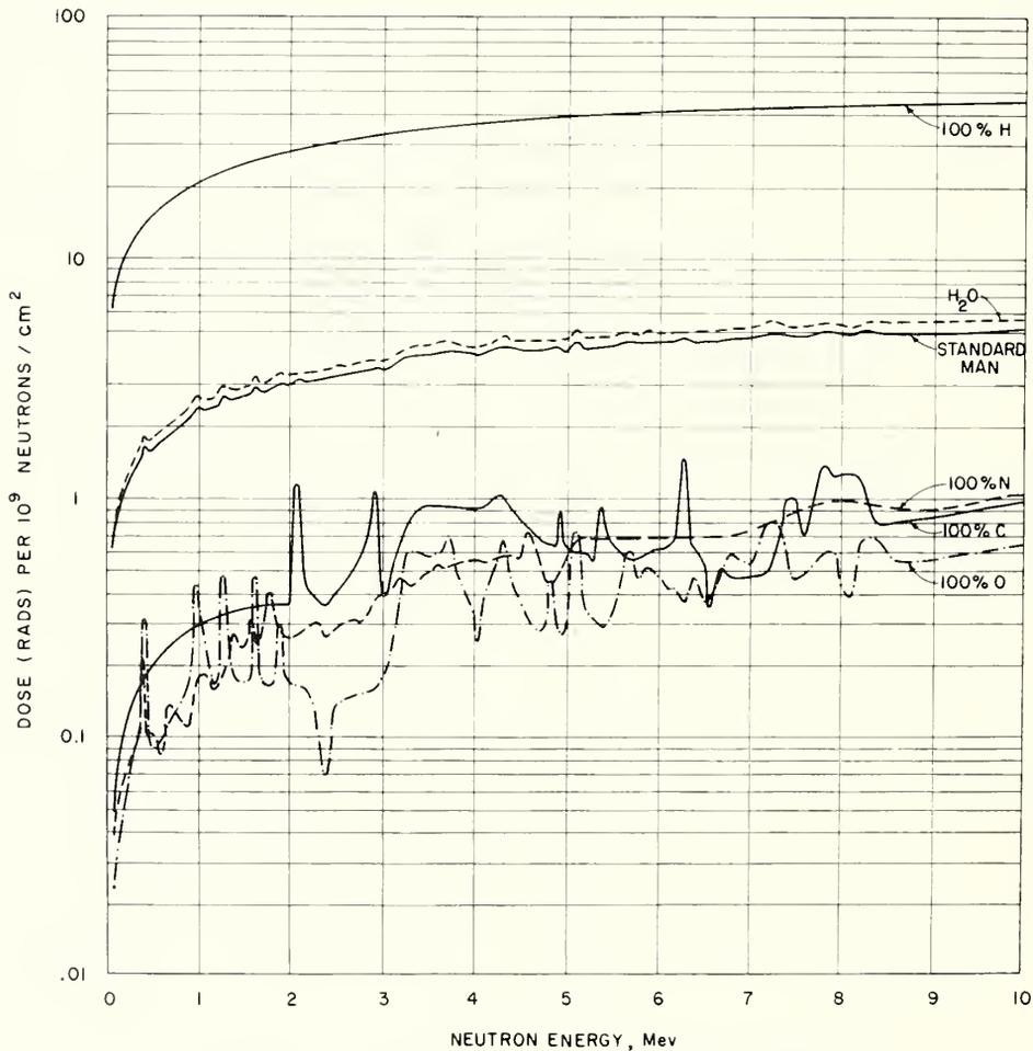
FIGURE 14. Absorbed dose delivered under equilibrium conditions by a time-integrated flux of  $10^9$  neutrons/cm<sup>2</sup> as a function of neutron energy.
