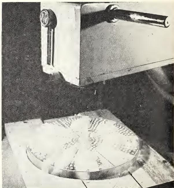
FIGURE 5. Apparatus suitable for exposing rats under conditions of maximal scatter, using a conventional x-ray therapy machine.
