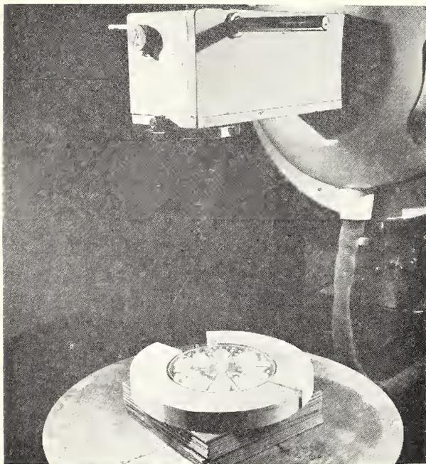
FIGURE 4. Apparatus suitable for exposing mice under conditions of maximal scatter, using a conventional x-ray therapy machine.
