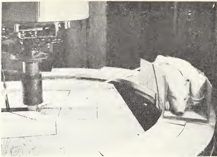
FIGURE 8. *A simple apparatus suitable for exposing swine or similar-sized animals, using the radial beam from a 250 kvp x-ray generator.*
