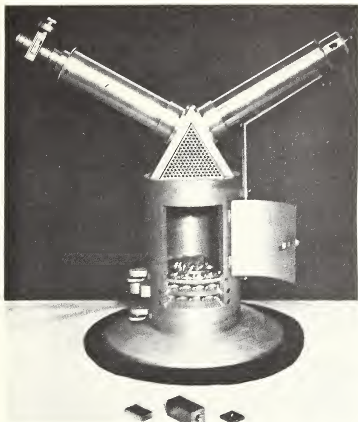
FIGURE 5. Photograph of the short-block interferometer.
