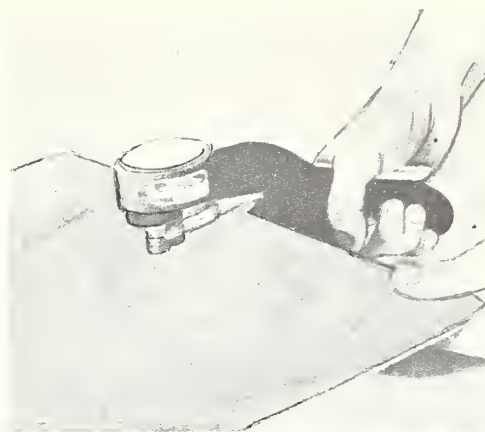
FIGURE 28. Sheet-metal dial micrometer.
