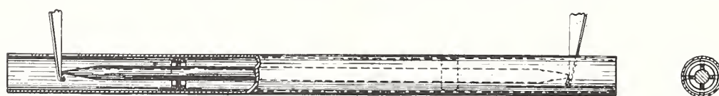
FIGURE 2. Sample, sample holder, and hinged fingers for wires in liquid bath.
