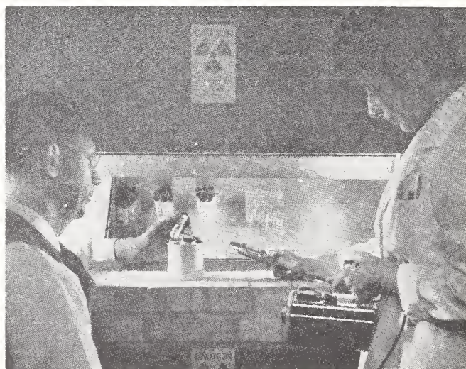
FIGURE 28. Radioactivity standards are stored in an outside brick room on shelves with brick and concrete lips having a thickness of 8 inches.
