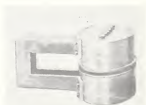
FIGURE 108. Measuring head of the Salford foil thickness gage.
