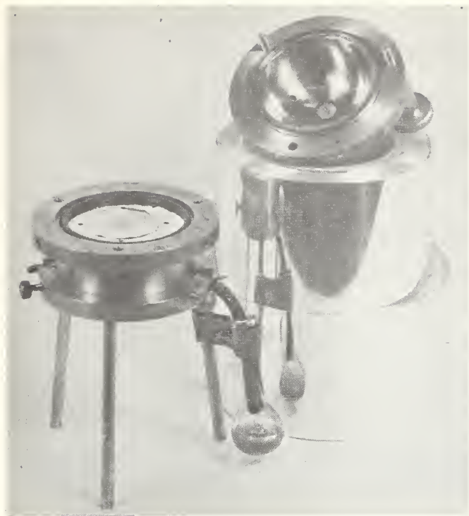
FIGURE 12. A closeup view of the 4\pi\beta -proportional counter in use at the National Bureau of Standards showing details of the source mounted on plastic supported by aluminum foil.
