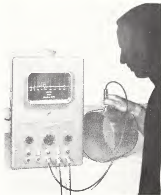
FIGURE 53. "Metroscope" thickness meter.
