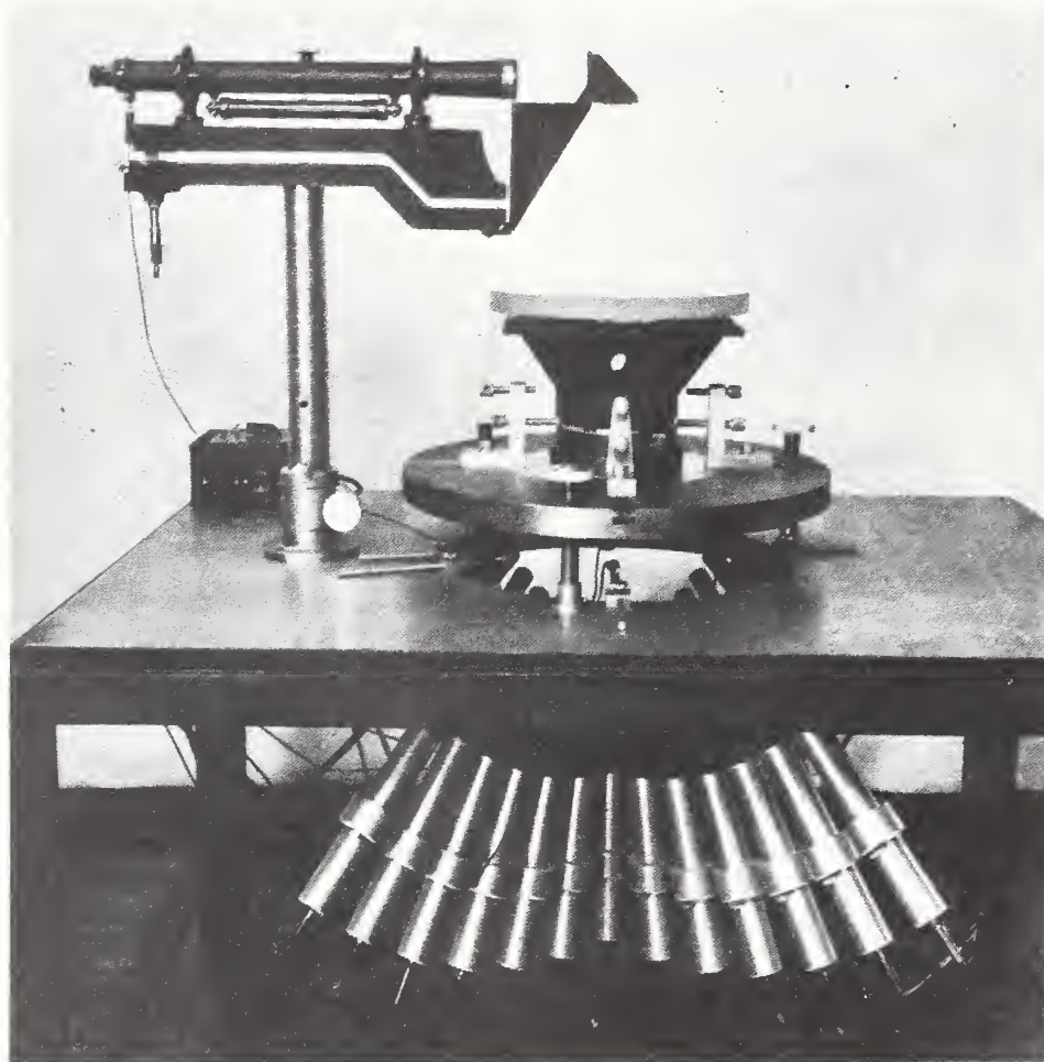
Fig. 3—Camera calibrator. Instrument as arranged for use. The camera under test points vertically downward. Its proper orientation is affected by the auto-collimating telescope and the plane-parallel piece of glass placed on the focal plane of the camera. Images on a finished negative appear every 7.5^\circ along each diagonal, with the collimation index marks registered on each side of the negative.
