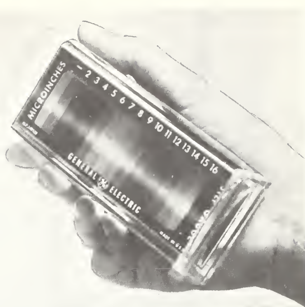
FIGURE 122. Step gage to measure thickness of molecular films.
