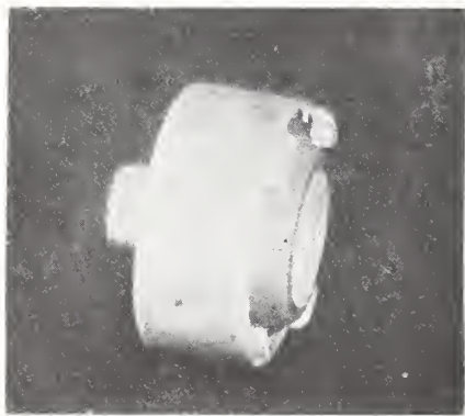
FIGURE 51. Crystal transducer searching unit.
