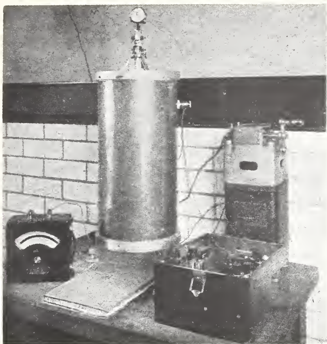
FIGURE 4. Fused-quartz tube and dial indicator thermal-expansion apparatus.
