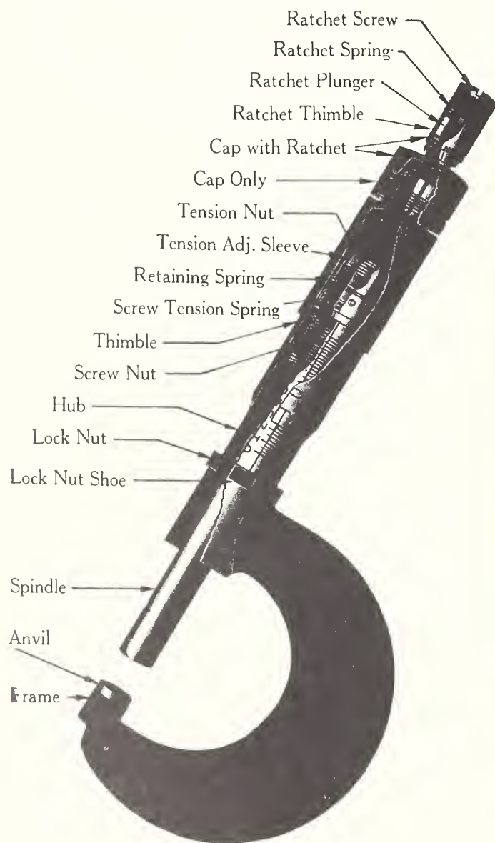
FIGURE 12. Micrometer caliper.
