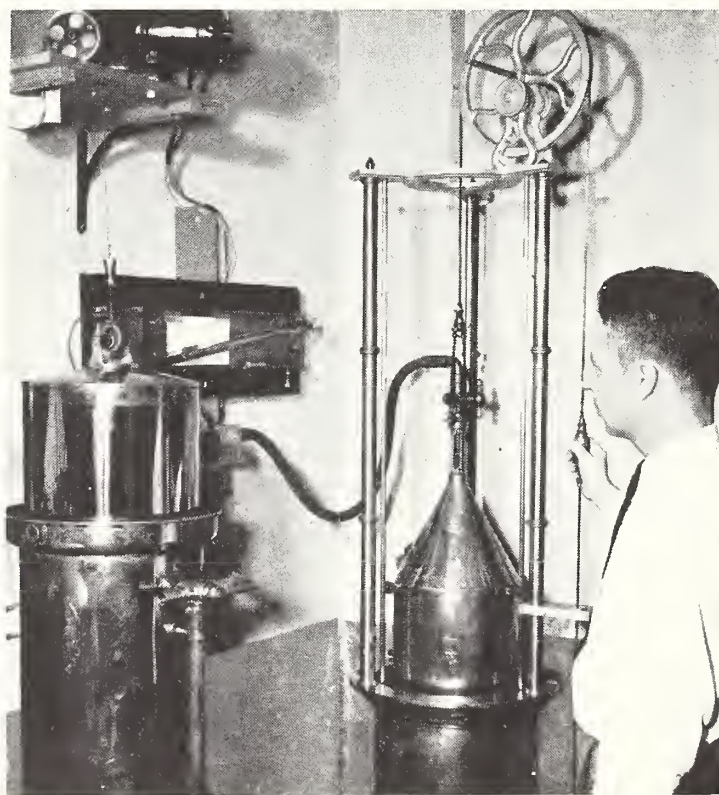
FIGURE 8. Calibration of a capacity standard at NBS.
