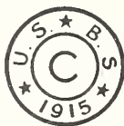
FIG. 8.—Seal for class C weights
