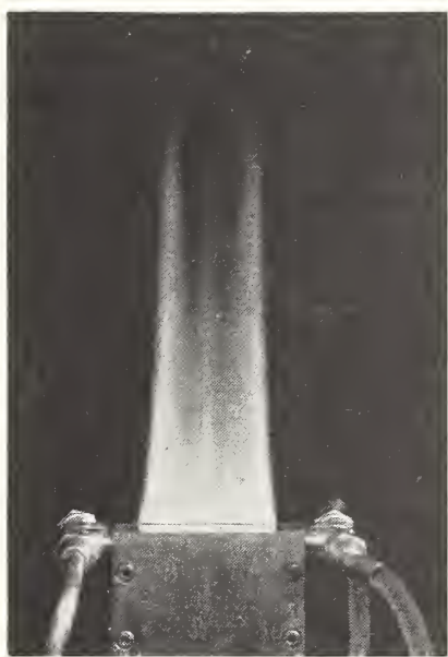
FIG. 2. Photograph of flame on slot burner. The reaction zone is the small bright line just above the burner. The remainder of the luminous zone is due to the hot gases in which there is little chemical reaction.
