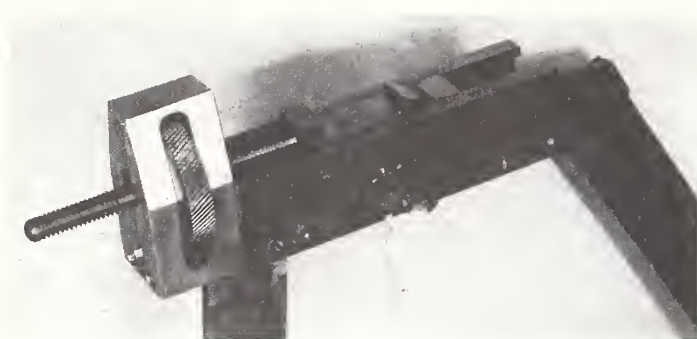
FIGURE 4. Clamping device for locking in position the rotating arm.
