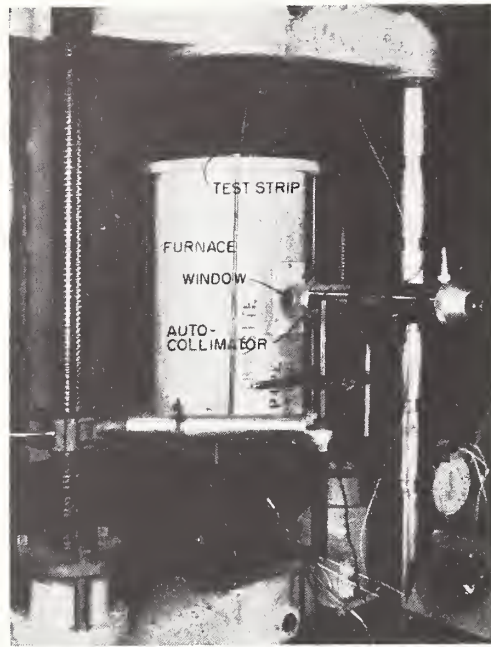
FIG. 3.—Test Equipment for Gage Factor Determination.
