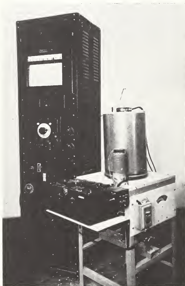
Fig. 2. Photograph of Pt-Rh resistance furnace and control equipment.
