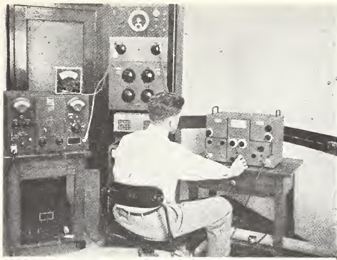
FIGURE 1. Calibration of the internal attenuators and linearity of a commercial field-strength meter.
