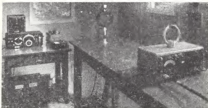
Fig. 13—"Standard-field" equipment assembly to determine loop antenna coefficients.
