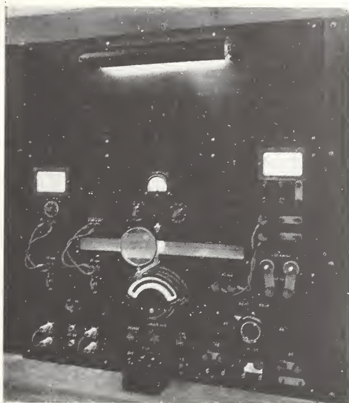
FIGURE 5. Instrument testing panel, including Lindeck element.
