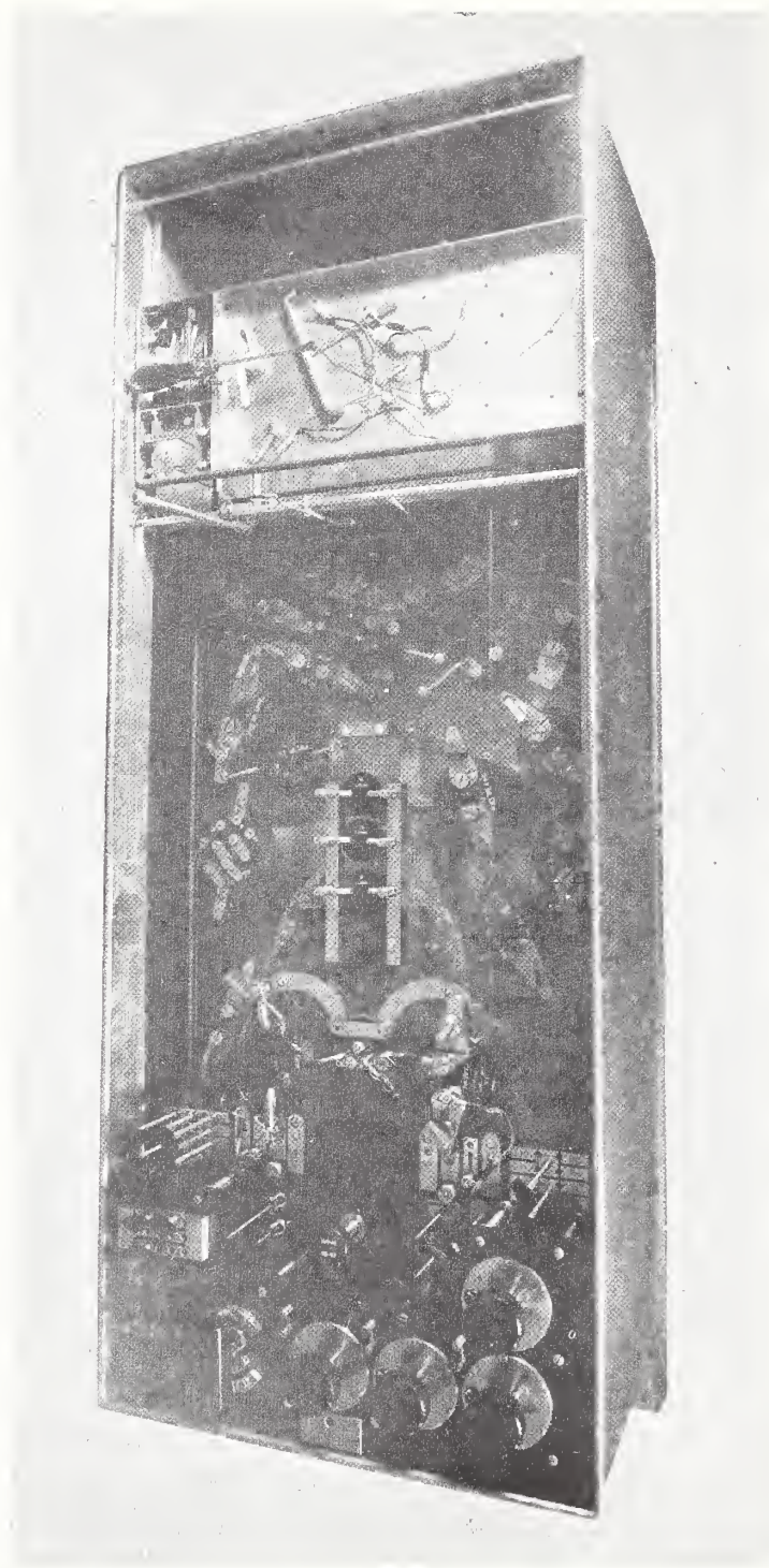
FIGURE 7.—General view of the NBS precision bridge and oil bath.
