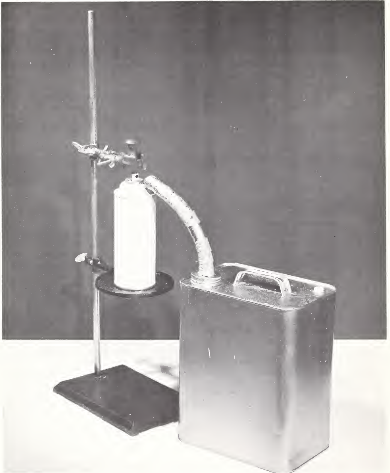
Fig. 1. A lightweight, portable test stand with an adjustable valve-actuator depressor and a receiving vessel. (Component list, assembly, and operation described on the facing page.)
