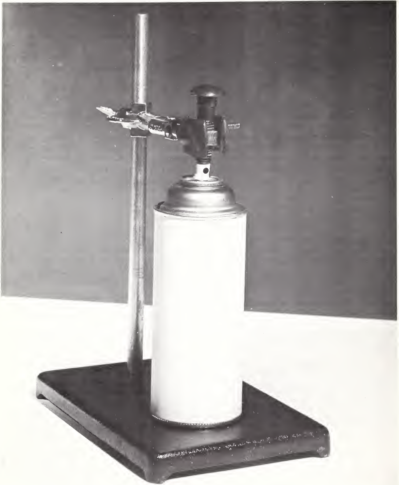
Fig. 1. A light weight portable test stand with an adjustable valve-actuator depressor. (Component list, assembly, and operation described on the facing page.)
