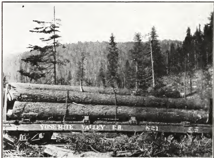
FIG. 27.—Use of adjustable log bunks; chains used only as an added precaution. (Rule 157.)
