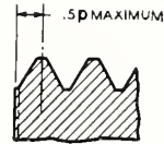
FIGURE 6.18. Start of perfect thread on gage.
