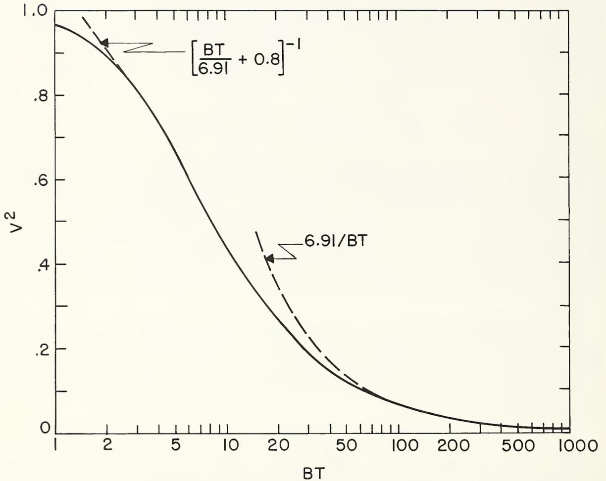
Figure 32. Normalized variance,  $(\langle (p^2)^2 \rangle - \langle p^2 \rangle^2) / \langle p^2 \rangle^2$ , where  $\langle \rangle$  denotes the average taken over all room locations, of the mean-squared sound pressure in a room having a reverberation time,  $T$ , and excited by random noise of bandwidth,  $B$ . The curve corresponds to eq. (85) which is valid for modal overlaps greater than about 3.
