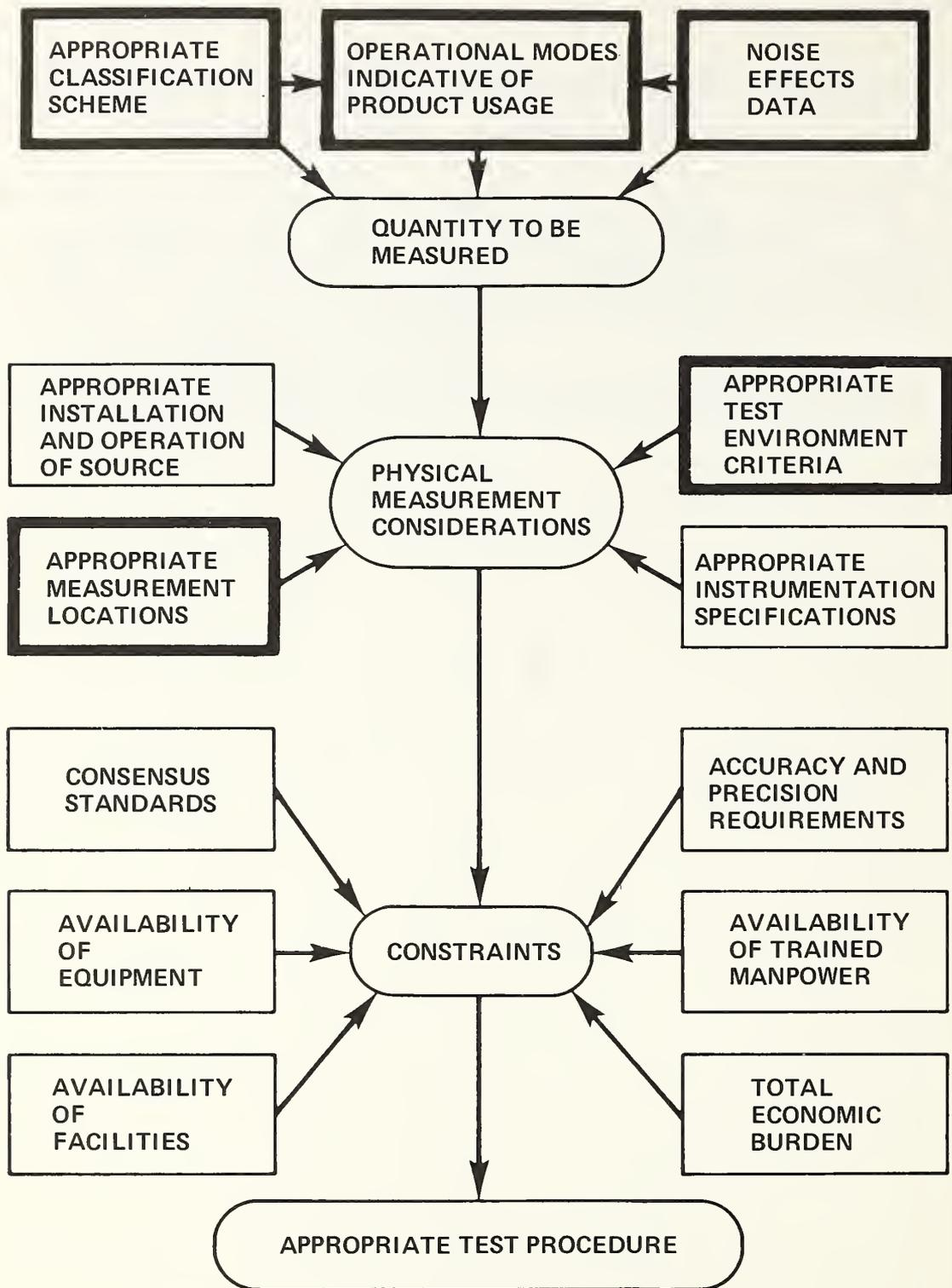
Figure 35. Development of appropriate test procedure.
