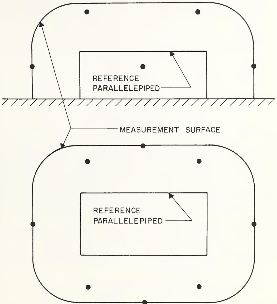
Figure 30. Microphone array for a "composed" measurement surface[13].
