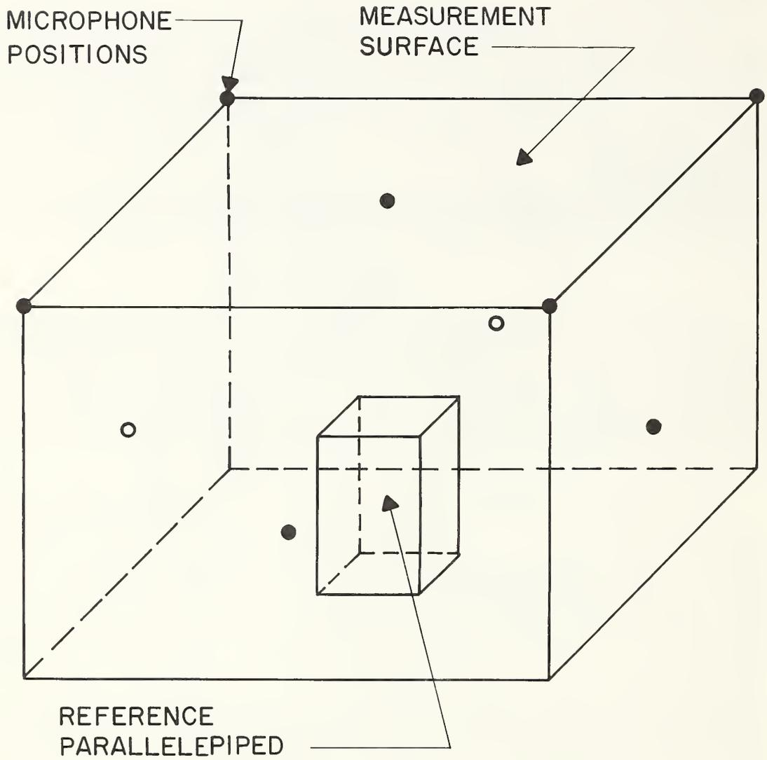
Figure 29. Microphone array for a parallelepiped measurement surface[13].
