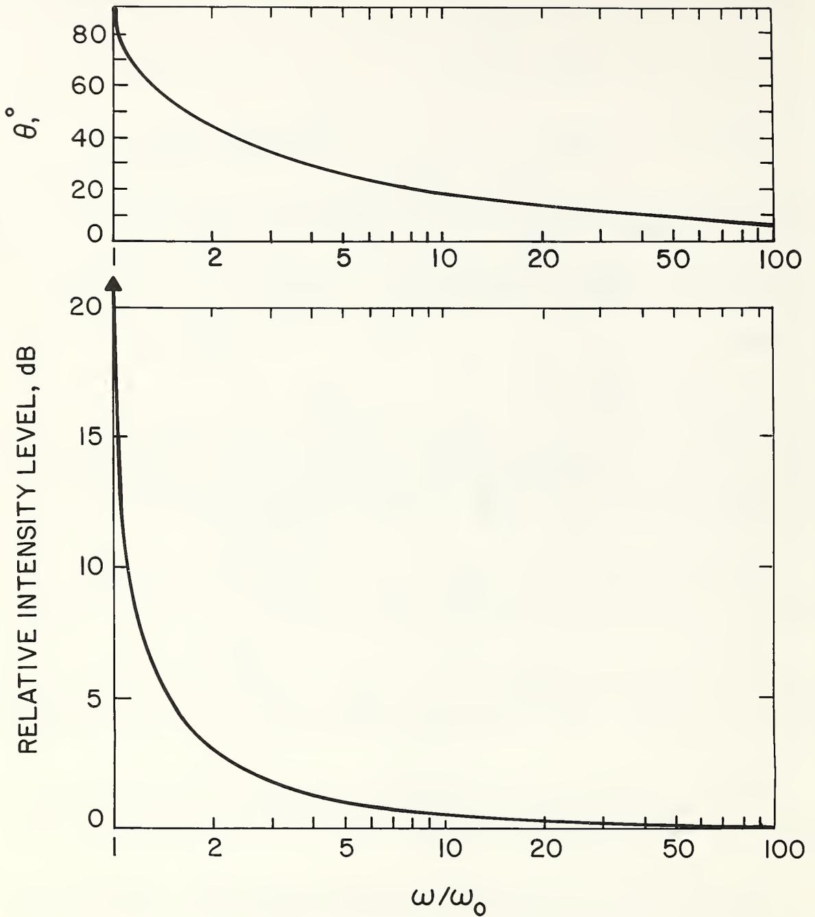
Figure 23. Far-field intensity level (lower figure) above the critical frequency for an infinite plate in flexure. The upper figure shows the direction (relative to the plane of the plate) in which sound is radiated.
