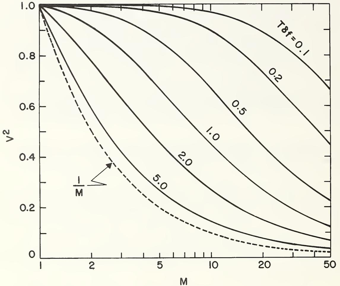
Figure 34. Normalized variance of the mean-squared sound pressure in a room, having a reverberation time,  $T$ , excited by  $M$  equal-strength pure tones uniformly separated in frequency by  $\delta f$ . The curves correspond to eq. (92) which is valid for modal overlaps greater than about 3.
