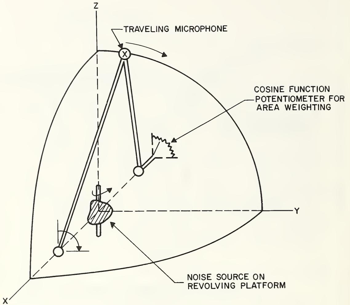
Figure 28. System for microphone traverses along meridional paths[14].
