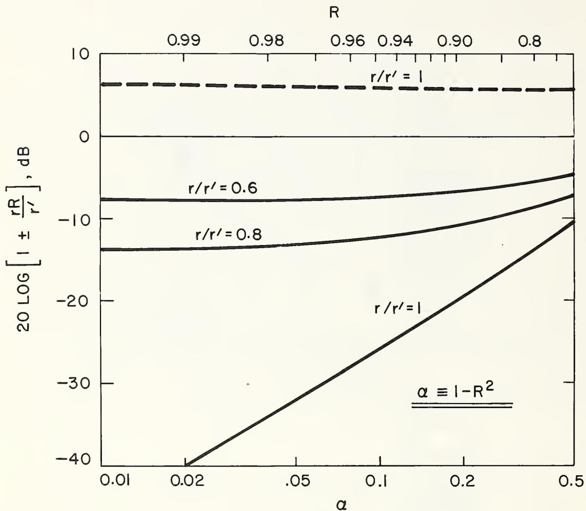
Figure 7. Limits for the effect of the image source (see Figure 6) on the observed sound pressure level as a function of the absorption coefficient of the reflecting plane with  $r/r'$  as a parameter. The solid lines correspond to destructive interference while the dashed line corresponds to constructive interference.
