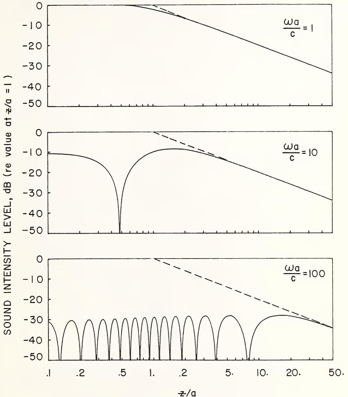
Figure 19. Variation of the axial intensity level due to a baffled rigid piston of radius,  $a$ , vibrating at an angular frequency,  $\omega$ . The dashed lines represent extrapolations of the far-field intensity level back toward the source.
