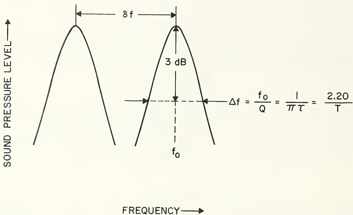
Figure 13. Drawing illustrating the spacing,  $\delta f$ , between normal modes, the width,  $\Delta f$ , of a normal mode, and the relationships among  $\Delta f$ ,  $f_0/Q$ ,  $\tau$ , and  $T$ .
