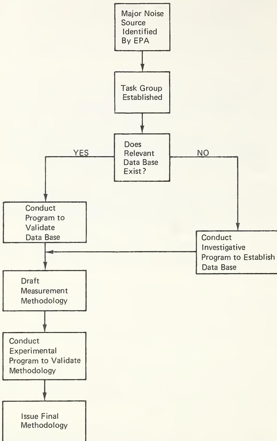
Figure 2. Recommended operational procedure for generating measurement methodologies.
