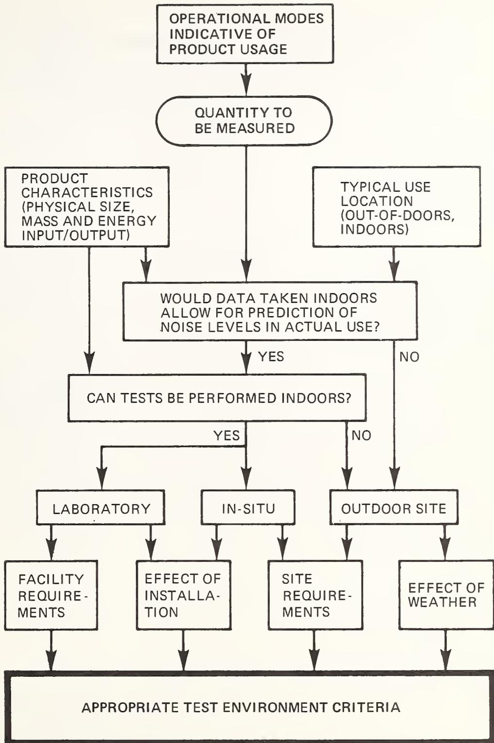
Figure 40. Selection of appropriate test environment criteria.
