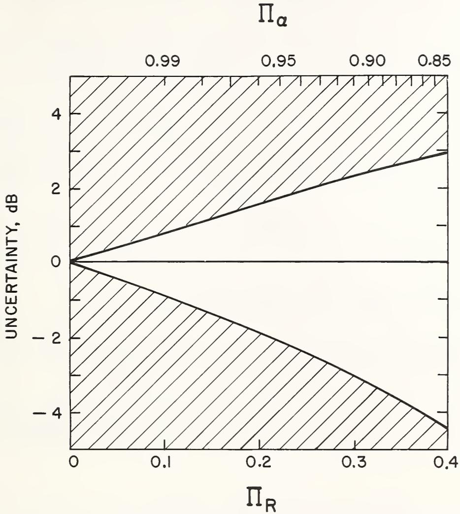
Figure 4. Maximum range of uncertainty in the sound pressure level in an anechoic chamber as a function of  $\Pi_R$  and  $\Pi_\alpha$ , defined in the text (for single wall, normal incidence).
