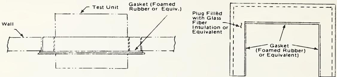
Fig. 3 Typical sound isolation plug
