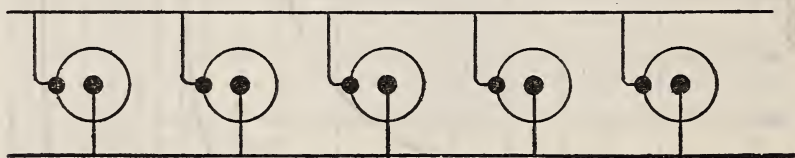
FIG. 7.—Cells connected in parallel.
