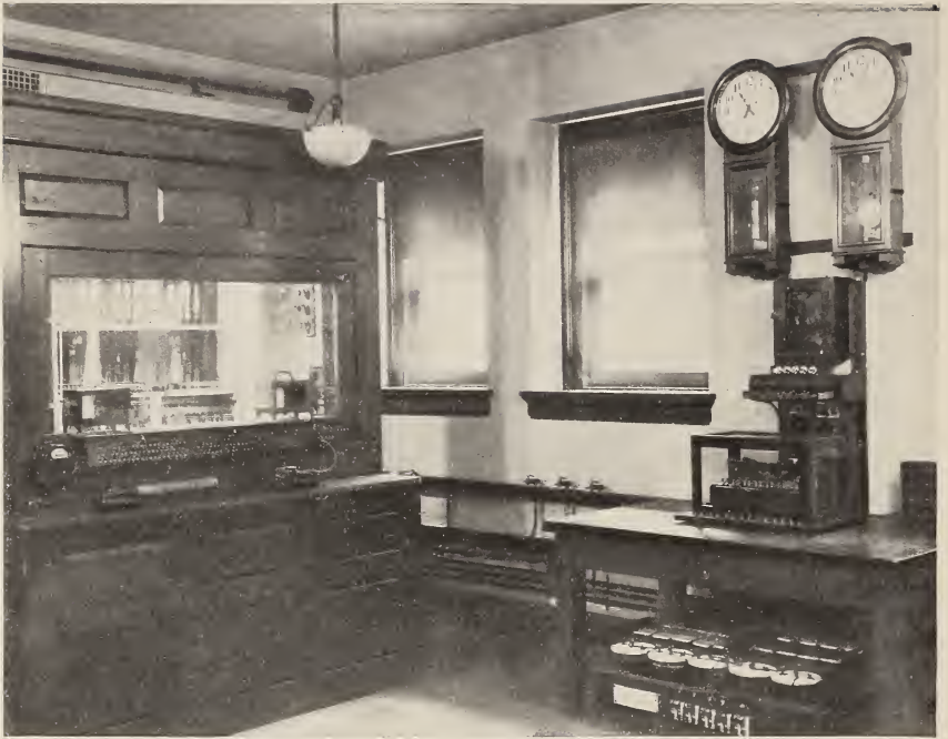
FRONTISPIECE.— Automatic apparatus for controlling the intermittent tests of dry cells.
