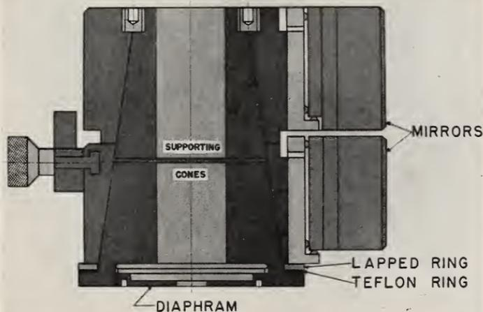
FIGURE 3. *Cross section of angle mirror assembly.*
