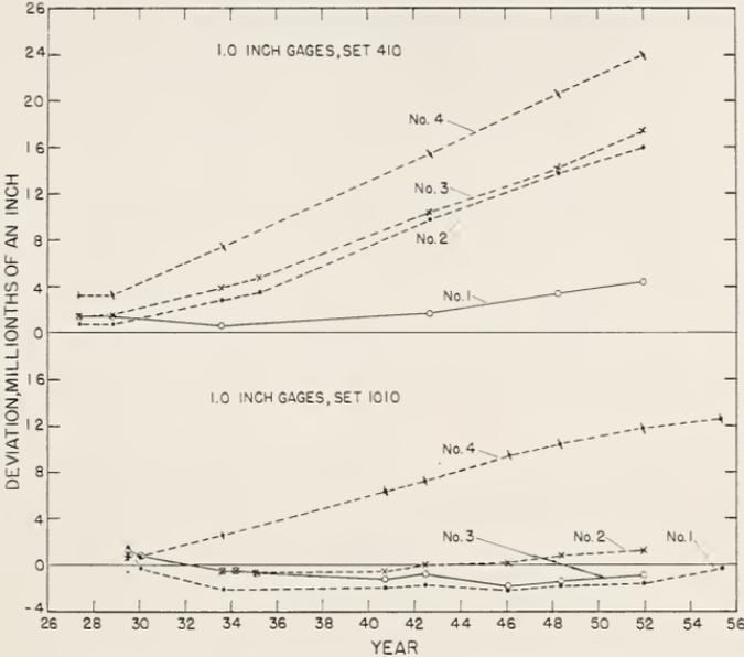
FIGURE 1. Length changes of 1-inch gage blocks.
