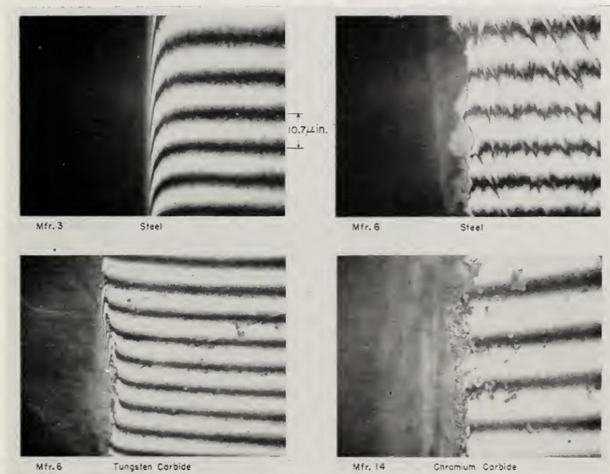
FIGURE 9. Edge conditions on grade AA gage blocks.
