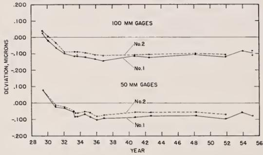
FIGURE 4. Length changes of 100- and 50-millimeter gage blocks.
