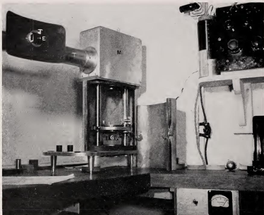
FIGURE 1. *Fizeau-type interferometer.*
