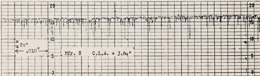
FIGURE 5. Graph of microfinish on grade A and AA tungsten carbide gage blocks.
