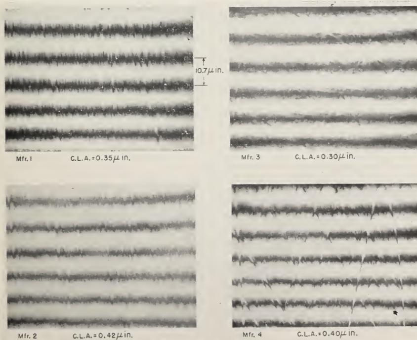
FIGURE 2. *Microfinish on grade A steel gage blocks.*
