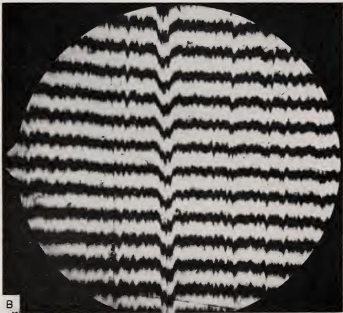
FIGURE 6. *Microinterferograms of ground steel surface A and lapped steel surface B.*
