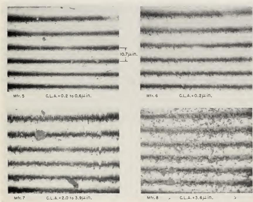
FIGURE 4. Microfinish on grade A and AA tungsten carbide gage blocks.
