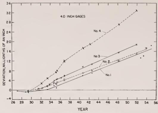
FIGURE 3. Length changes of 4-inch gage blocks.
