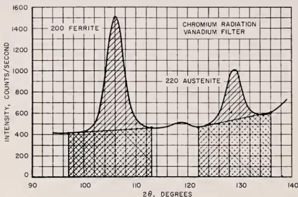
FIGURE 5. Retained austenite measurement.
