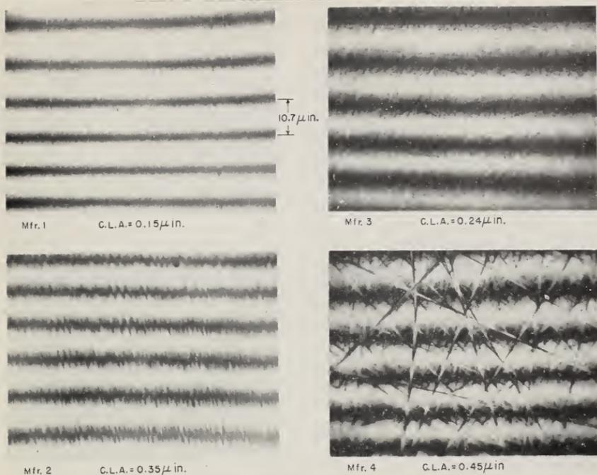
FIGURE 1. *Microfinish on grade AA steel gage blocks.*
