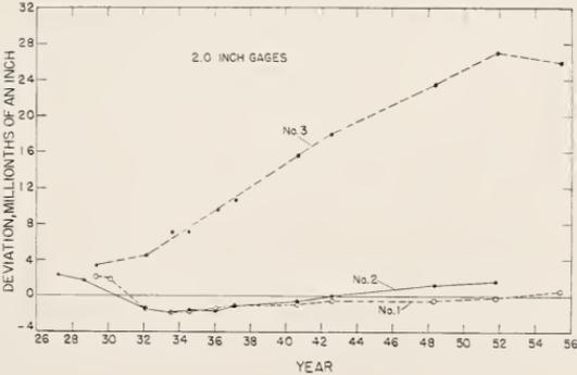
FIGURE 2. Length changes of 2-inch gage blocks.
