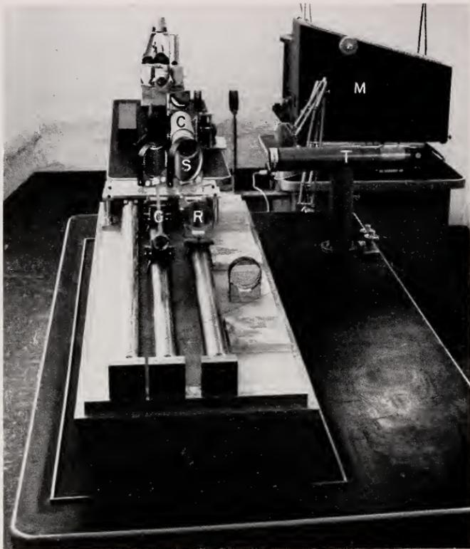
FIGURE 3. Michelson-type interferometer for long lengths.
