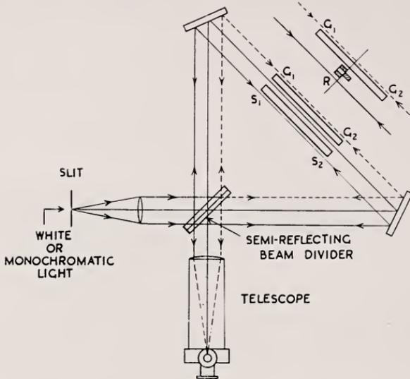
FIGURE 12. Diagram of optical arrangement of Hilger double-ended gauge interferometer.
