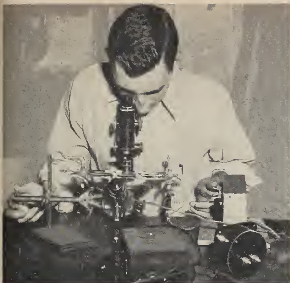
FIGURE 4. Mobility measurement of collagen particles using horizontal electrophoretic cell.
