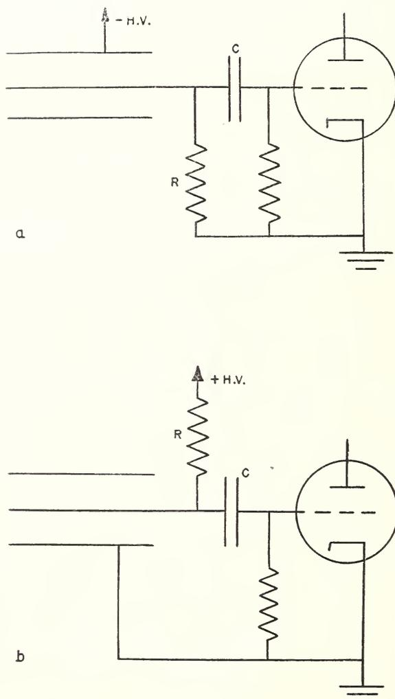
FIGURE 22. Methods for connecting counters to the high voltage.
