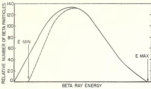
FIGURE 13. The typical form of a beta-ray spectrum (solid curve) in relation to the portion transmitted by a thin absorber (dotted) curve.
