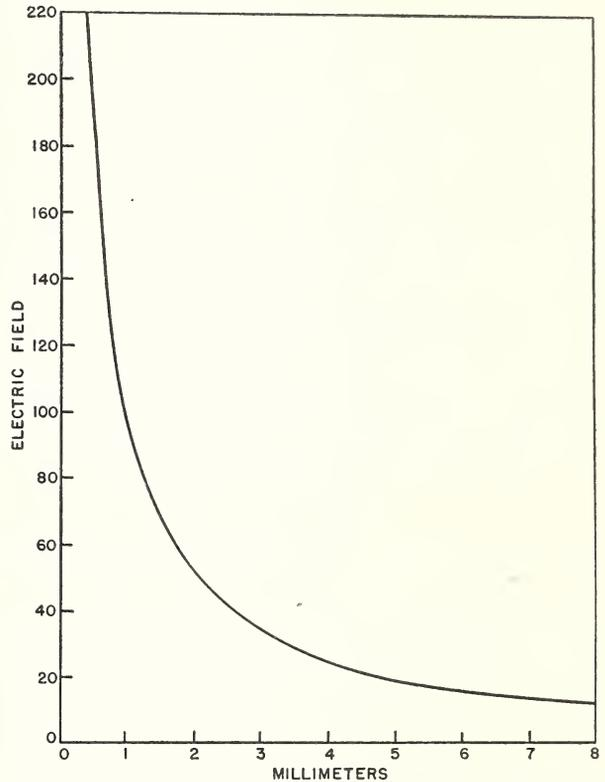
FIGURE 2. Variation of the electric field with distance from the axis of the center wire.
