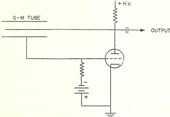
FIGURE 5. Quenching circuit of Neher and Harper for rapid extinguishing of the counter discharge in permanent gas counters.
