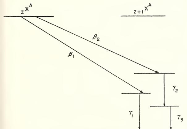
FIGURE 26. Typical disintegration scheme for a radioisotope of atomic number  $Z$  and mass number  $A$  which disintegrates by emission of beta rays,  $\beta_1$  and  $\beta_2$  of two different maximum energies to form the radioisotope of atomic number  $Z + 1$  and mass number  $A$ .
