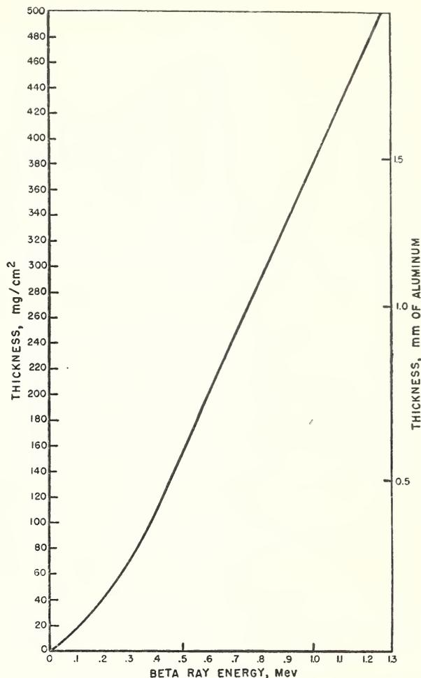
FIGURE 12. Maximum range of beta particles of various energies.
