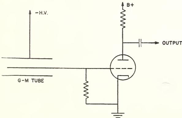
FIGURE 6. The Neher-Pickering quenching circuit.
