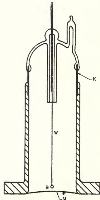
FIGURE 16. End-window beta-ray counter.
