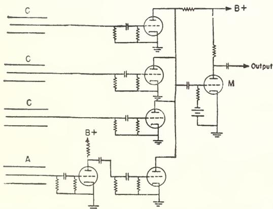
FIGURE 32. *Anticoincident circuit; CCC=coincidence counters, A=anticoincidence counter.*
