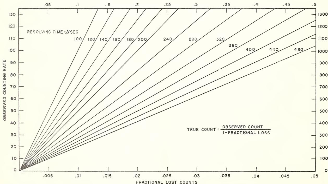
FIGURE 25a. Fractional lost counts for different resolving times and for a wide range of observed counting rates. The true counting rate is equal to observed counting rate as shown on the y-axis multiplied by (1-Fractional Lost Counts) where the fractional lost counts is read on the x-axis for the resolving time in question.
