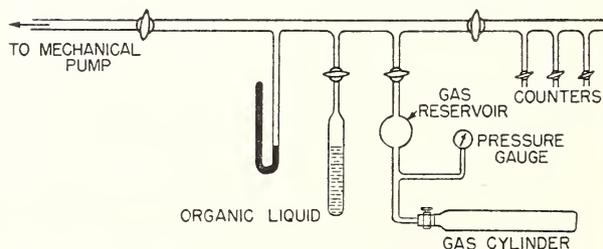
FIGURE 37. A typical system for filling counters.
