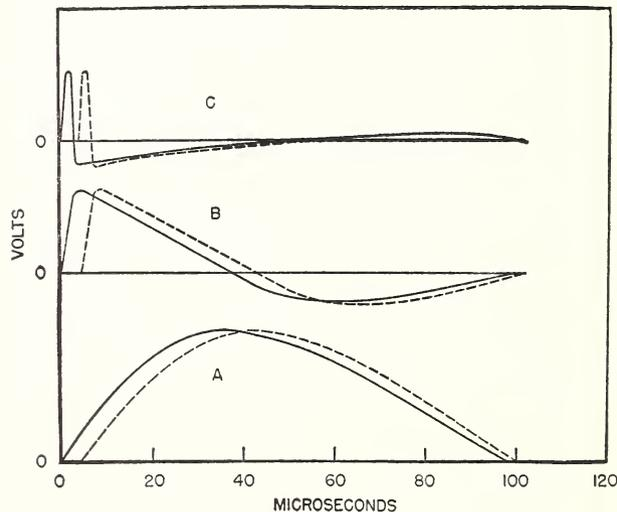
FIGURE 30. Diagram of the successive differentiation of an electrical pulse.
