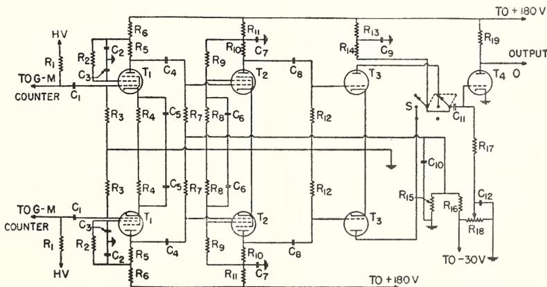
FIGURE 31. Wiring diagram of a coincidence circuit using electrical differentiation for sharpening the pulses.
