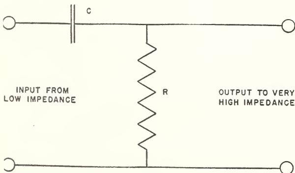
FIGURE 29. Diagram of a filter circuit for electrical differentiation of a pulse.
