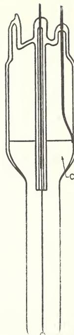
FIGURE 18. Dipping counter for measuring beta rays from solutions.
