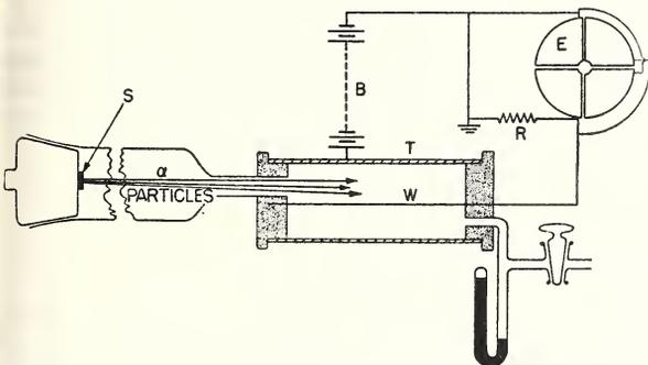
FIGURE 1. Apparatus used by Rutherford and Geiger for electrical counting of alpha particles.
