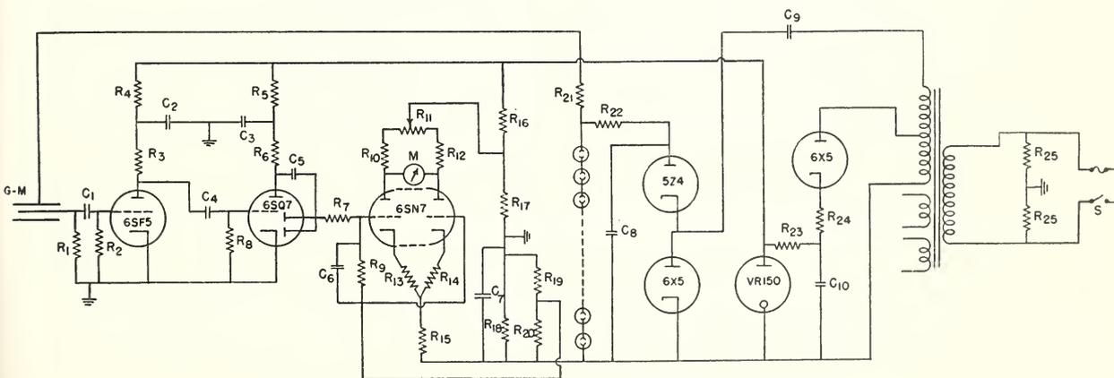
FIGURE 23. Wiring diagram for counting-rate meter.
