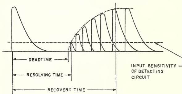
FIGURE 8. Diagram showing the deadtime and subsequent gradual recovery of pulse size.
