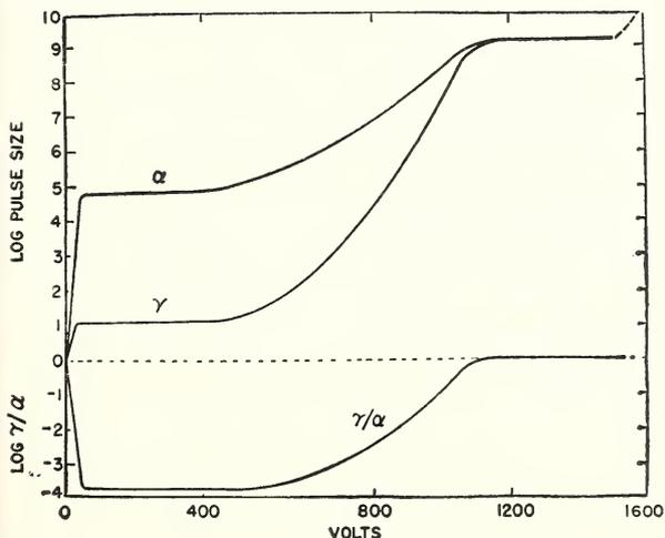
FIGURE 33. Curves showing the relation of pulse sizes from alpha particles and gamma-ray photons for various voltages on a counting tube.
