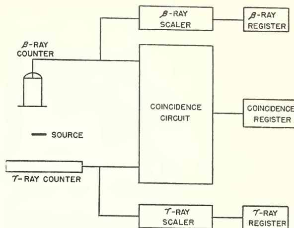
FIGURE 27. Block diagram of a coincidence circuit for determining coincidences between beta and gamma rays.
