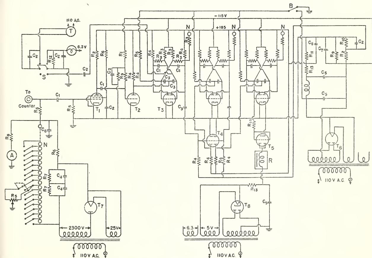
FIGURE 21. Wiring diagram of a complete scaler having a ratio 1:16 showing high voltage rectifying circuit, electrical timer and output stage with recorder.
