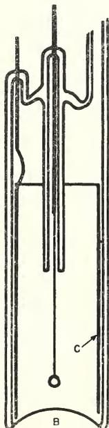
FIGURE 17. Bubble-window beta-ray counter.
