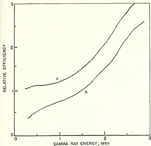
FIGURE 11. Relative efficiencies of platinum- and copper-tube counters.
