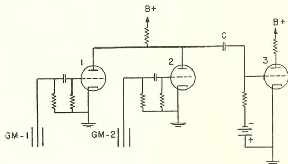
FIGURE 28. Basic Rossi circuit for determining coincidences between two Geiger-Müller counters, GM-1 and GM-2.
