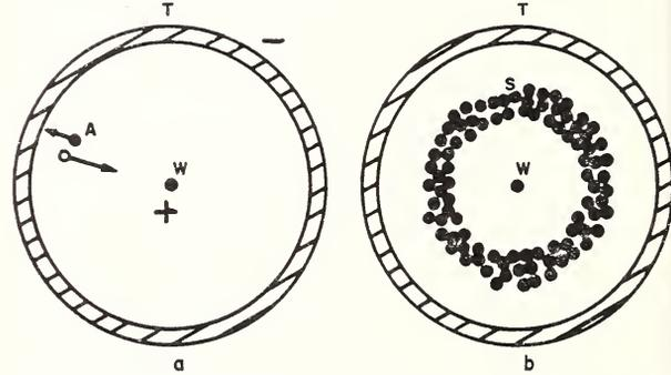
FIGURE 7. Diagram showing steps in formation of an electron avalanche and the positive ion sheath.
