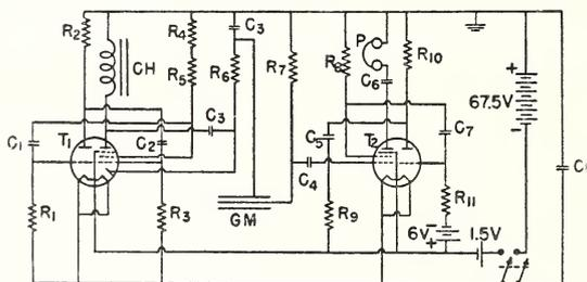
FIGURE 25. Wiring diagram of battery operated portable counting circuit.
