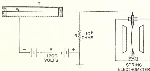
FIGURE 3. Diagram of the counter as developed by Geiger and Müller.
