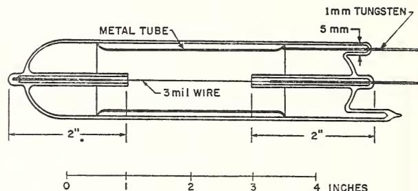
FIGURE 9. Cross section of gamma-ray counter sealed in a glass tube.
