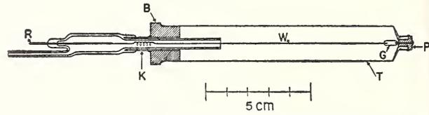
FIGURE 14. Thin-walled counter made from aluminum toothpaste tube.
