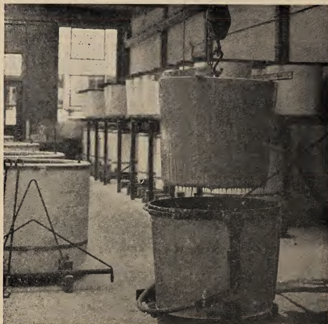
FIGURE 5.—Excess slip draining from the coated core after having remained in the clay slip for 6 minutes.
