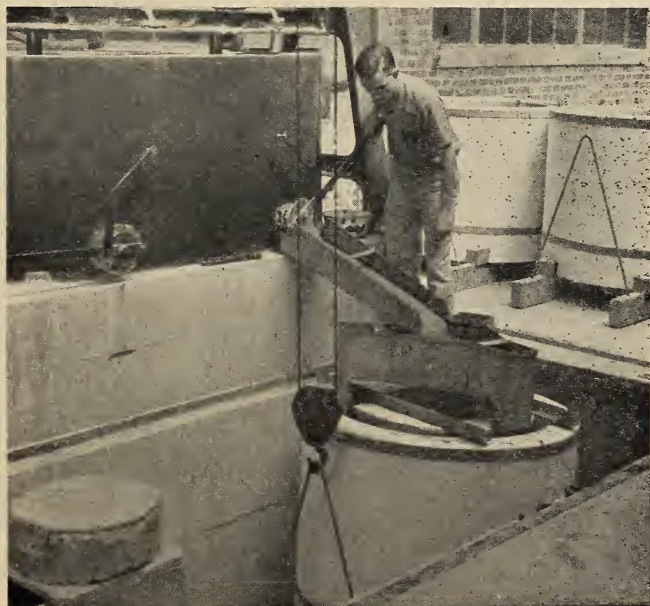
FIGURE 7.— Casting the pot around the lining.
