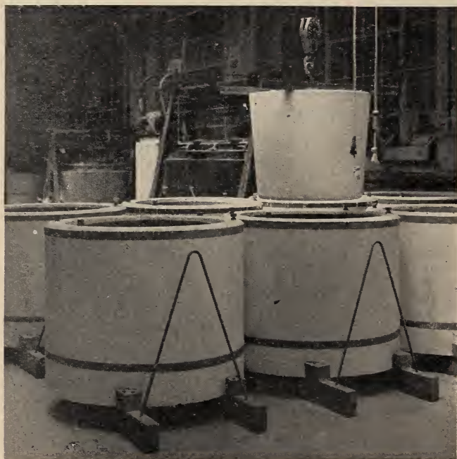
FIGURE 8.—Core removed from pot 8 hours after casting.
