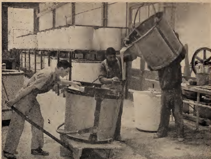
FIGURE 4.—Clay slip being poured into receiver after core had been lowered and locked into position.
