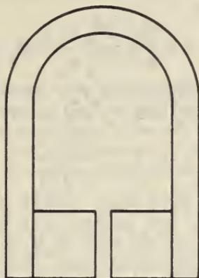
FIGURE 10.—Ordinary U-shaped magnet with pole pieces.
