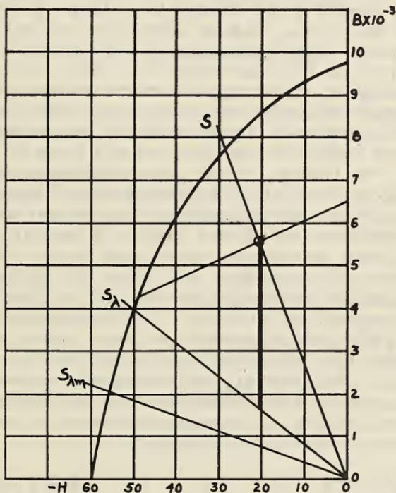
FIGURE 17.—Permanent-magnet diagram for alternative design of instrument magnet.
