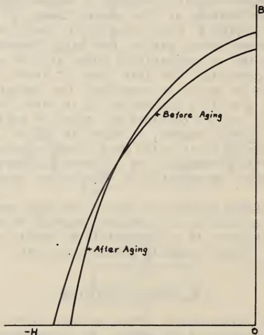
FIGURE 7.—Effect of aging on the demagnetization curve.
