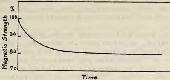
FIGURE 8.—Decay of magnetization with time.
