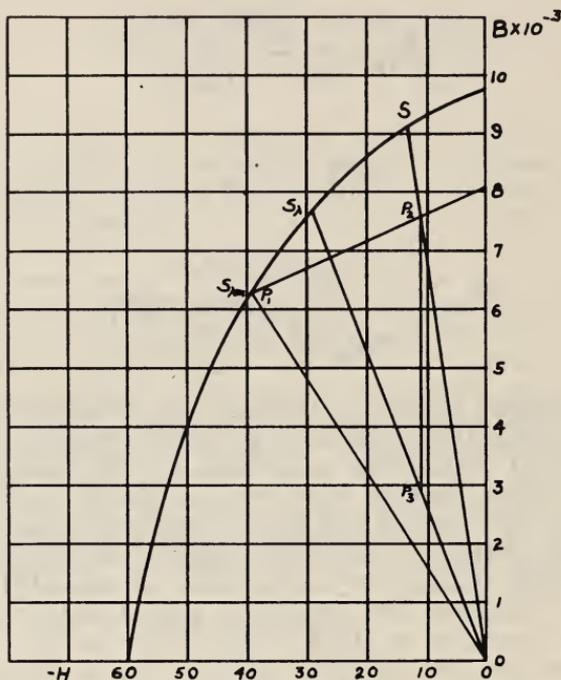
FIGURE 13.—Permanent-magnet diagram for an instrument magnet.
