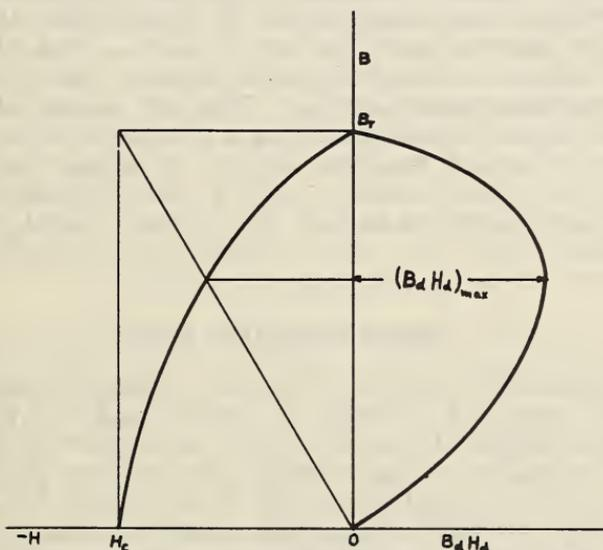
FIGURE 2.—Demagnetization and energy-product curves.
