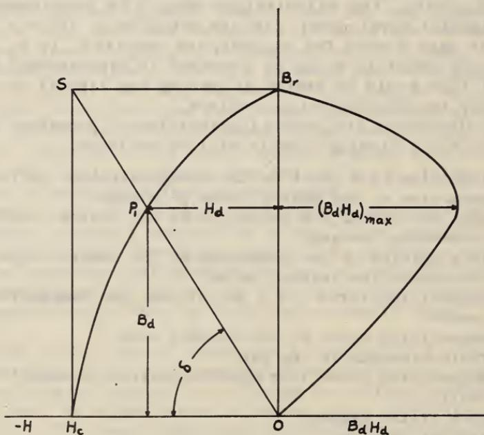
FIGURE 9.—Shearing line and demagnetization curve.
