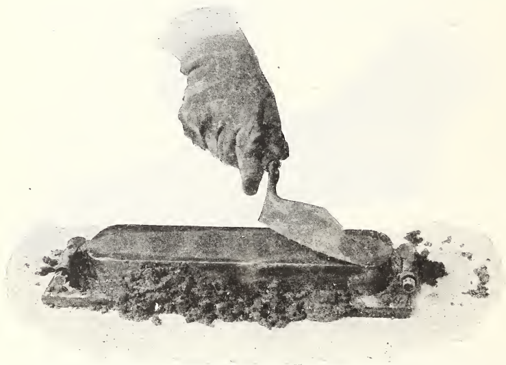
Fig. 8.— Correct Method of Troweling Surface of Briquettes
