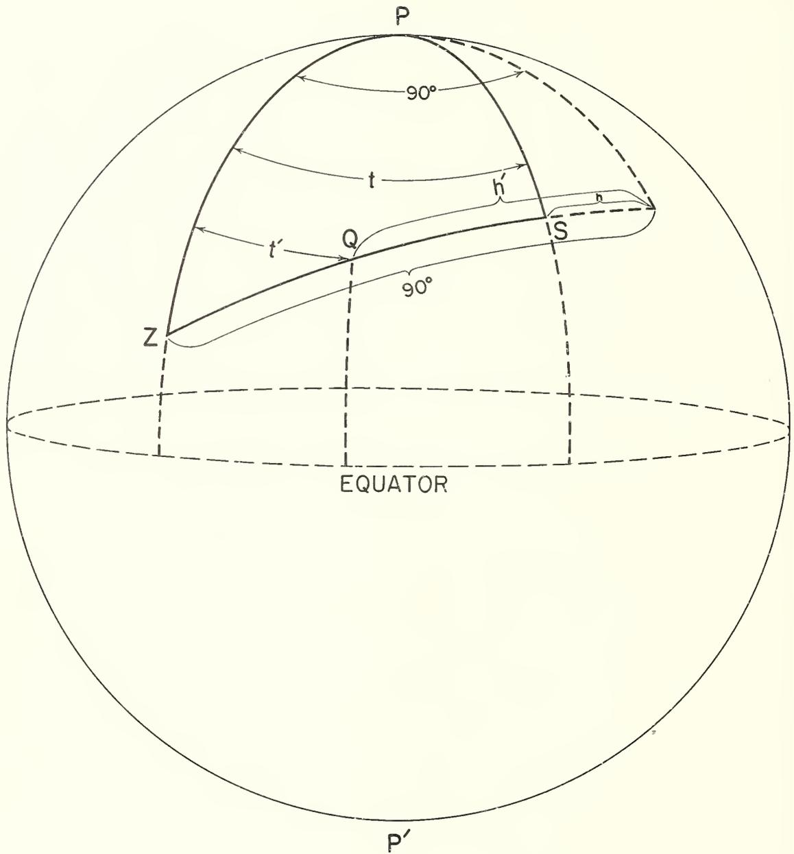
Fig. 14. DIAGRAM OF TRANSMISSION PATH AUXILIARY TO EXPLANATION OF USE OF DISTANCE -- BEARING NOMOGRAM, FIG. 15.
