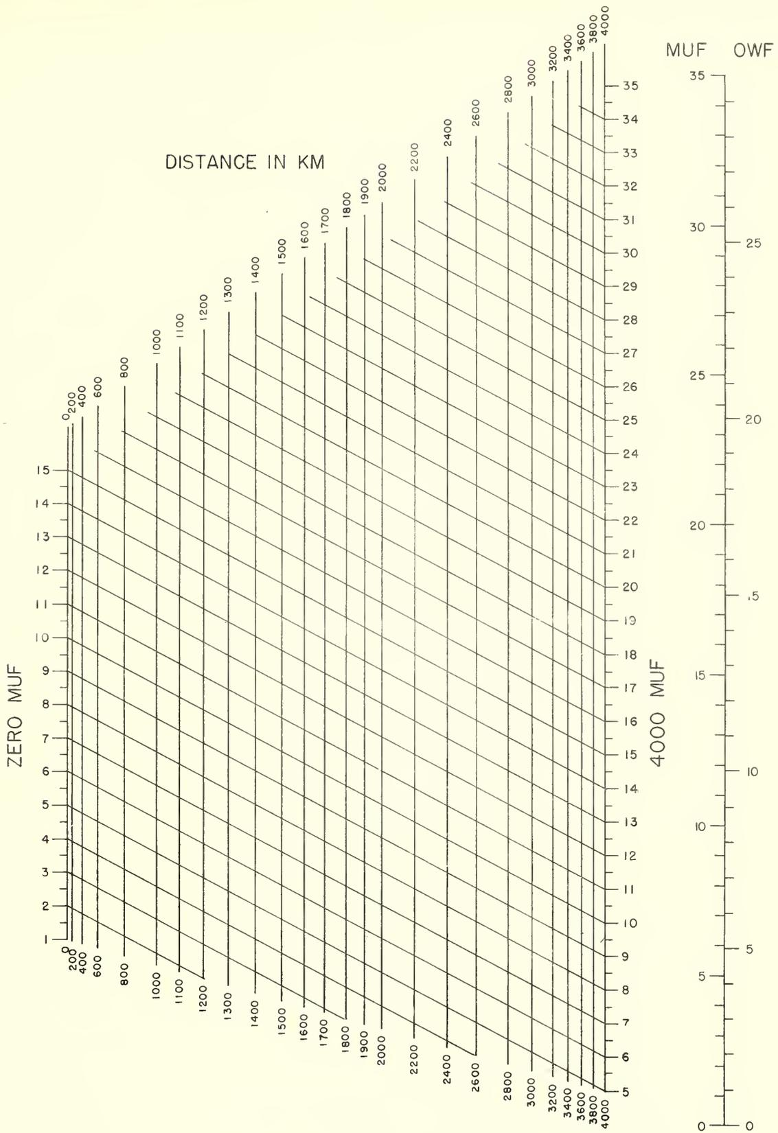
FIG.11 NOMOGRAM FOR TRANSFORMING  $F_2$ -ZERO-MUF AND  $F_2$ -4000-MUF TO EQUIVALENT MAXIMUM USABLE FREQUENCIES AT INTERMEDIATE TRANSMISSION DISTANCES; CONVERSION SCALE FOR OBTAINING OPTIMUM WORKING FREQUENCIES.
