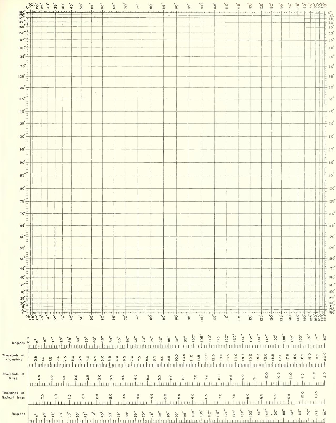
Fig. 15. Nomogram for obtaining great-circle distances, bearings, latitude and longitude of transmission control points, solar zenith angles.
