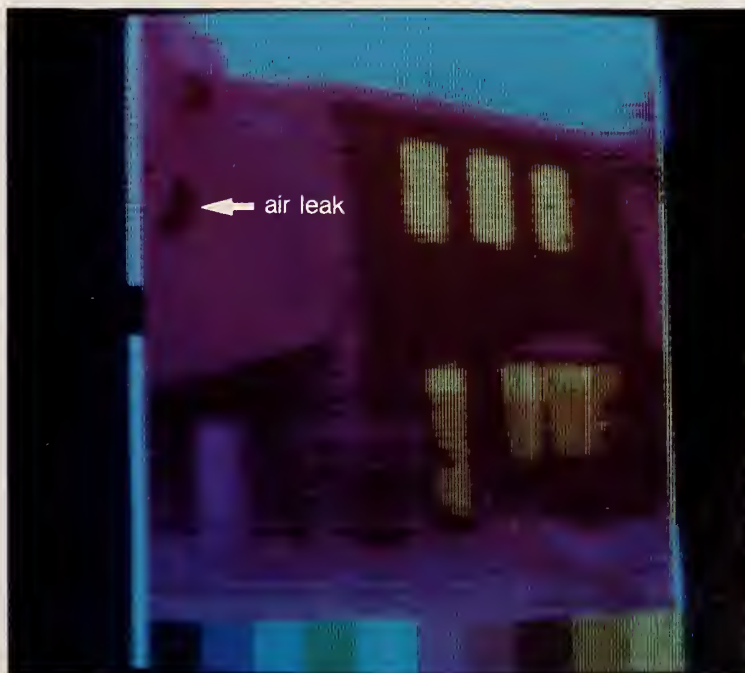
Figure 3b. Exterior thermographic scan while pressurized.
