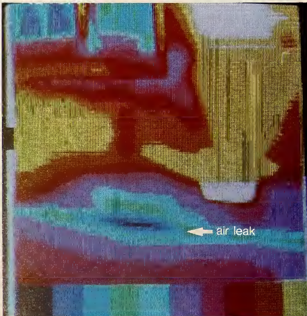
Figure 4b. Wall/floor interface while pressurized.
