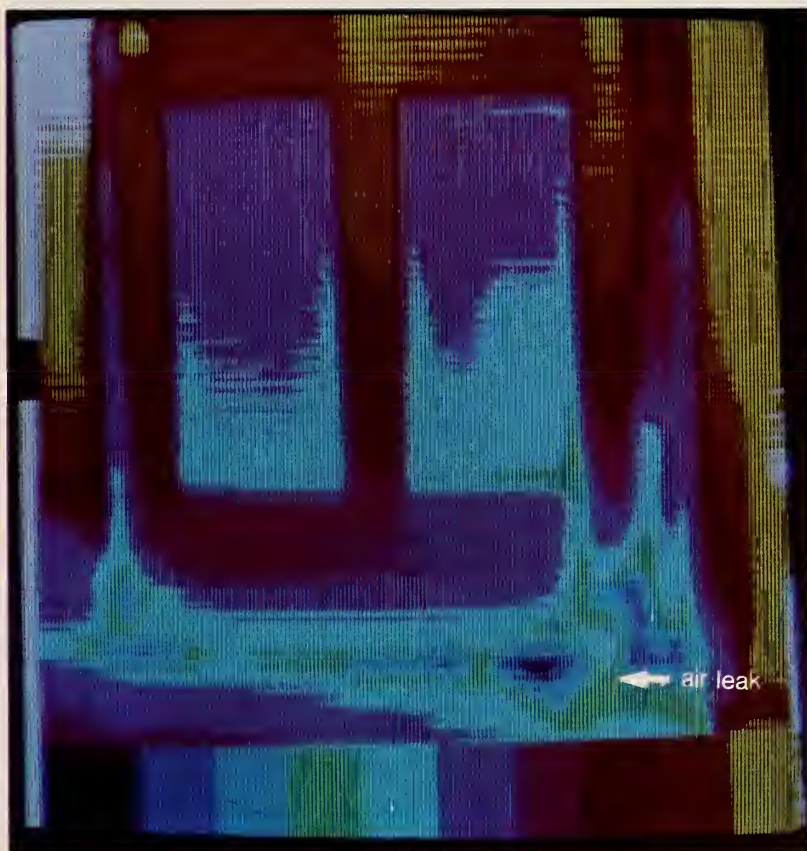
Figure 5. Front door while pressurized.
