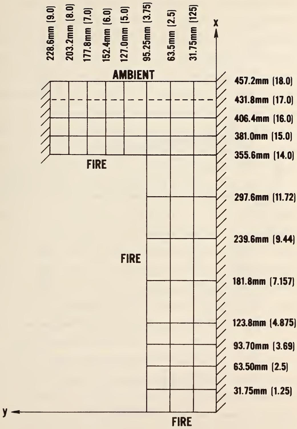
Fig. 11 Cross-Section Descretization for Beam-Slab Section
