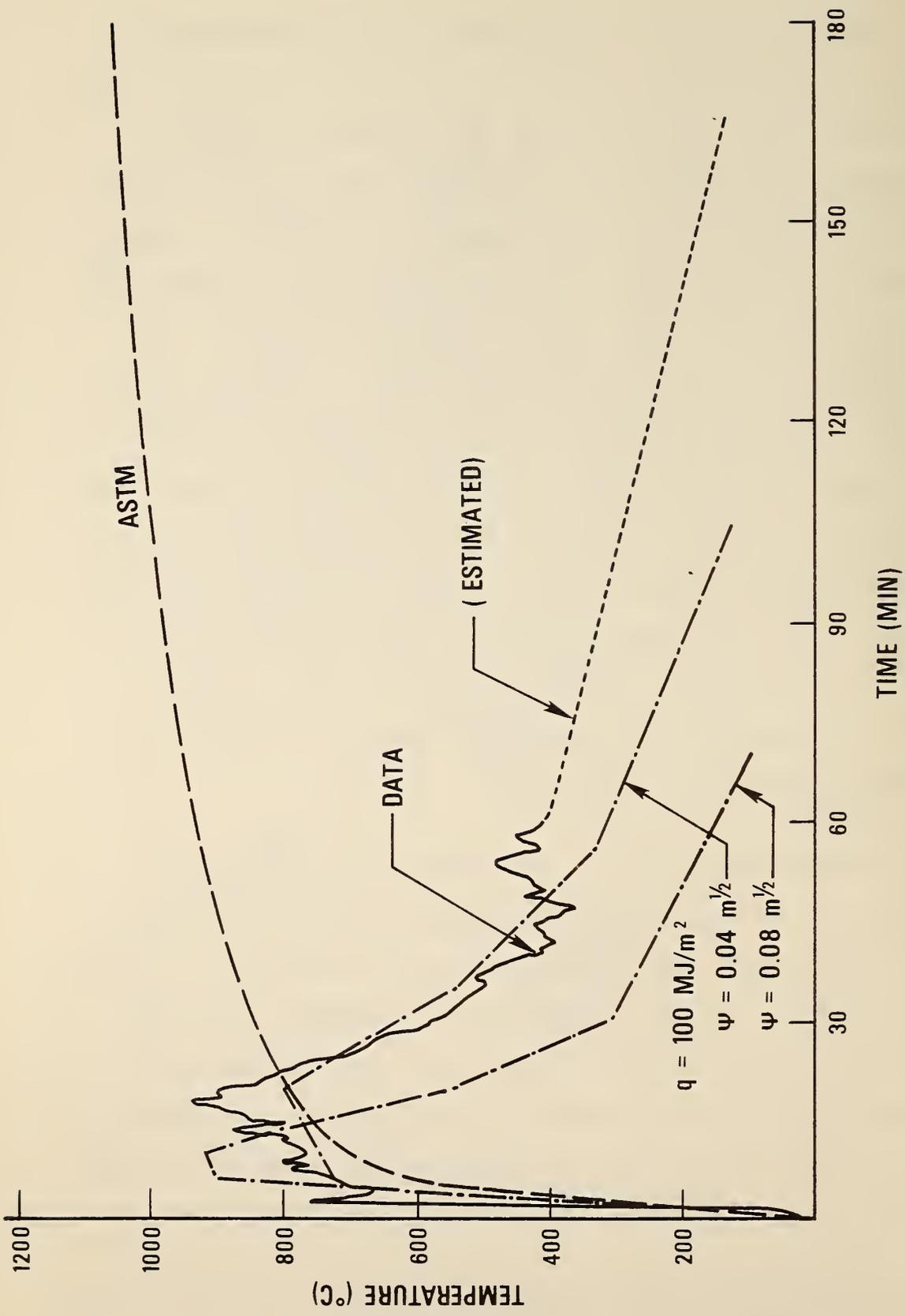
Fig. 2 Comparison of ASTM Fire Curve with Measured Fire Temperatures
