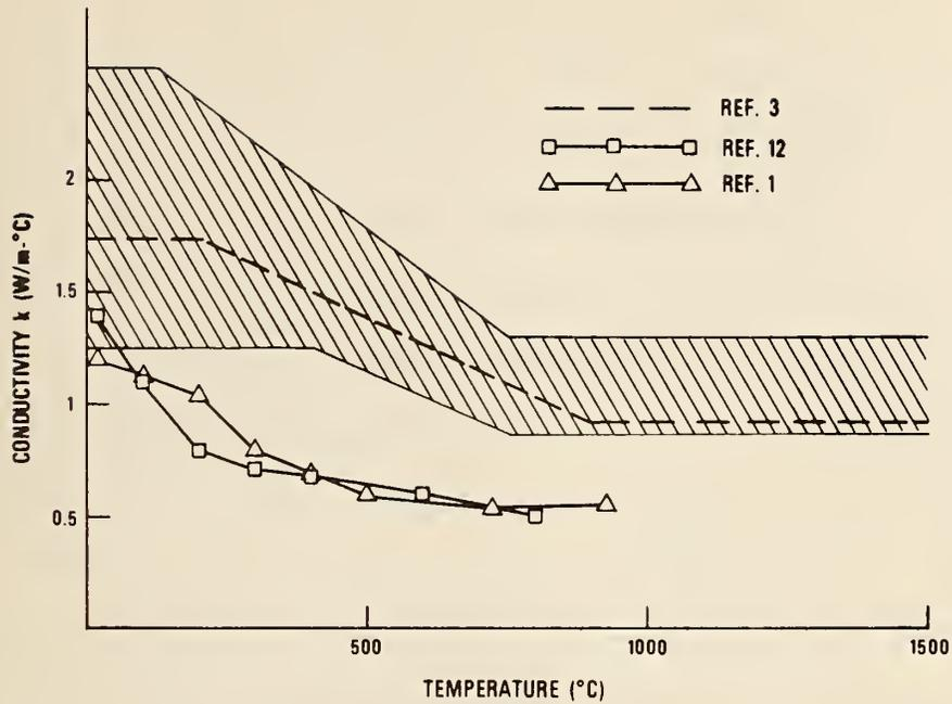
Fig. 4 Effect of Temperature on Conductivity of Concrete
