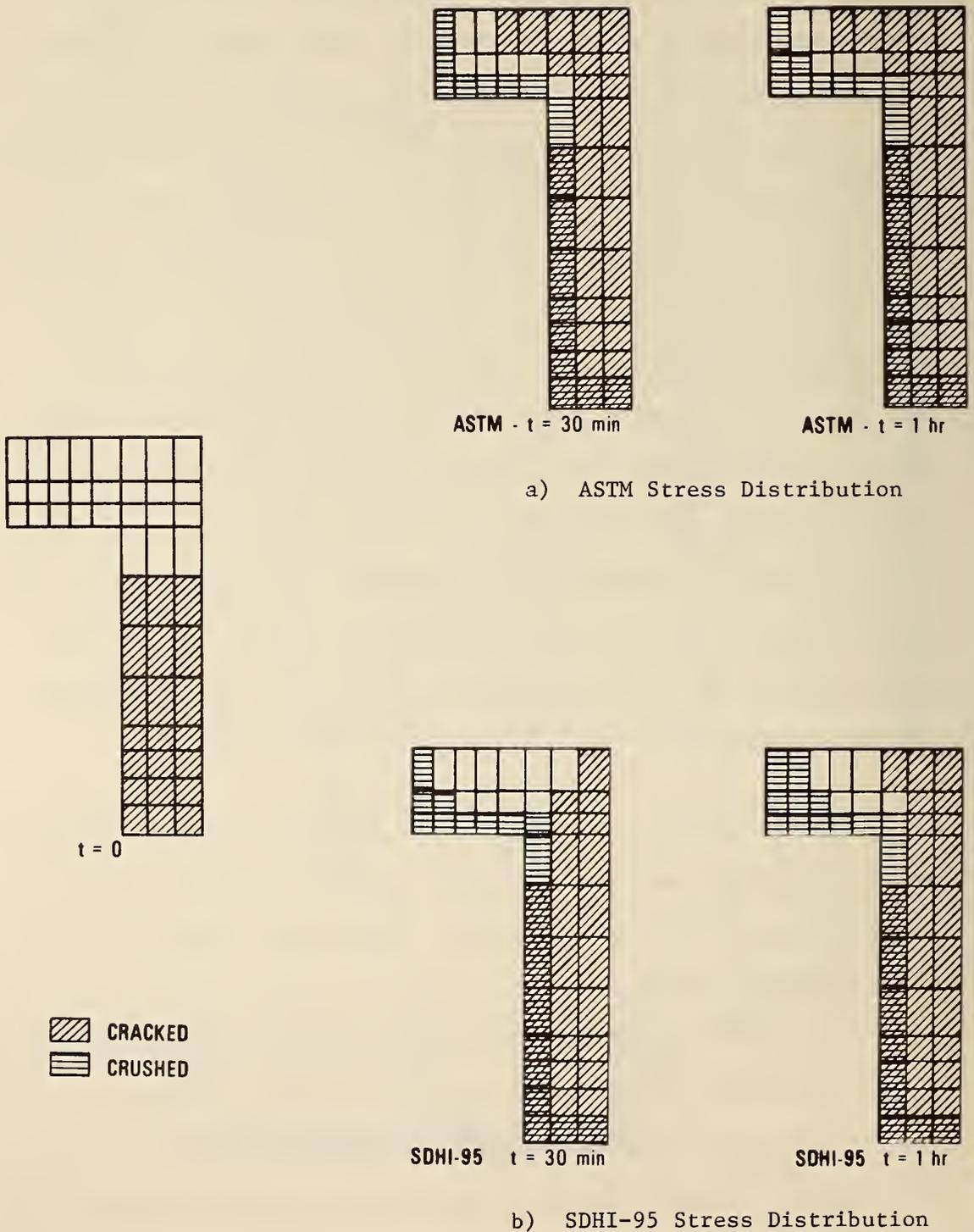
Fig. 16 Effect of Stress Distribution on Beam-Slab Section for ASTM and SDHI-95 Fire Curves
