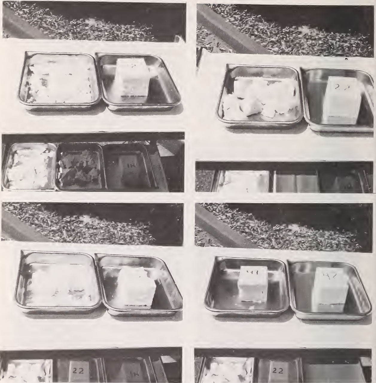
Figure 2. Foam Specimens after Exposure to 122°F (50°C) and 92% rh for 7 Weeks Control Specimens 12, 22, 32 and 42 were not Exposed to High Temperature and Humidity.
