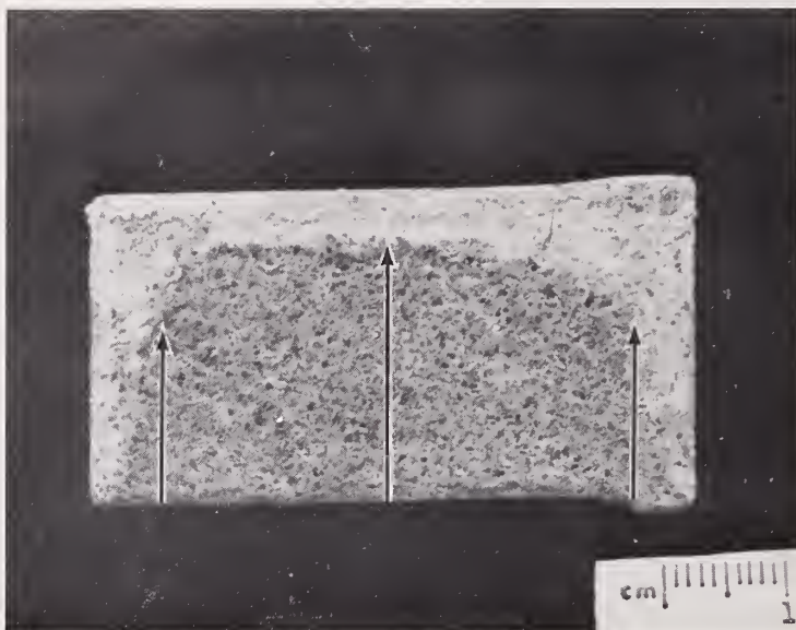
Figure 24. Water Condensation/Evaporation (4.3): degradation and transport of stone preservative treatment by water condensation/evaporation testing (2400 cycles). Side view of specimen. Arrows indicate direction of water migration from bottom, coated surface of specimen to the top, uncoated surface.
