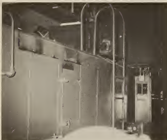
Figure 15. Typical oven used to elevate the temperature of products by indirect heating. Note the single burner in the heat exchanger on top of the oven.
