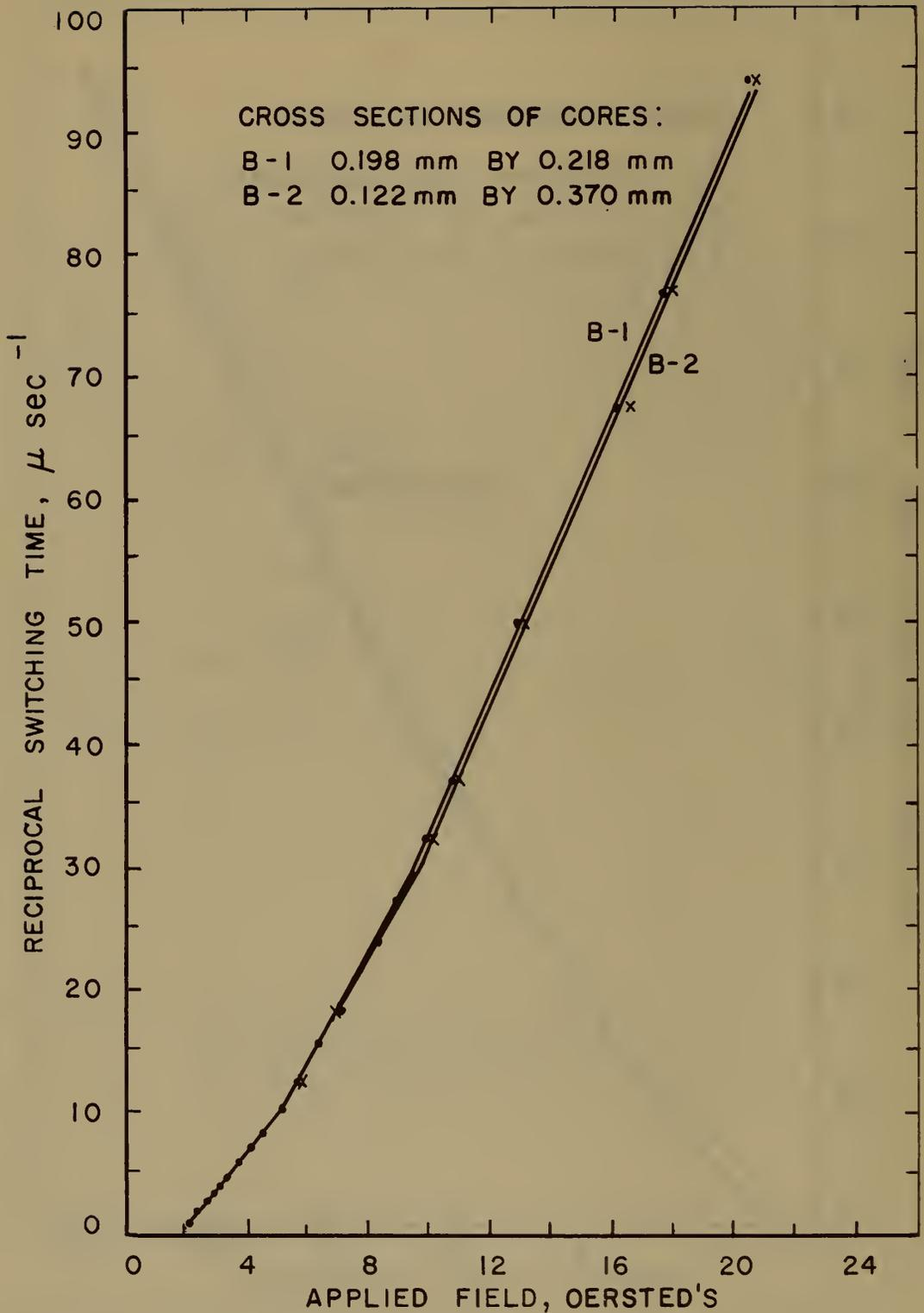
Figure 11. Reciprocal Switching Time Versus Applied Field for 2 Type F<sub>5</sub> Cores of Different Cross Section
