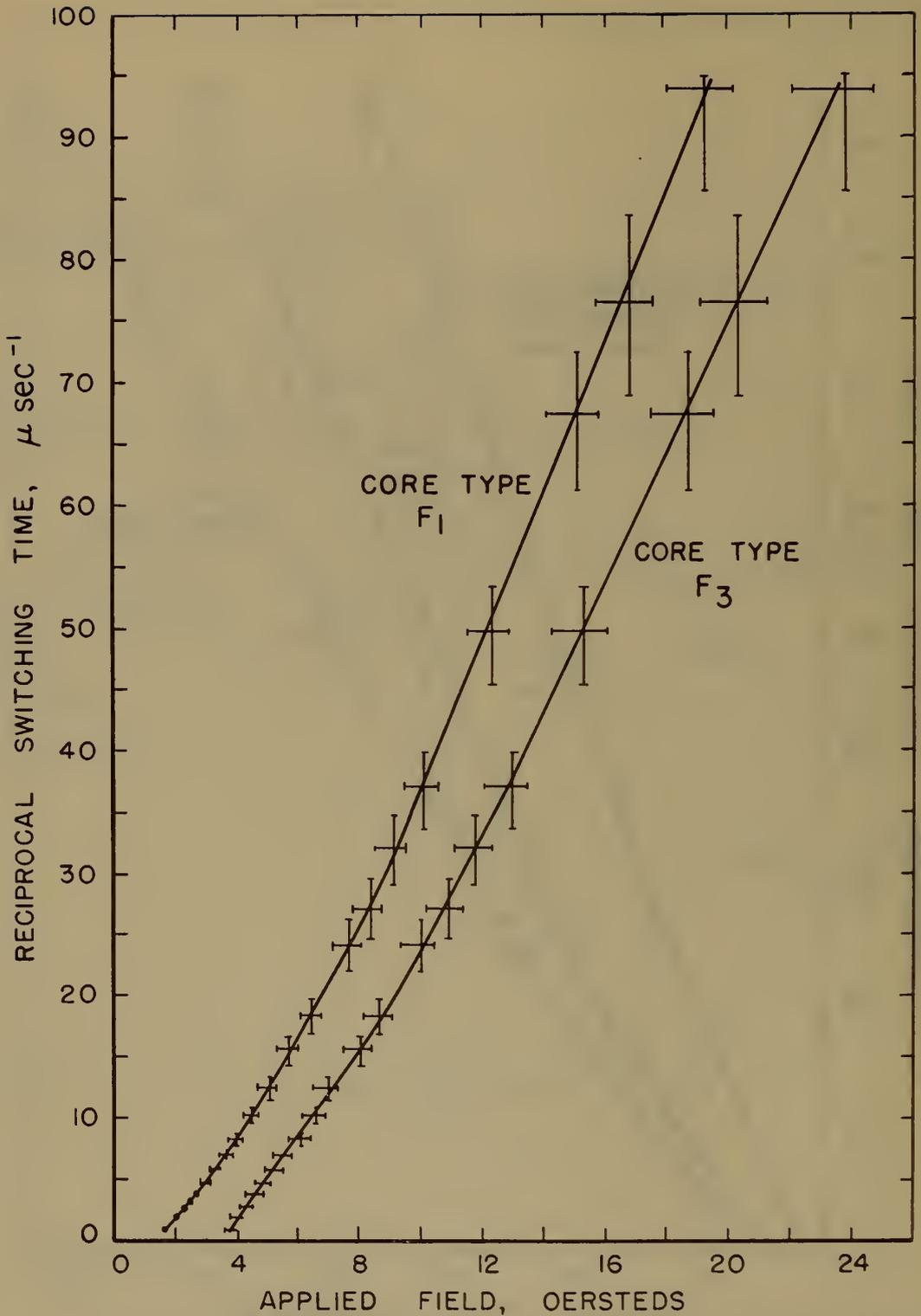
Figure 7. Reciprocal Switching Time Versus Applied Field for Core Types F<sub>1</sub> and F<sub>3</sub>
