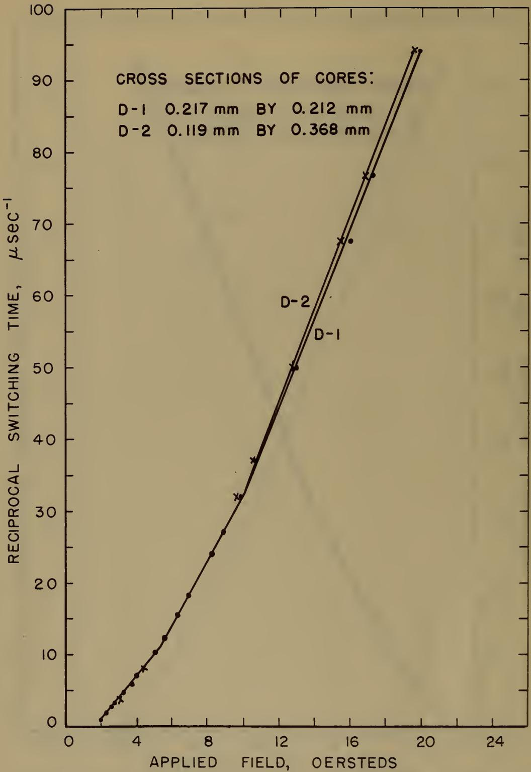
Figure 13. Reciprocal Switching Time Versus Applied Field for 2 Type F<sub>5</sub> Cores of Different Cross Section
