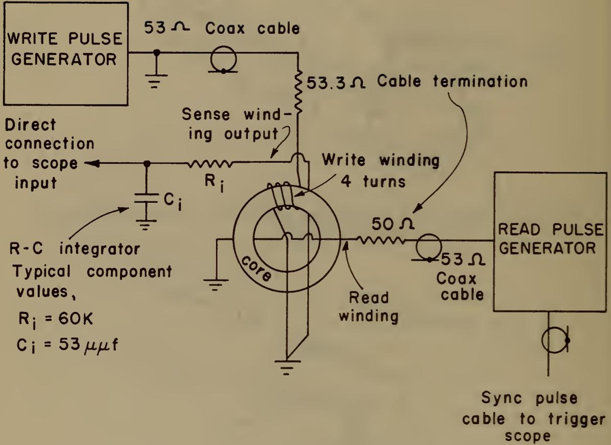
Figure 5. Experimental Layout for Obtaining Switching Curve Data
