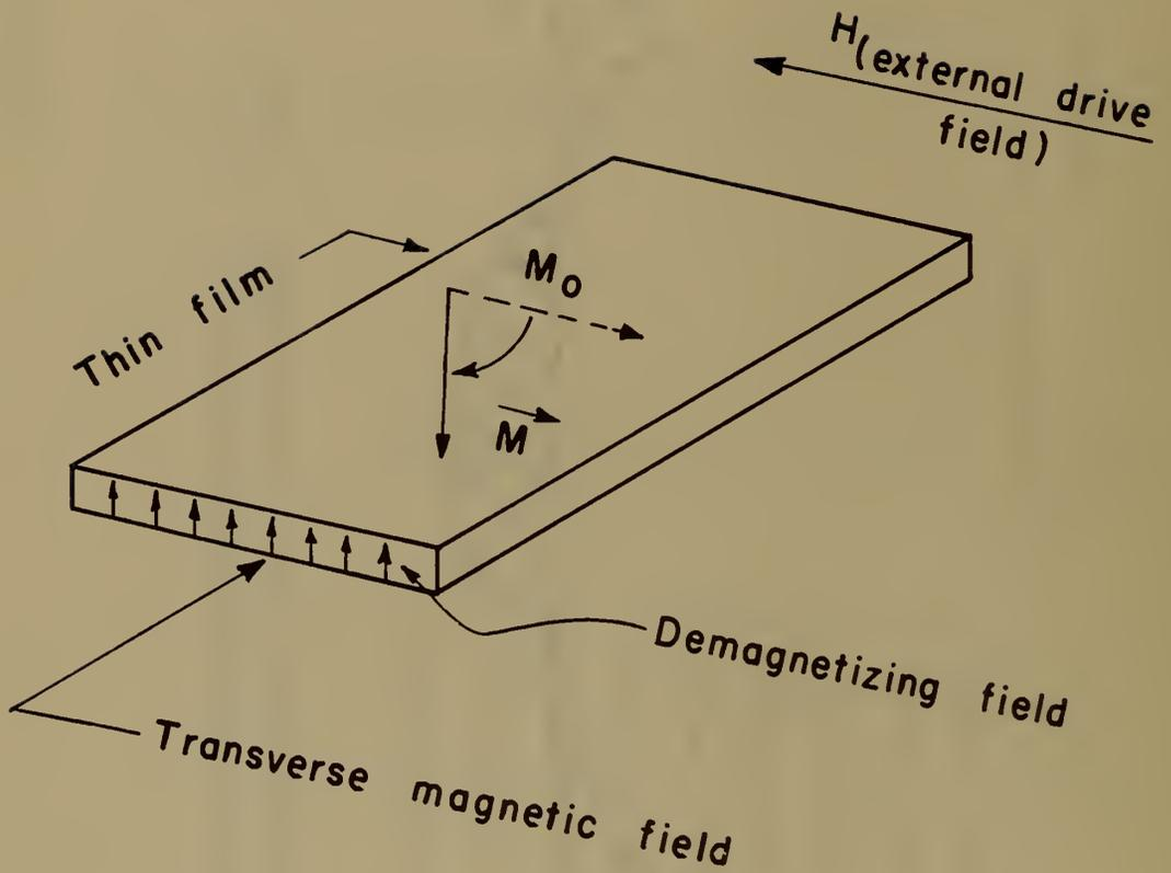
Figure 2. Flux Reversal in Thin Films by Coherent Rotation
