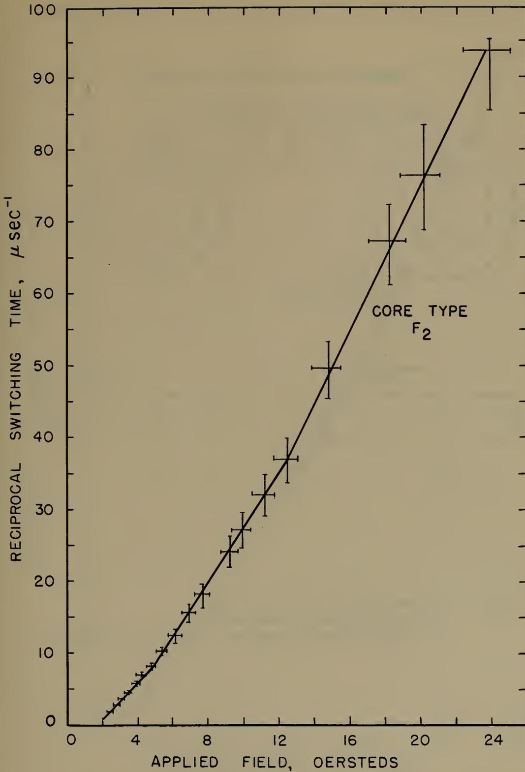
Figure 8. Reciprocal Switching Time Versus Applied Field for Ferrite Core Type F<sub>2</sub>.
