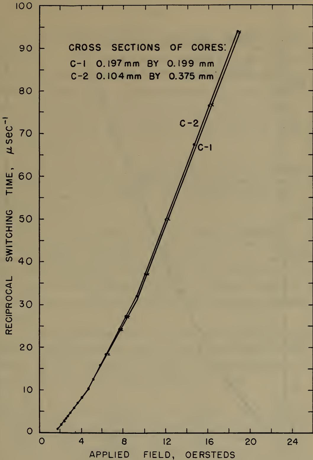
Figure 12. Reciprocal Switching Time Versus Applied Field for 2 Type F<sub>1</sub> Cores of Different Cross Section
