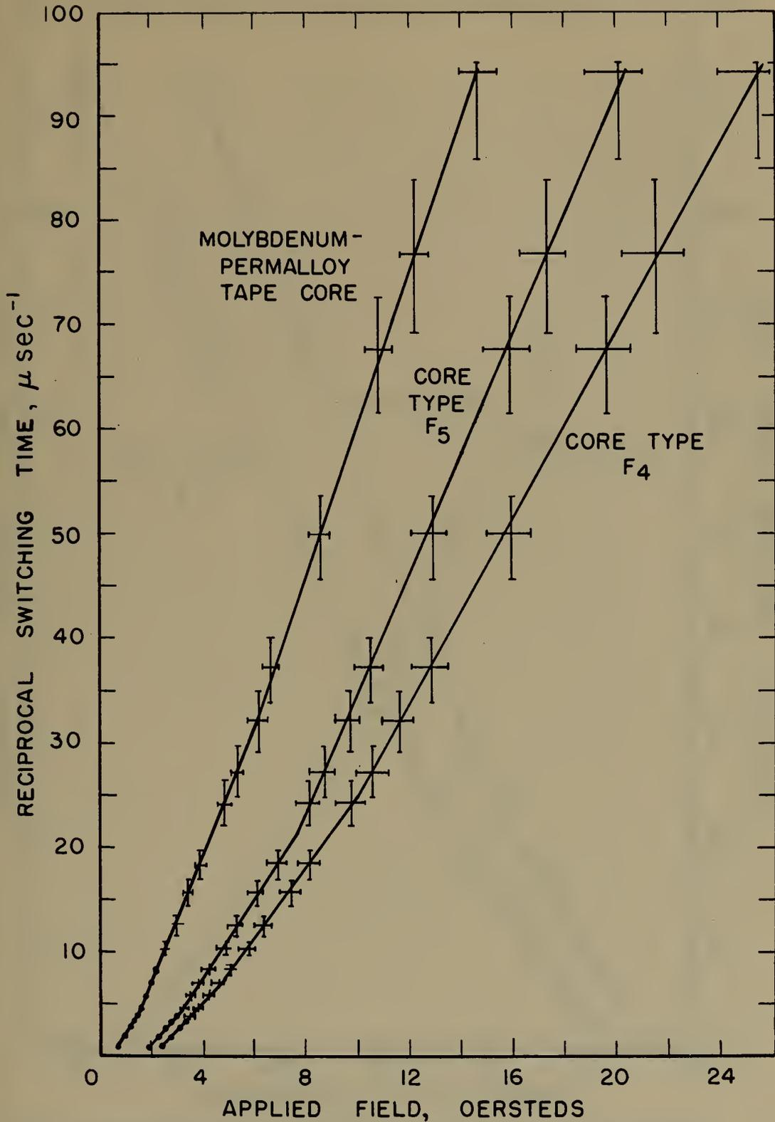
Figure 6. Reciprocal Switching Time Versus Applied Field for a Ferromagnetic Tape Toroid and Ferrite Core Types F<sub>4</sub> and F<sub>5</sub>
