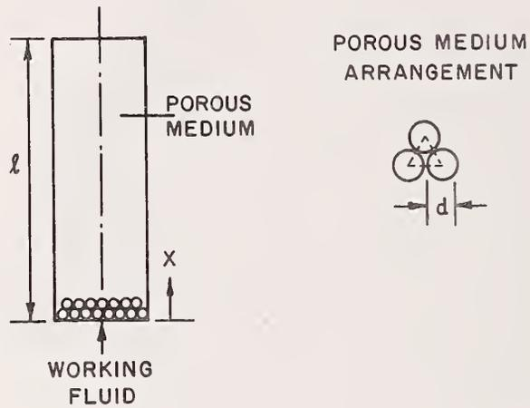
Figure B8 Schematic Representation of a Pebble Bed-Type Thermal Storage Unit from Reference [14]
