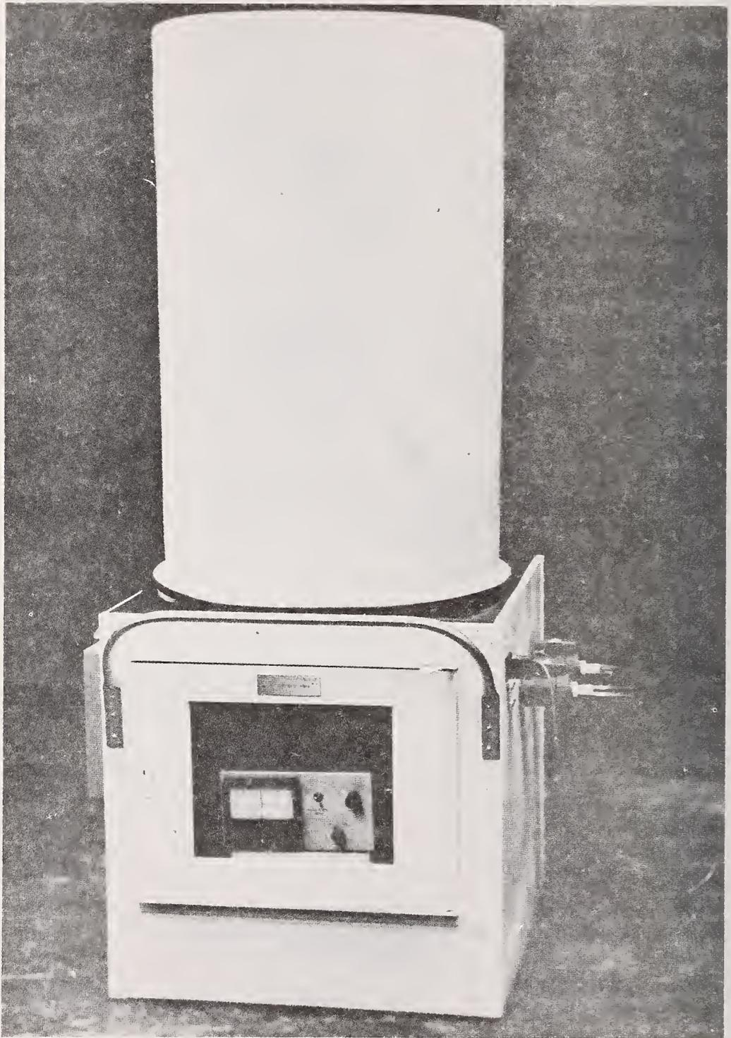
Figure 27 Arthur D. Little Calorimeter used for Determining the Thermal Efficiency of Solar Collectors [67]
