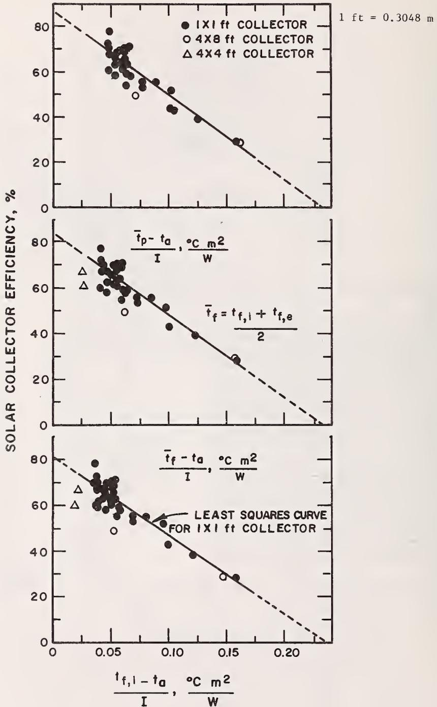
Figure 23 Efficiency Curve for a Double-Glazed Liquid-Heating Solar Collector of Three Different Sizes [56]
