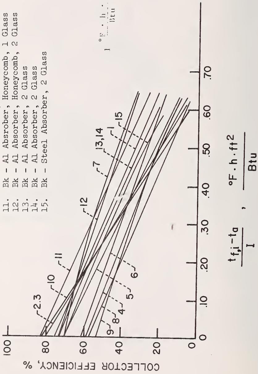
Figure 31 Efficiency Curve for Fifteen Liquid-Heating Solar Collectors Determined using the Indoor Test Facility at the NASA Lewis Research Center [29]
