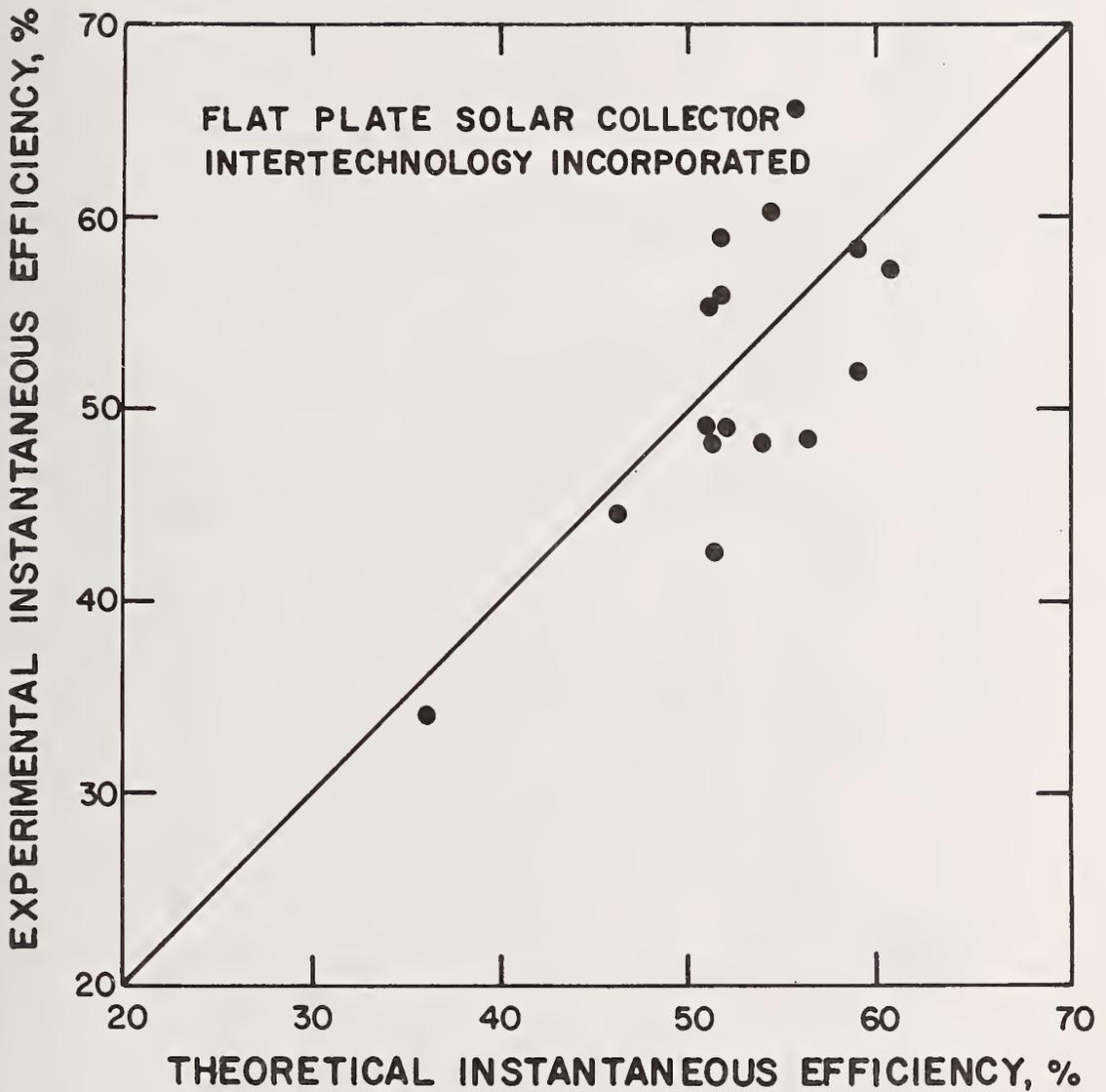
Figure 20 Measured Versus Predicted Thermal Efficiency for a Large Solar Collector Array Installed as part of a Solar Heating Experiment in Warrenton, Virginia [53]
