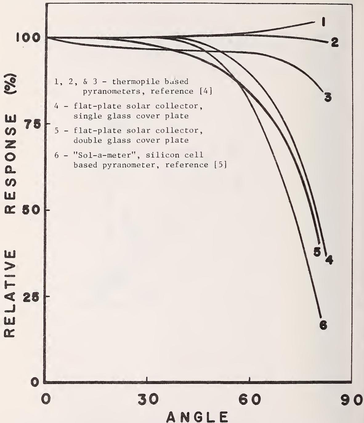
Figure C2. The Relative Directional Response of Commercially Available Pyranometers.
