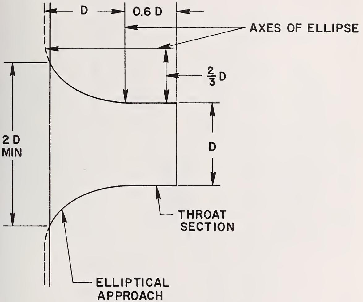
Figure A6 Air Flow Measuring Nozzle
