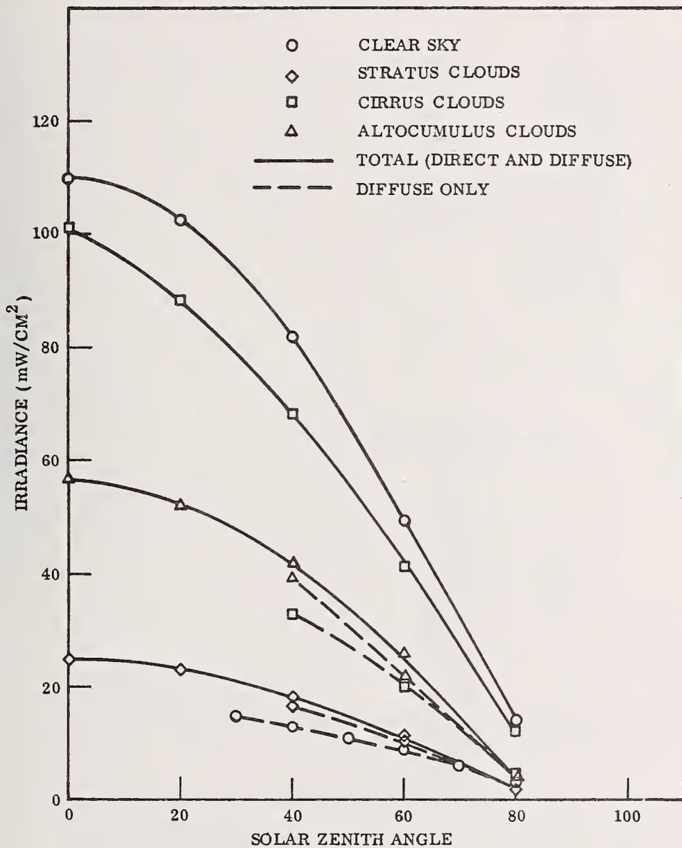
Figure 58 Ground Solar Irradiance for Various Cloud Conditions [97]
