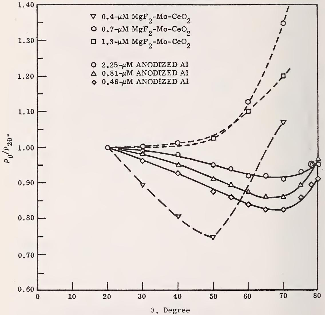
Figure 63 Normalized Directional Reflectance of Two Types of Solar Absorber Coatings [98]
