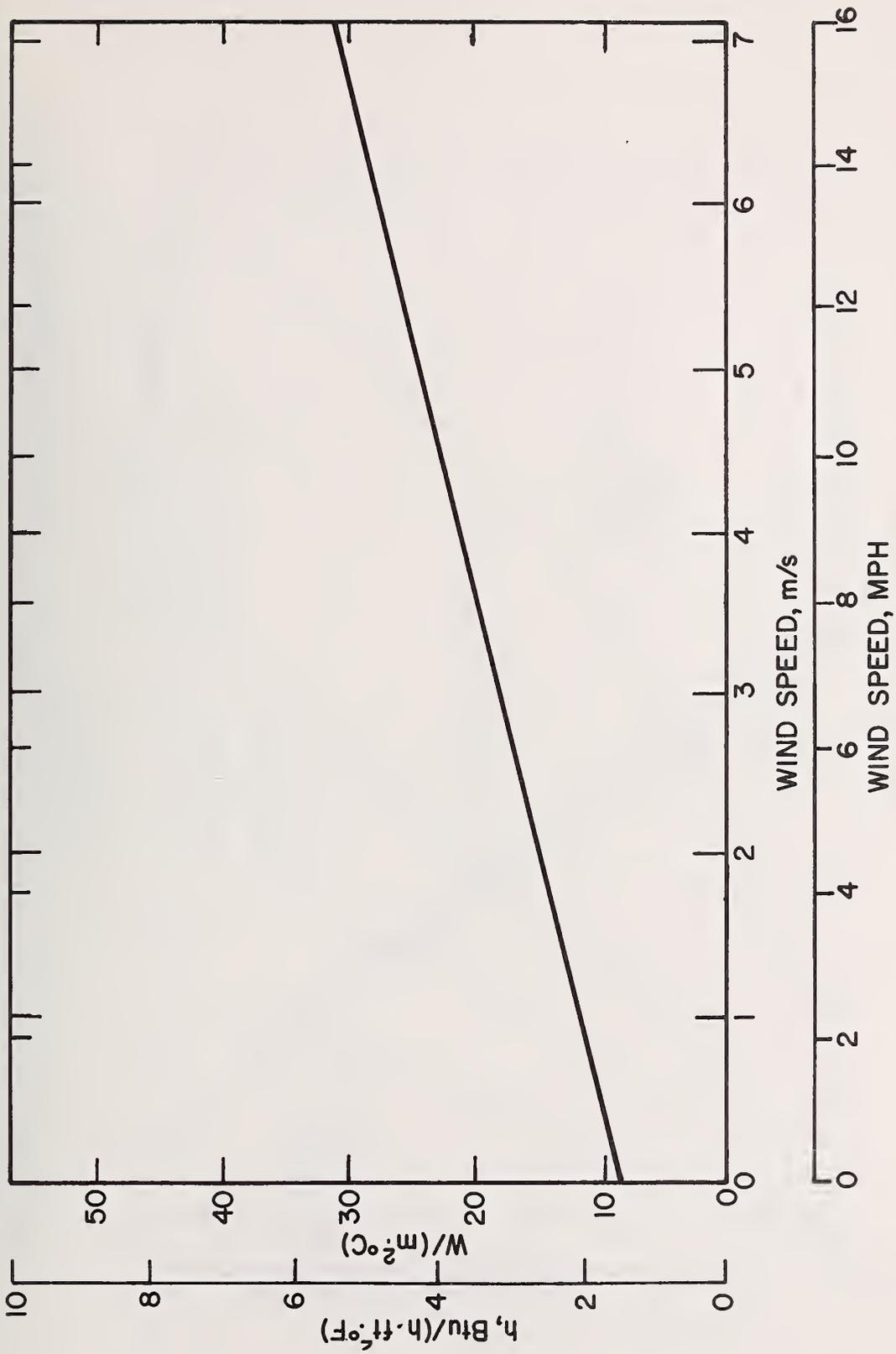
Figure 46 The Outside Surface Heat Transfer Coefficient of a Solar Collector Versus the Wind Speed
