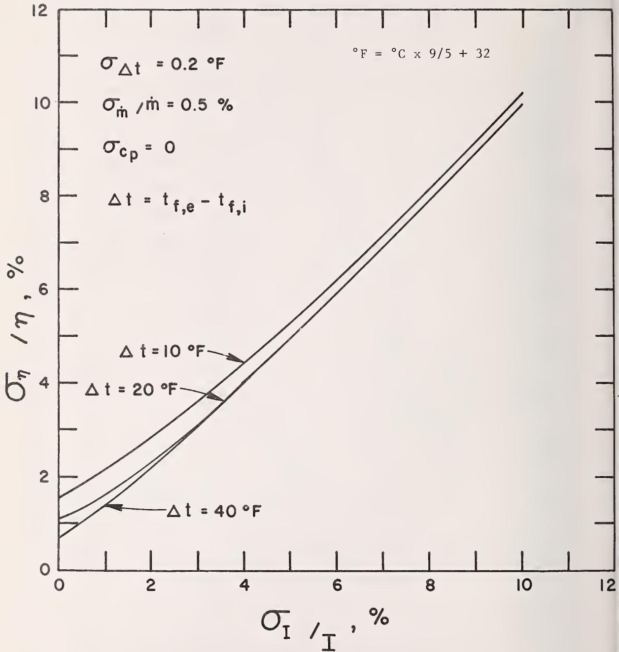
Figure 45 Uncertainty in Solar Collector Thermal Efficiency as a Function of the Uncertainty in Insolation .
