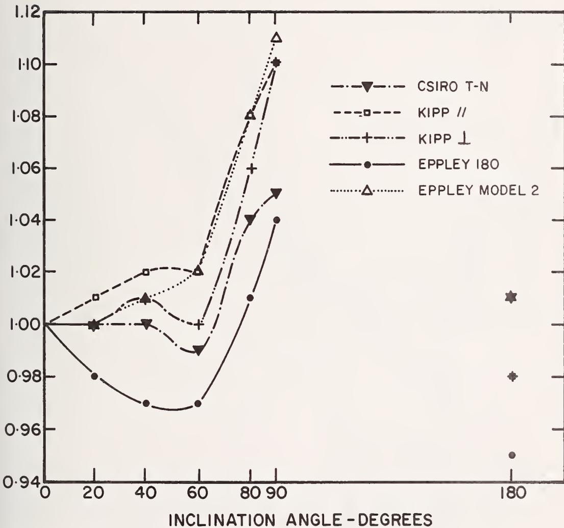
Figure 44 Variation in Response with Attitude for Selected Pyranometers as Determined by Norris [93]
