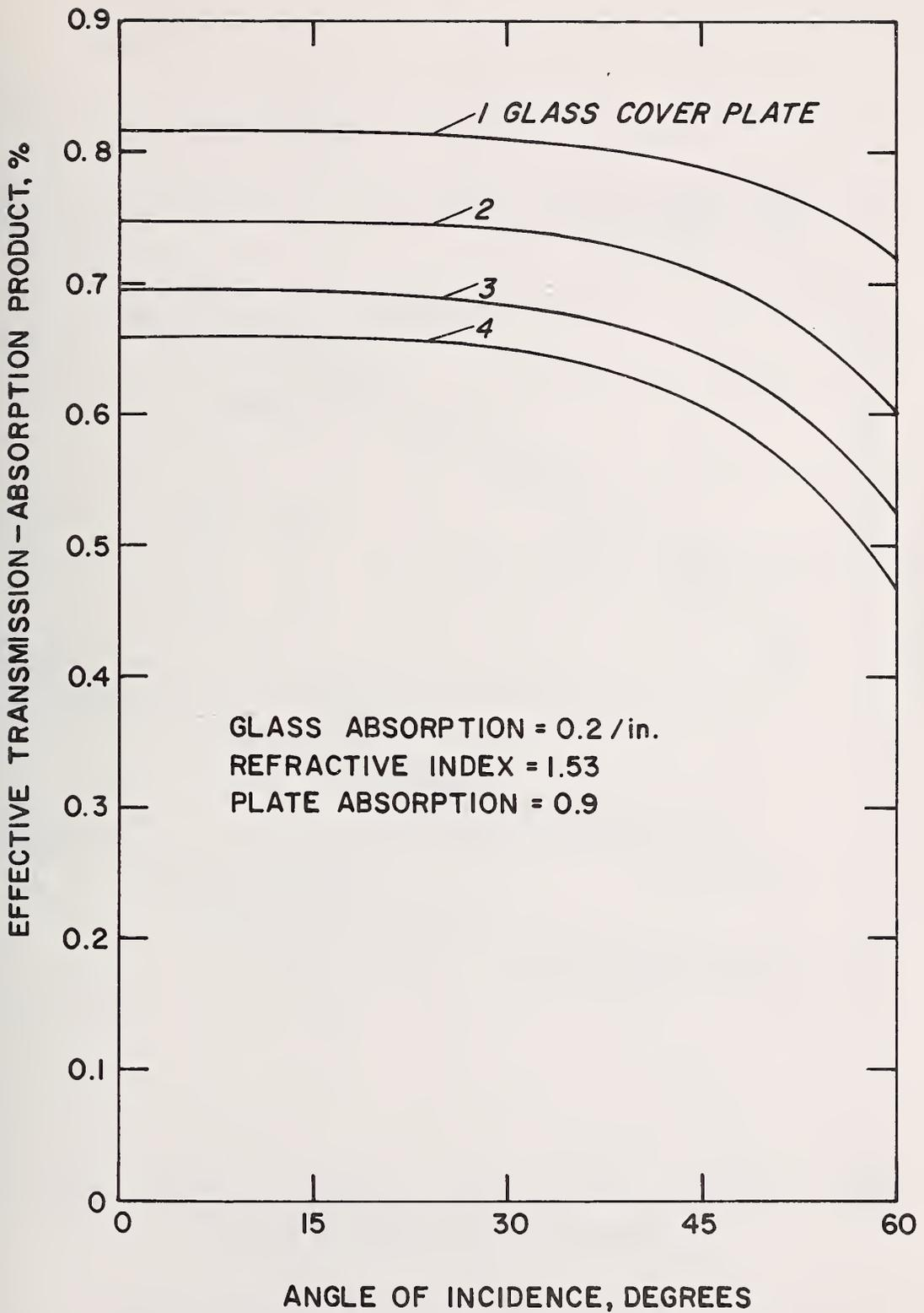
Figure 4 Transmittance-Absorptance Product for Multiple-Cover, Flat-Black Coating Combinations on a Flat-Plate Solar Collector [17]
