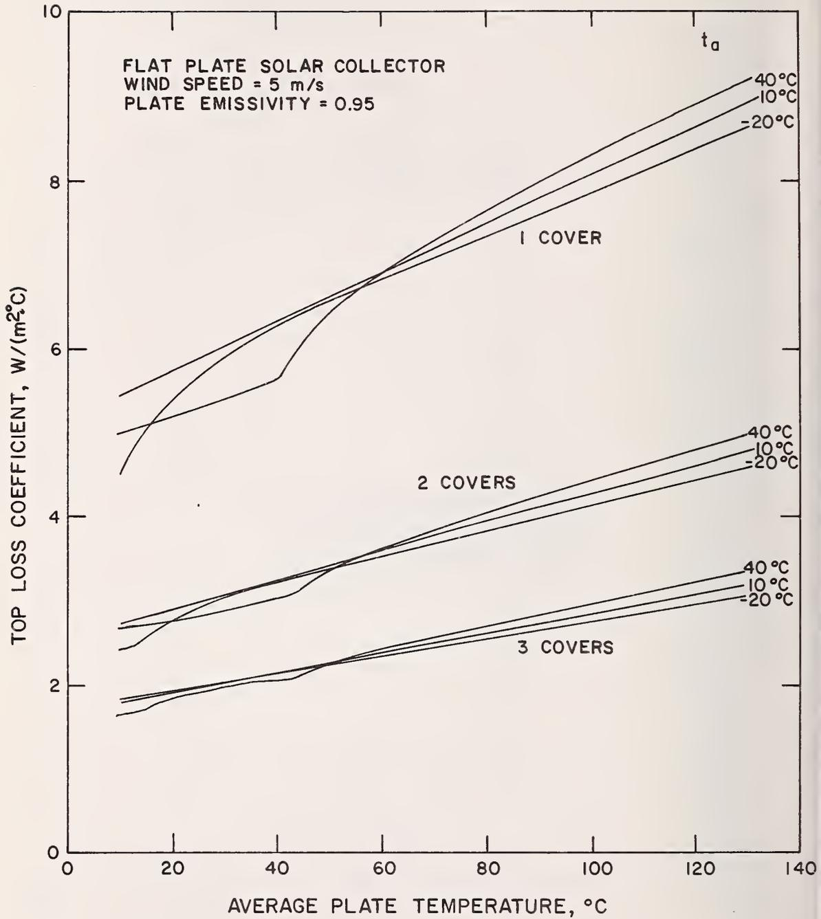
Figure 5. Top Loss Coefficient for Multiple-Cover Flat-Plate Solar Collectors as a Function of Ambient and Plate Temperature [18]
