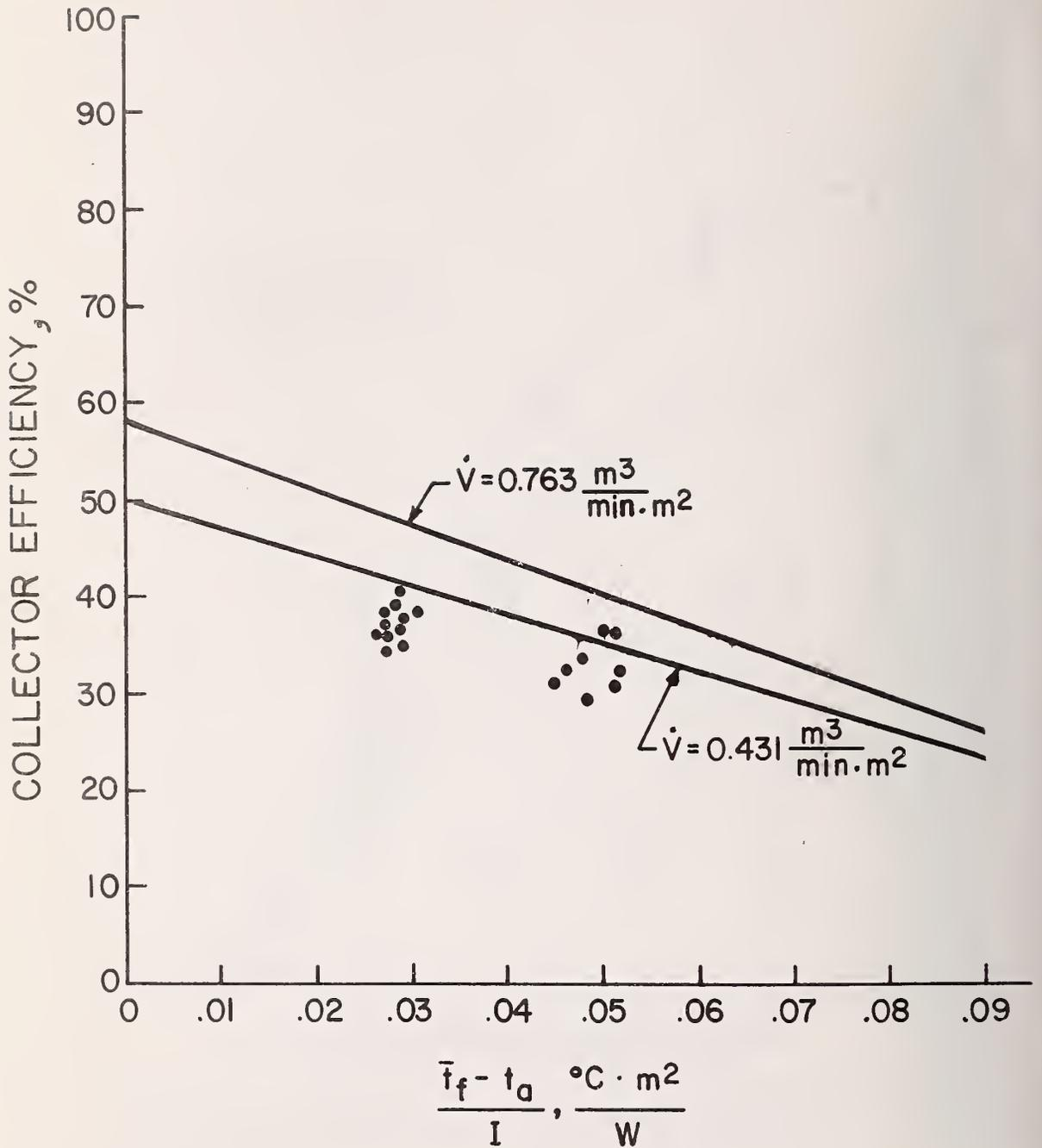
Figure 39 Comparison of Predicted and Measured Air Collector Efficiencies [90]
