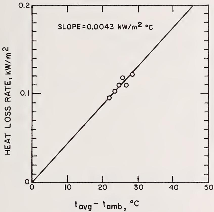
Figure 16 Heat Loss Rate as a Function of Temperature Difference for a Double-Glazed Liquid-Heating Flat-Plate Solar Collector [51]
