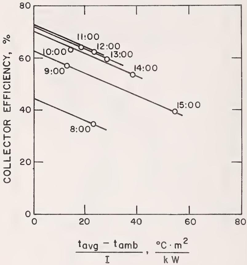
Figure 17 Efficiency Curve for a Double-Glazed Liquid-Heating Flat-Plate Solar Collector [51]
