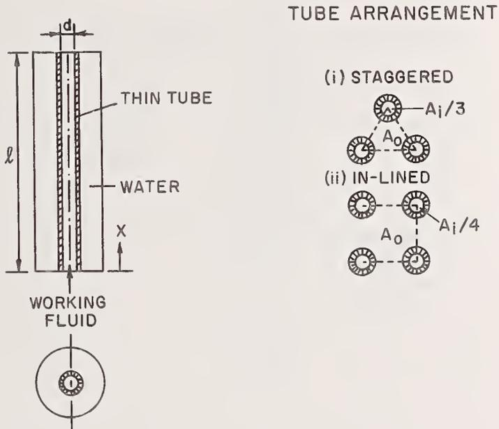
Figure B7 Schematic Representation of a Heat Exchanger-Type Thermal Storage Unit from Reference [14]
