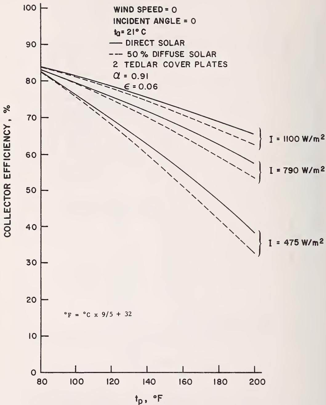
Figure 61 Comparison of Calculated Solar Collector Efficiency for Direct and 50% Diffuse Solar Radiation and with the Sun Normal to the Collector
