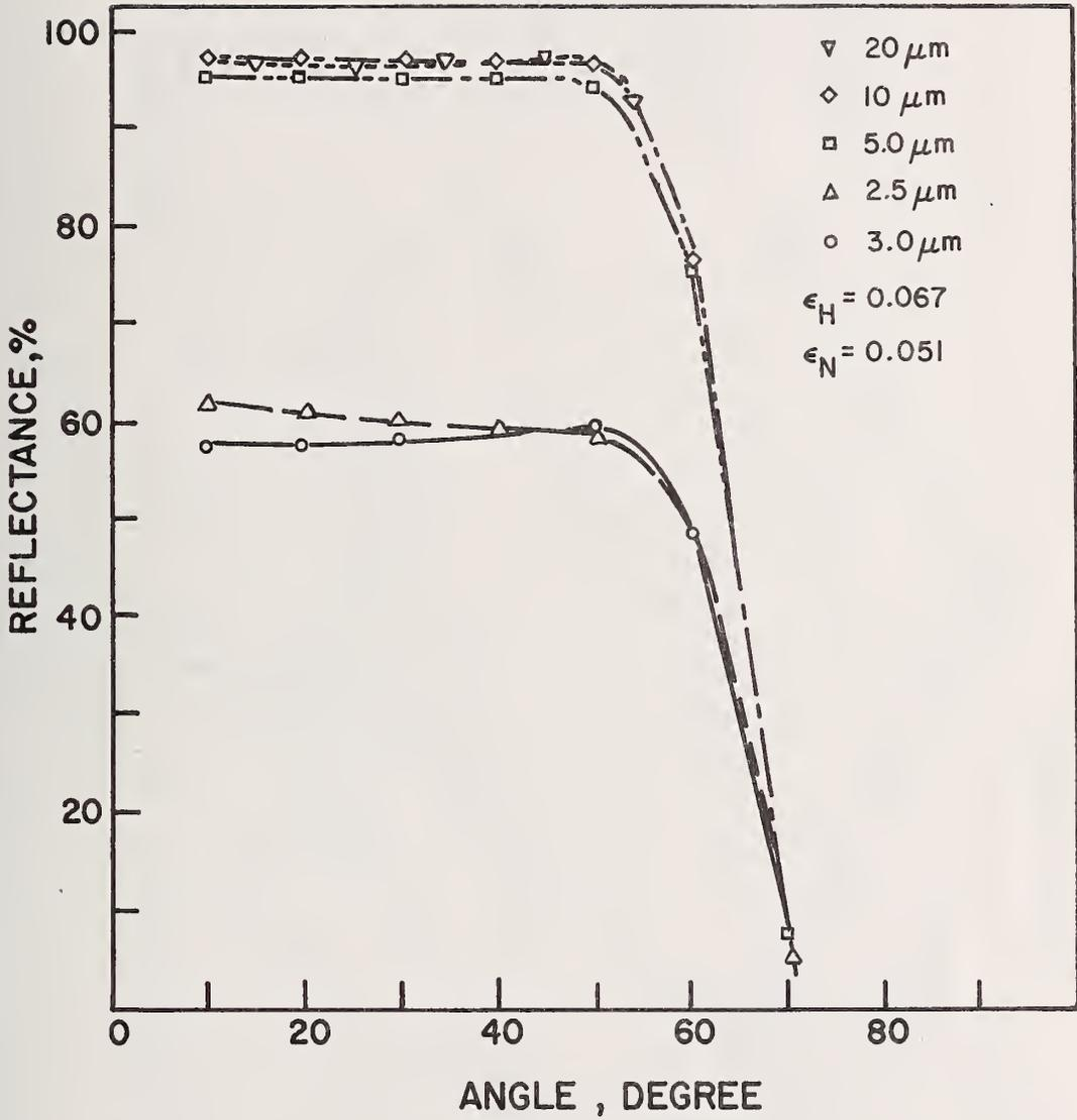
Figure 64 Infrared Reflectance of Cobalt Oxide Versus Incident Angle [98]
