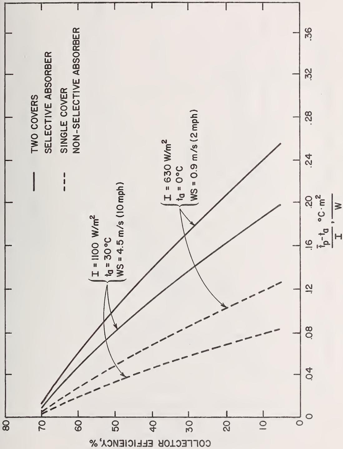
Figure 56 The Effect of Simultaneous Variations in Insolation, Ambient Temperature, and Wind Speed on the Efficiency Curve for Single- and Double-Glazed Flat-Plate Solar Collectors
