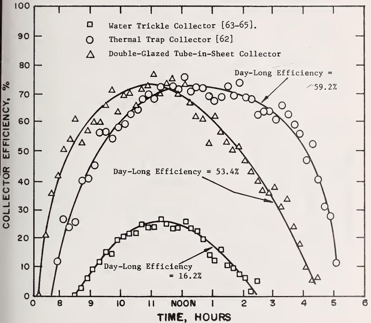
Figure 24 Thermal Efficiency of three different Liquid-Heating Solar Collectors as a Function of Time of Day [61]
