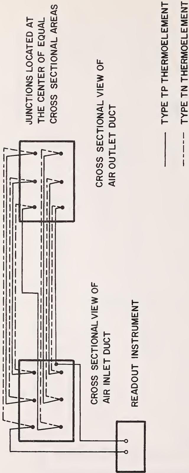
Figure B2 Schematic of the Thermopile Arrangement Used to Measure the Temperature Difference Across the Thermal Storage System
