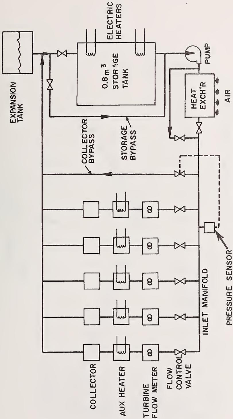
Figure 32 Schematic of the Liquid Flow loop used in the Outdoor Solar Collector Test Facility at the NASA Lewis Research Center [73]
