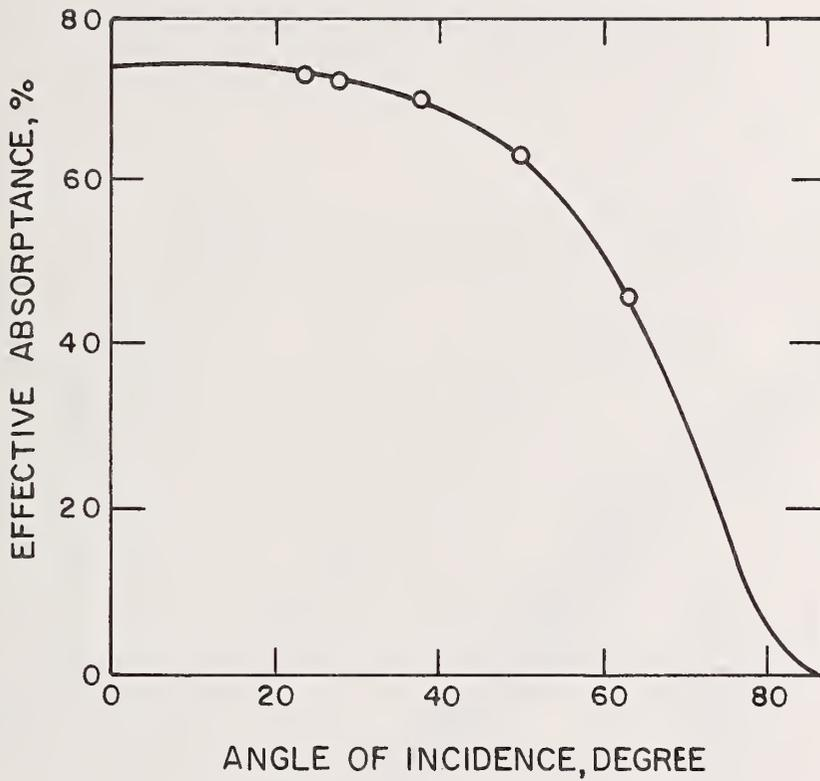
Figure 18 Effective Absorptance of a Double-Glazed Liquid-Heating Flat-Plate Collector as a Function of Incidence Angle [51]
