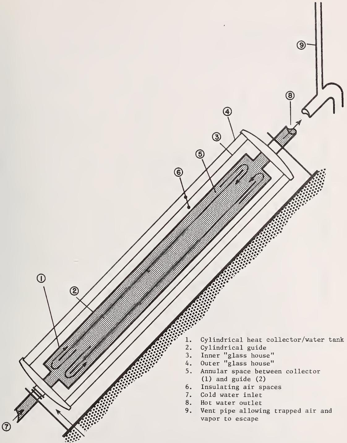
1. Cylindrical heat collector/water tank
