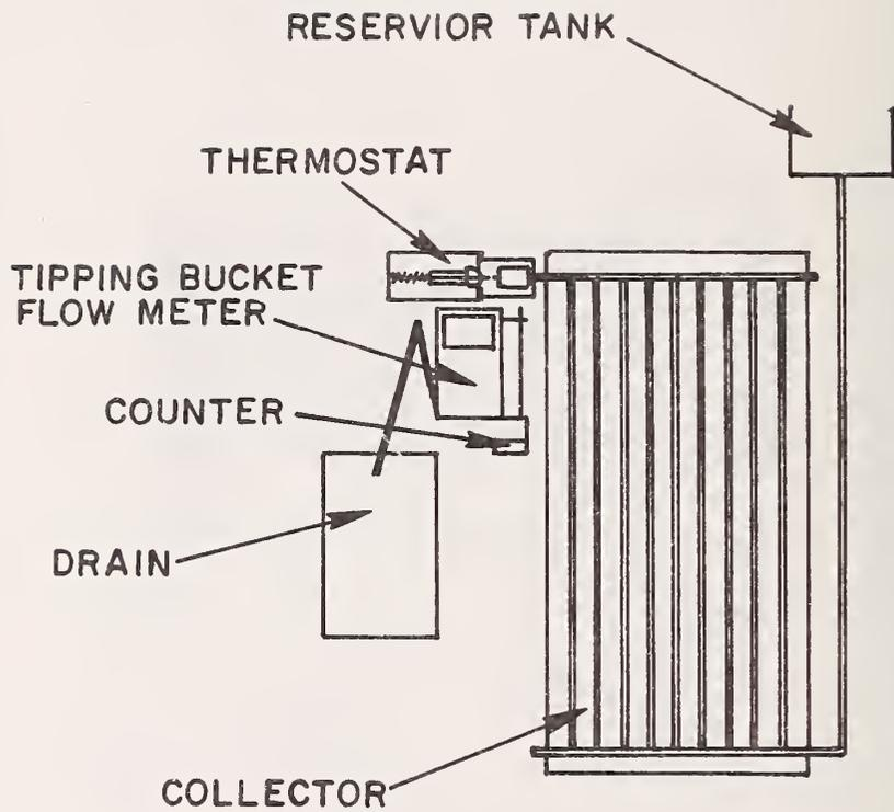
Figure 13 Apparatus Used by Doron [42] for Determining the Thermal Efficiency of Solar Collectors
