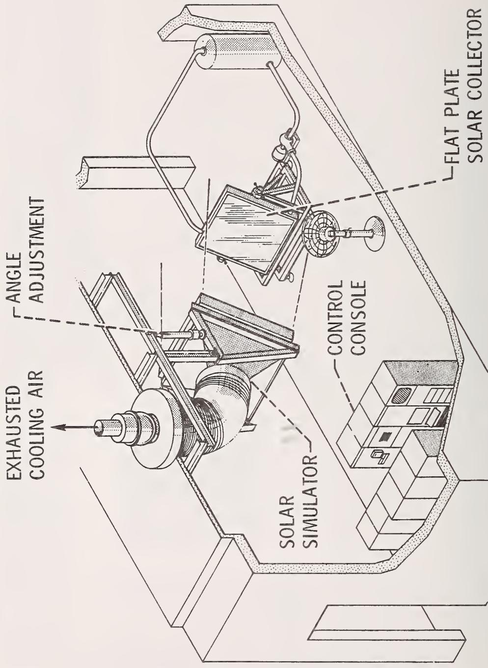
Figure 29 Schematic of the Indoor Solar Collector Test Facility at the NASA Lewis Research Center [29]
