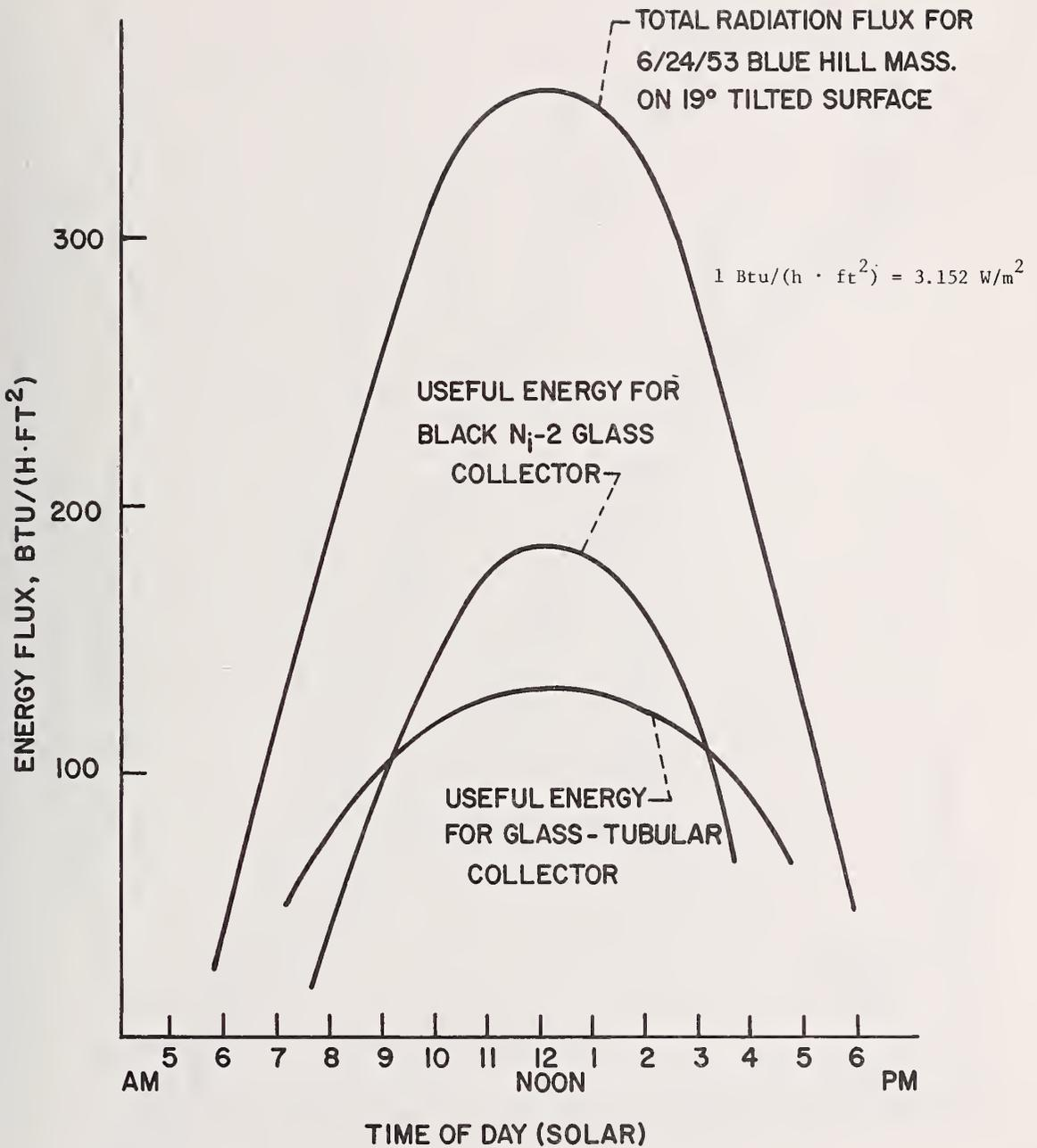
Figure 72 Predicted Daily Performance for an Evacuated Cylindrical Solar Collector and a Double-Glazed Flat-Plate Solar Collector, Both with Selectively Coated Absorbers [75]
