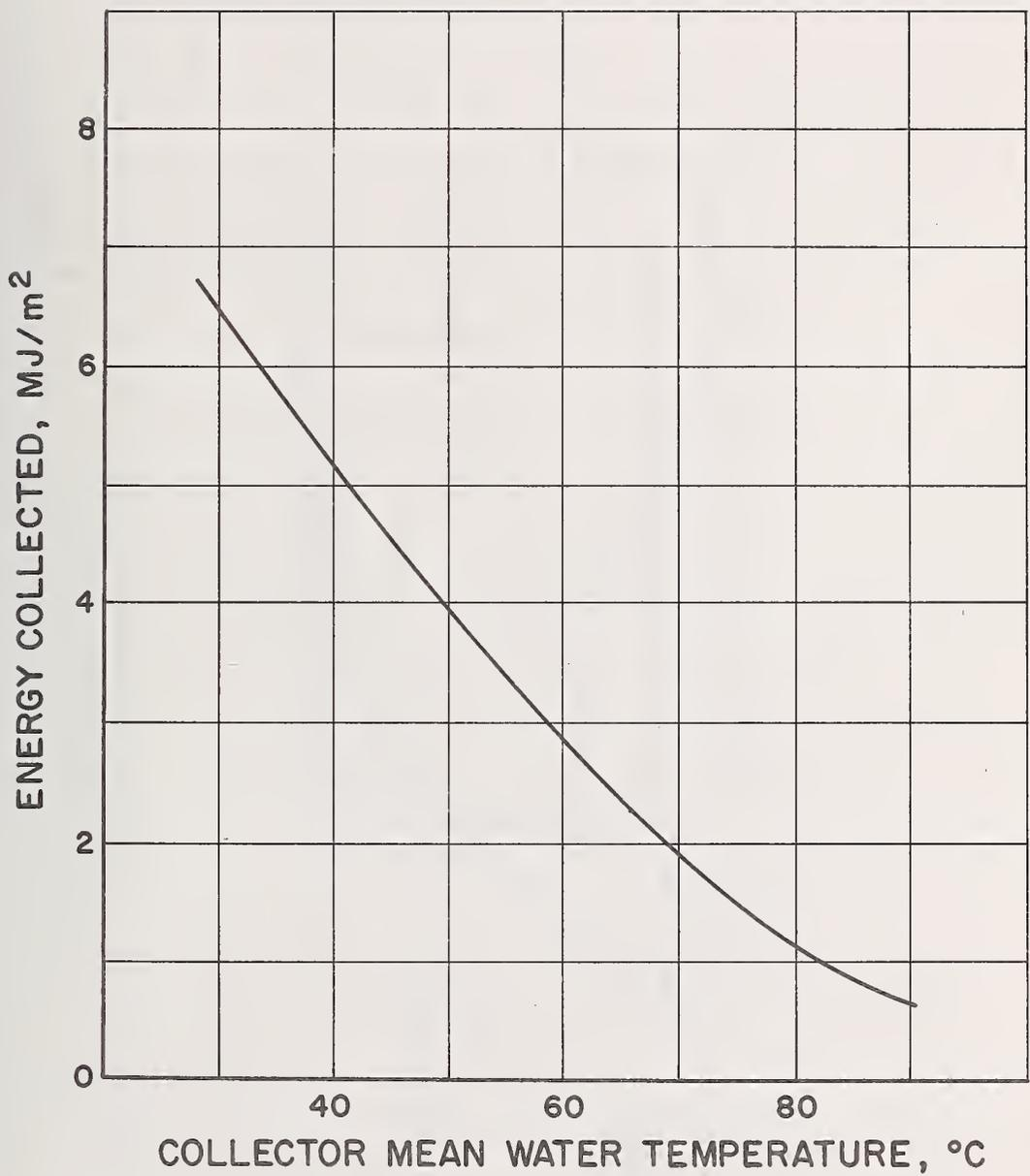
Figure 74 Daily Energy Collected as a Function of Collector Operating Temperature for a Single-Glazed Liquid-Heating Solar Collector in Australia [128]
