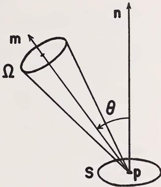
Figure C1. The Geometry for the Definition of Spectral Radiance.
