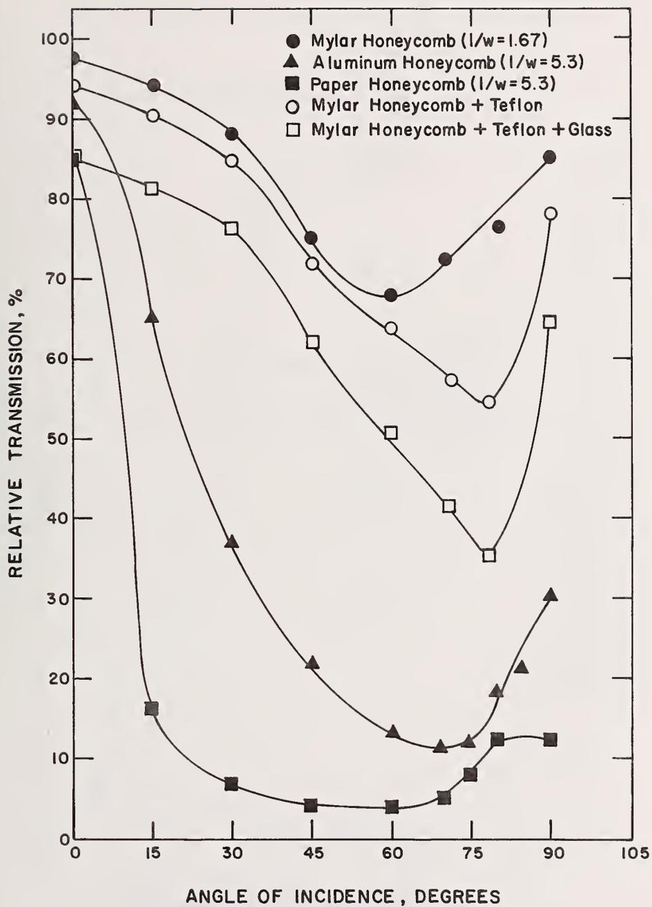
Figure 66 Relative Transmission of Selected Honeycomb Materials as a Function of Incident Angle[104]
