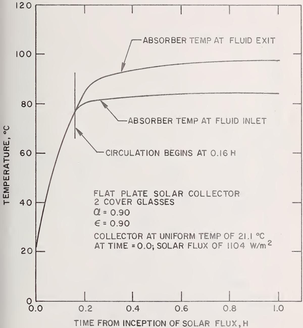
Figure 6 Thermal Response Characteristics of a Liquid-Heating Flat-Plate Solar Collector [19]
