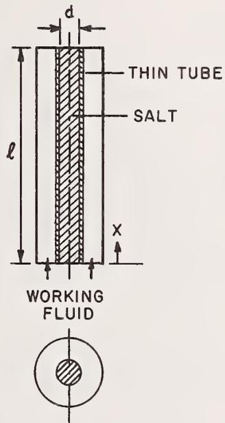
Figure B9 Schematic Representation of a Latent Heat-Type Thermal Storage Unit from Reference [14]
