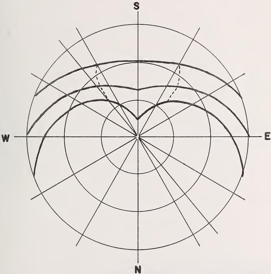
Figure C3. The Projection of the Path of the Sun through a Hemisphere Whose Polar Axis is Perpendicular to the Surface of the Earth at a Latitude of  $37^{\circ}$ .
