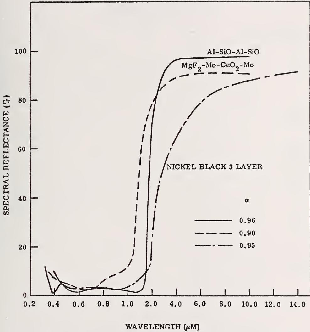
Figure 60 Reflectance of Spectrally Selective Coatings [98]
