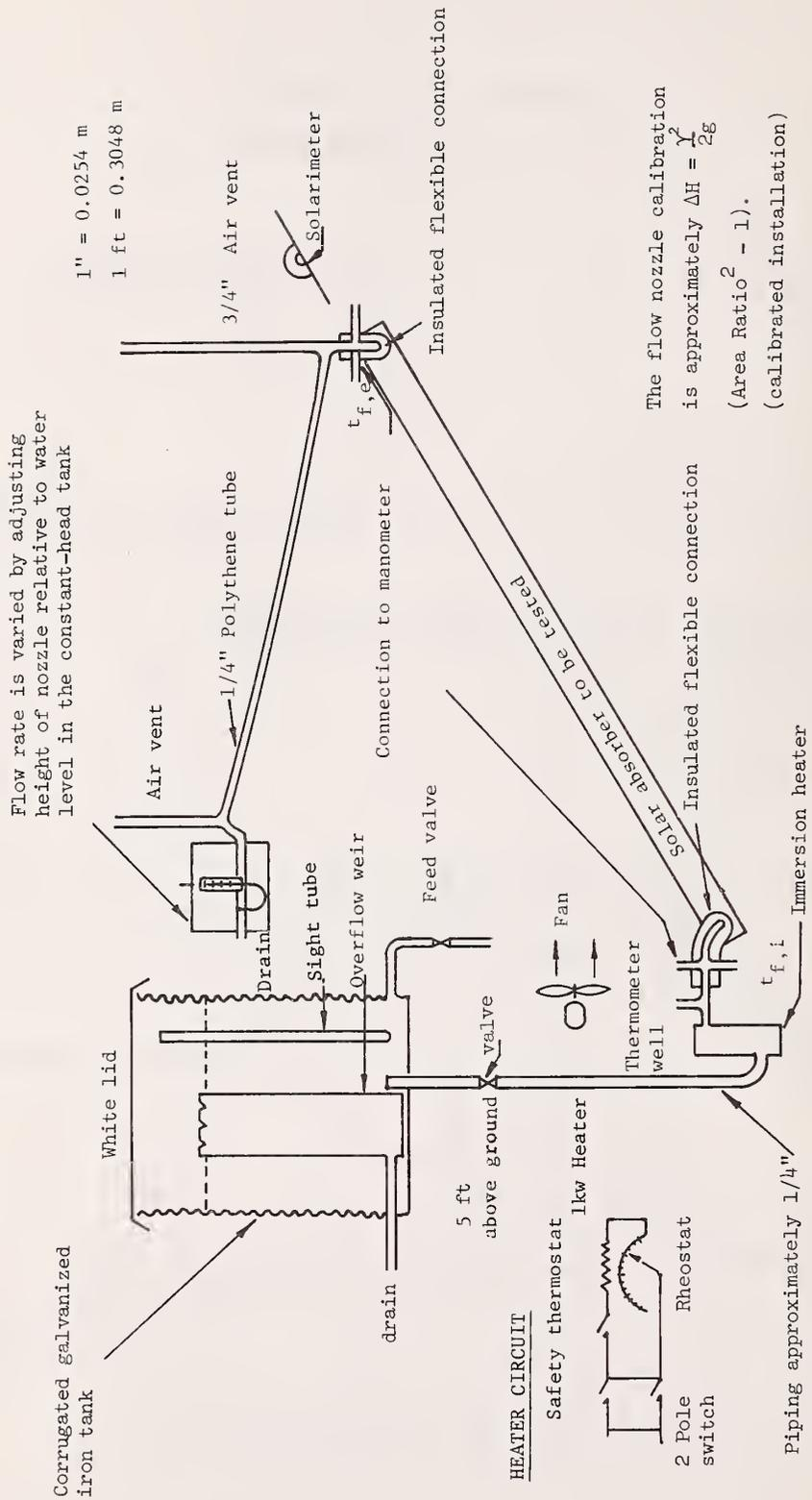
Figure 11 Apparatus Proposed by Whillier and Richards [31] for Determining the Thermal Efficiency of Solar Collectors
