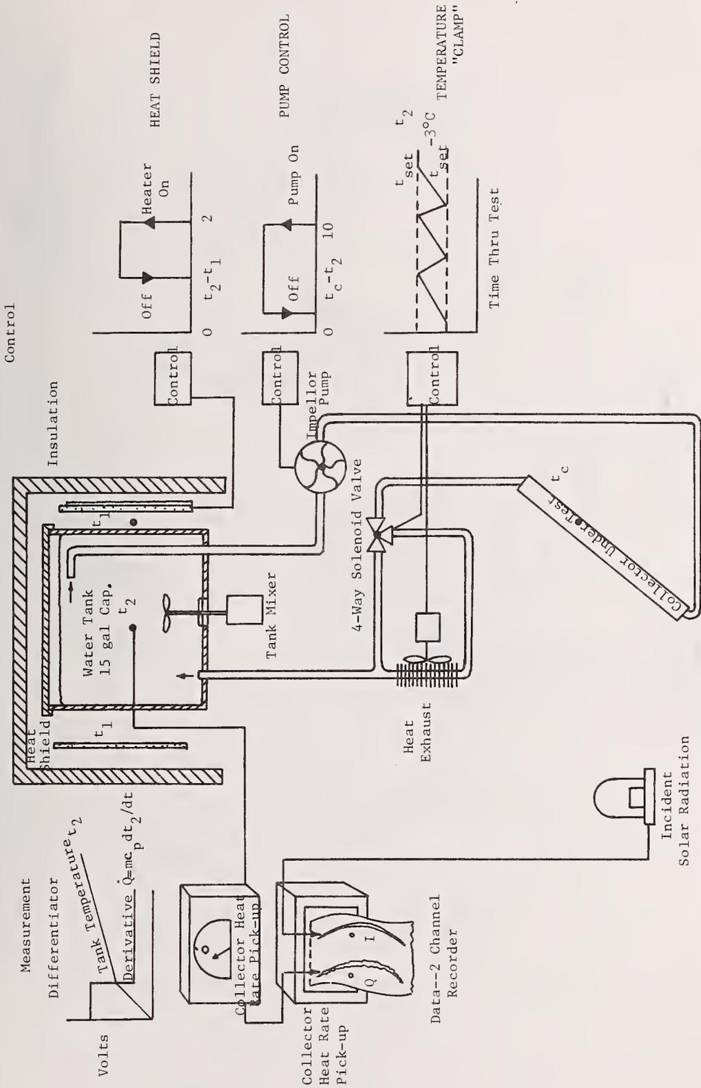
Figure 28 Schematic of the Arthur D. Little Calorimeter used for Determining the Thermal Efficiency of Solar Collectors [68]
