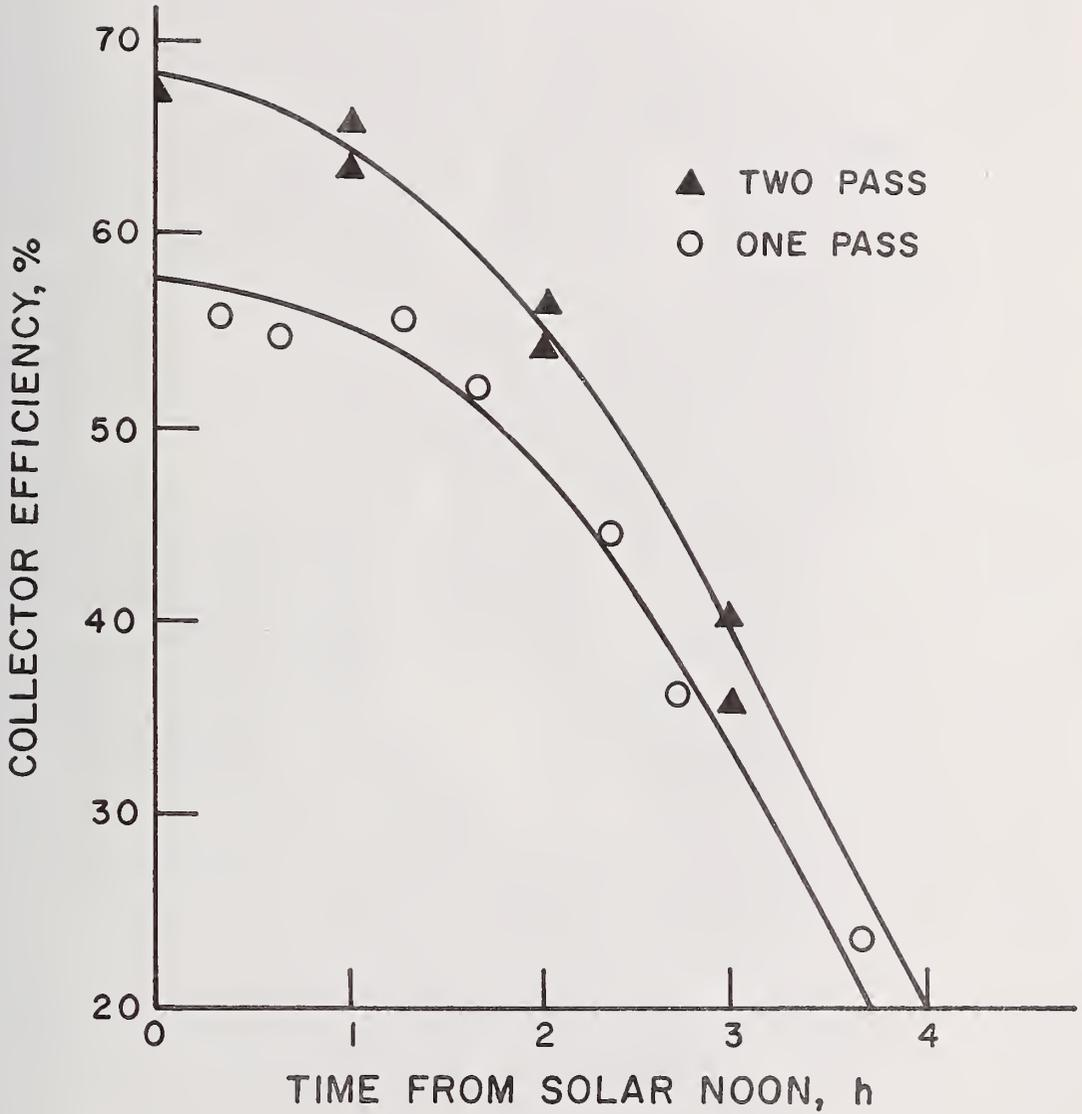
Figure 38 Thermal Efficiency as a Function of Time of Day for a One- and Two- Pass Solar Air Heater [89]
