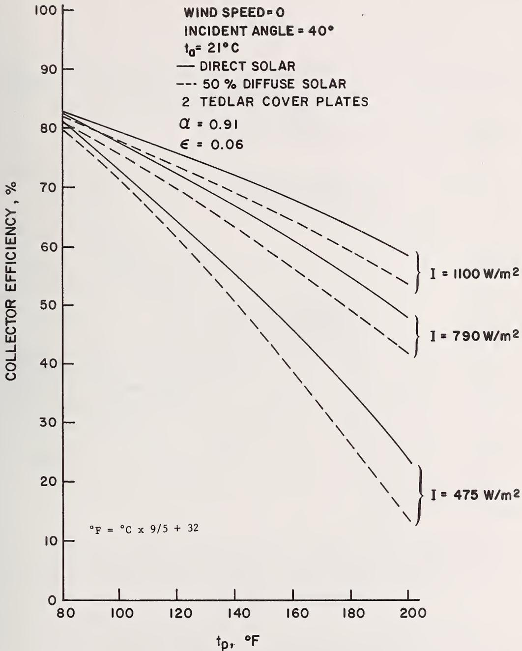
Figure 62 Comparison of Calculated Solar Collector Efficiency for Direct and 50% Diffuse Solar Radiation with the Sun 40° Off the Collector Normal
