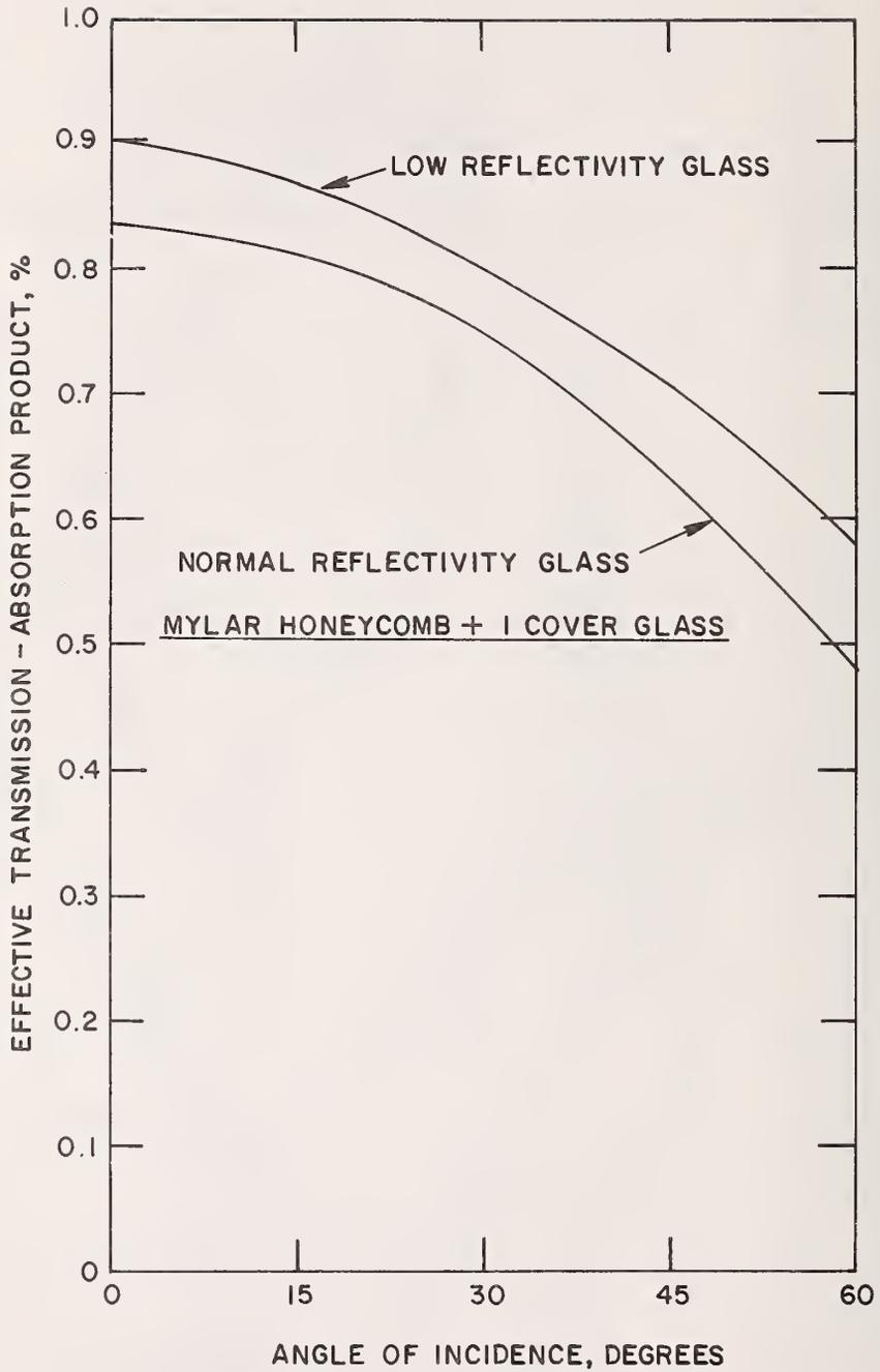
Figure 67 Transmission - Absorptance Product for a Single-Glazed Flat-Plate Solar Collector Incorporating a Honeycomb Convection Suppressor [17]
