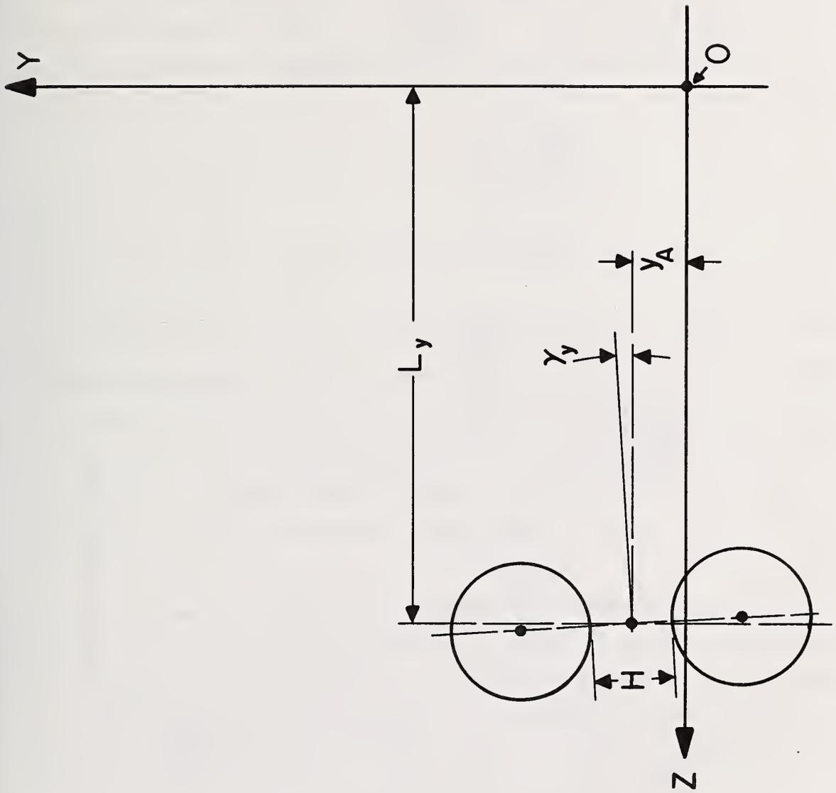
Figure 16. Coordinate system used in this report. In this view the X-axis is perpendicular to the plane of the figure. The circles at the left side of the figure represent the vertical aperture slits.
