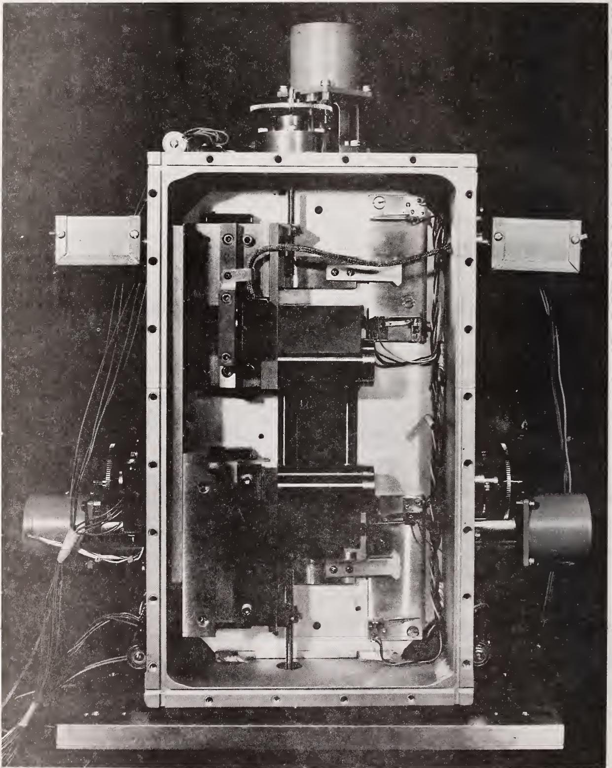
Figure 4. Photograph of Aperture Slit Assembly.
