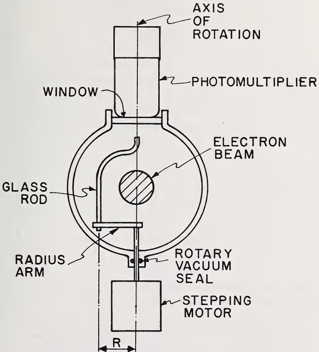
Figure 12. Upstream beam profile scanner.
