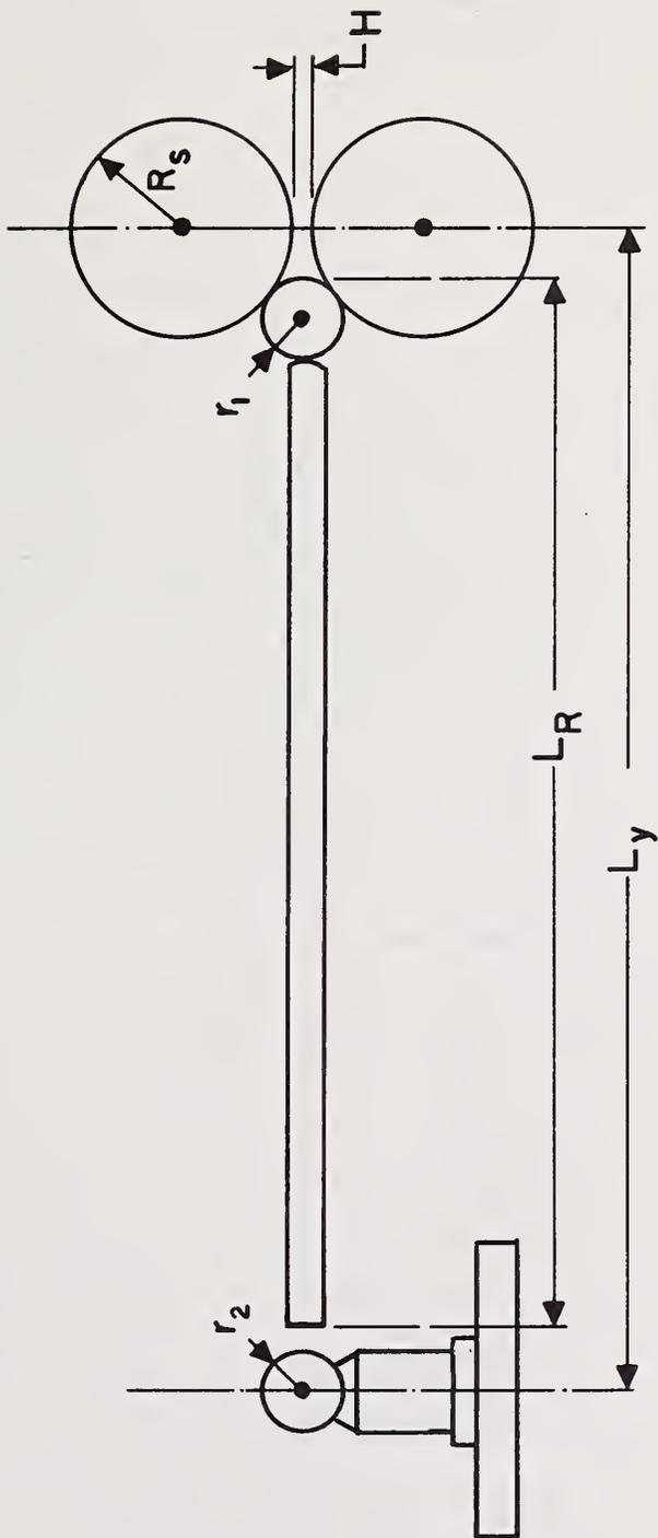
Figure 23. Setup for measuring  $L_y$ , side view.
