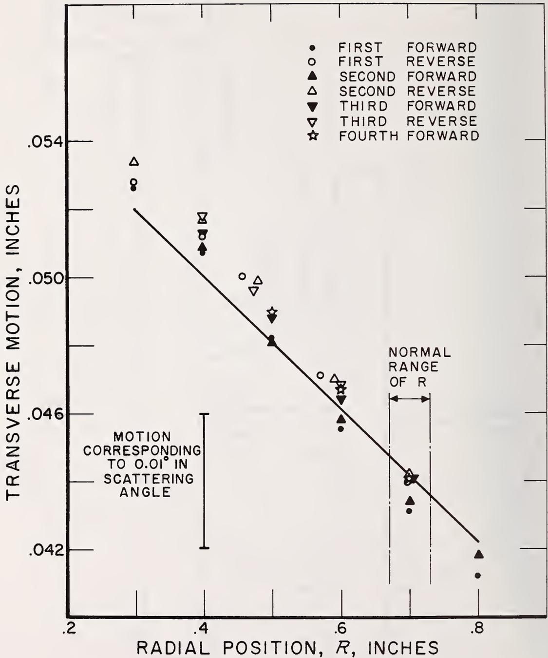
Figure 3. Transverse motion of spectrometer aperture accompanying radial motion. The solid curve indicates the motion predicted from the change of scattering angle with radial position.
