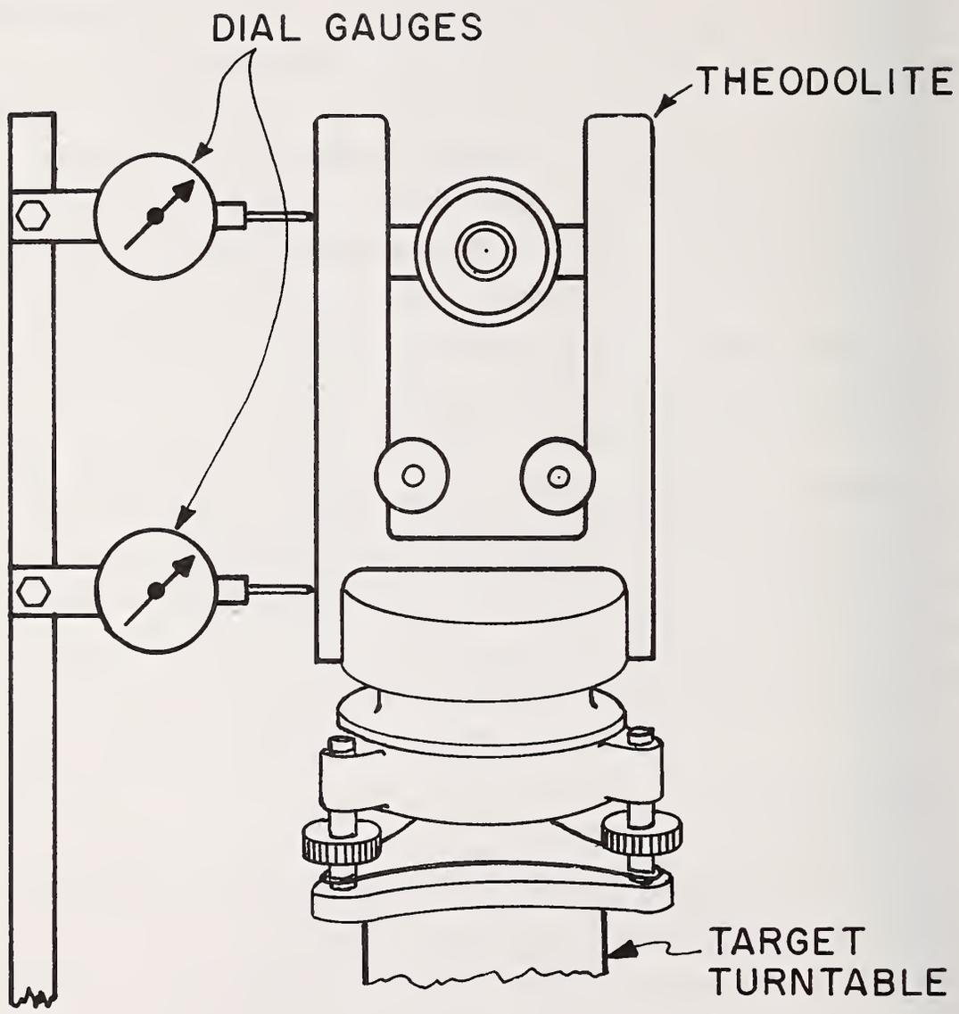
Figure 20. Setup for aligning the theodolite on the axis of rotation.
