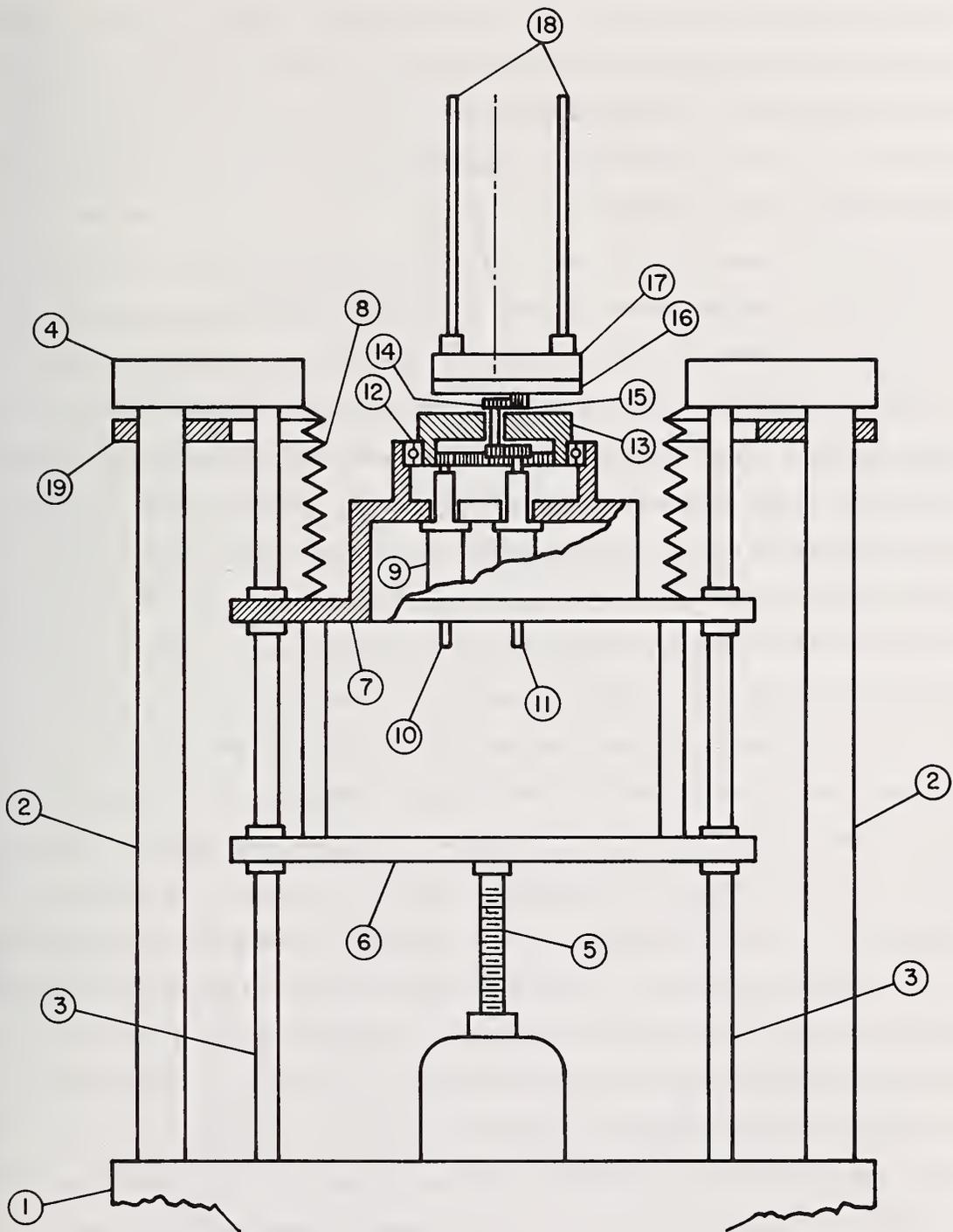
Figure 6. Target Pedestal Assembly. The components are: (1) base, (2) support column, (3) guide rods, (4) scattering chamber baseplate, (5) jackscrew, (6) jacking flange, (7) bellows flange, (8) bellows, (9) rotary feed-thrus, (10) rotation driveshaft, (11) oscillation driveshaft, (12) turntable bearing, (13) turntable, (14) linear cam, (15) idler wheel, (16) translation stage, (17) target platform, (18) target ladder roads, (19) indicator ring.
