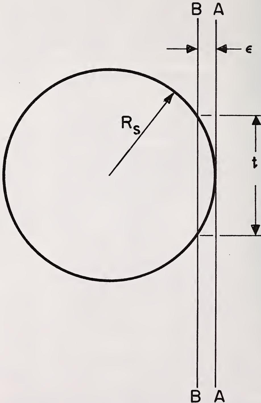
Figure 5. Illustration of slit-edge penetration effects.
