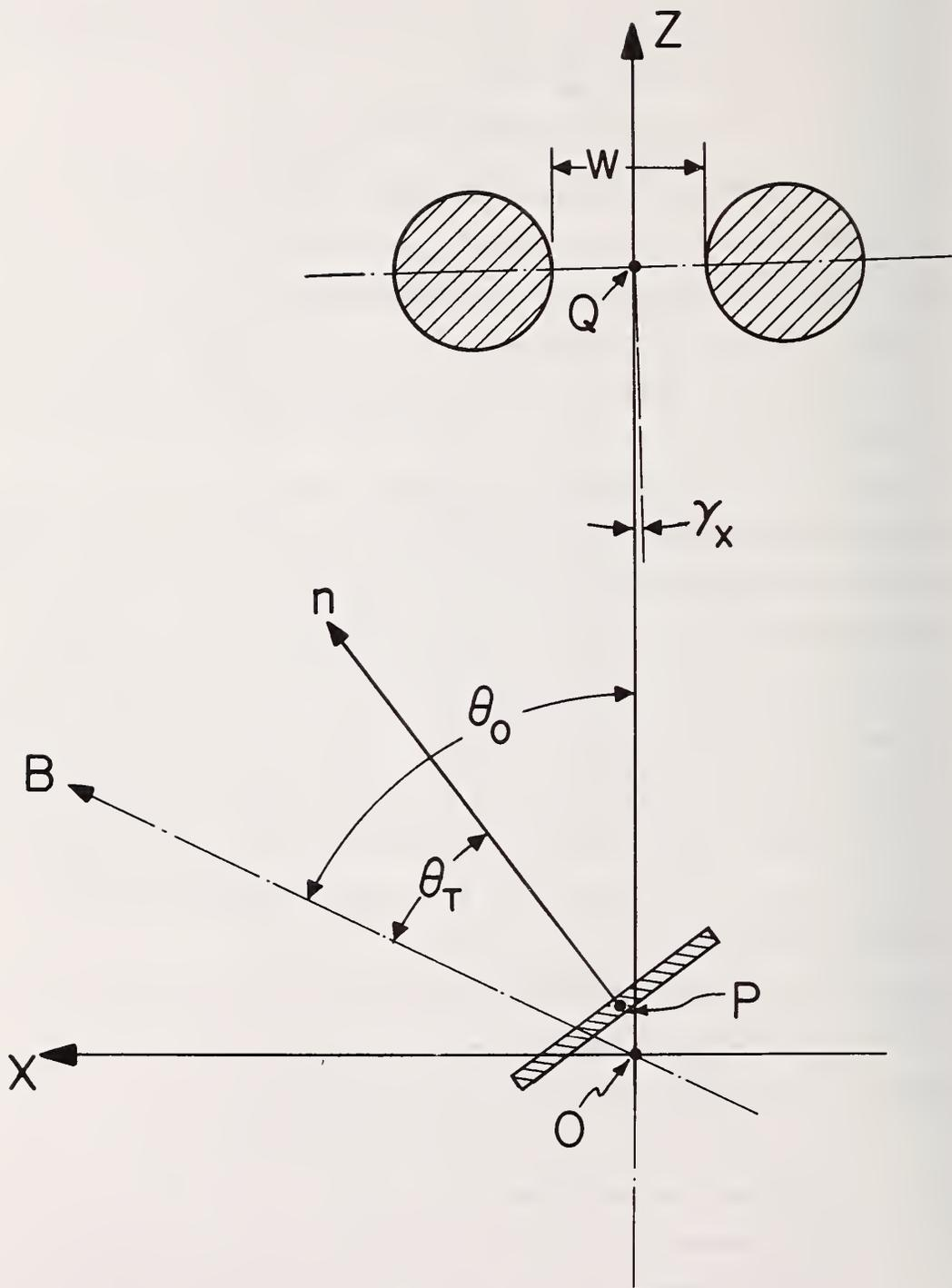
Figure 14. Coordinate system used in this report, in plan view. The shaded circles represent the horizontal aperture slits. The shaded rectangle represents a target oriented in transmission geometry. The line B indicated the beam direction.
