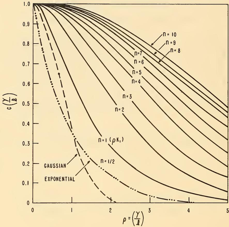
AUTOCORRELATION FUNCTION OF THE MODIFIED BESSEL FUNCTION
