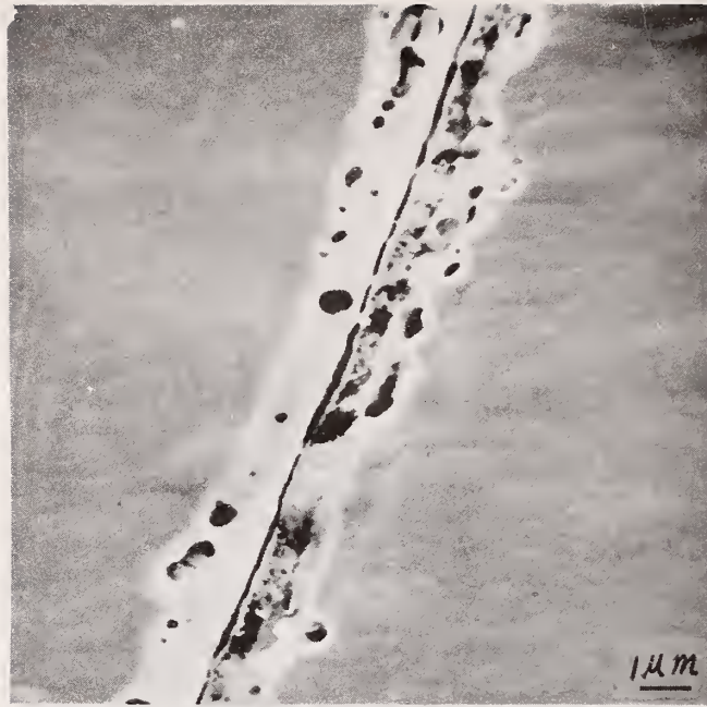
Figure 10 Evidence for chemical attack in nickel region associated with crack in test panel.
