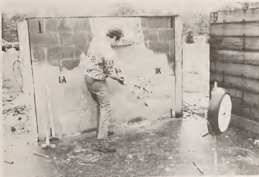
Figure 5. Spalling from Hole Pattern; Test 1K
