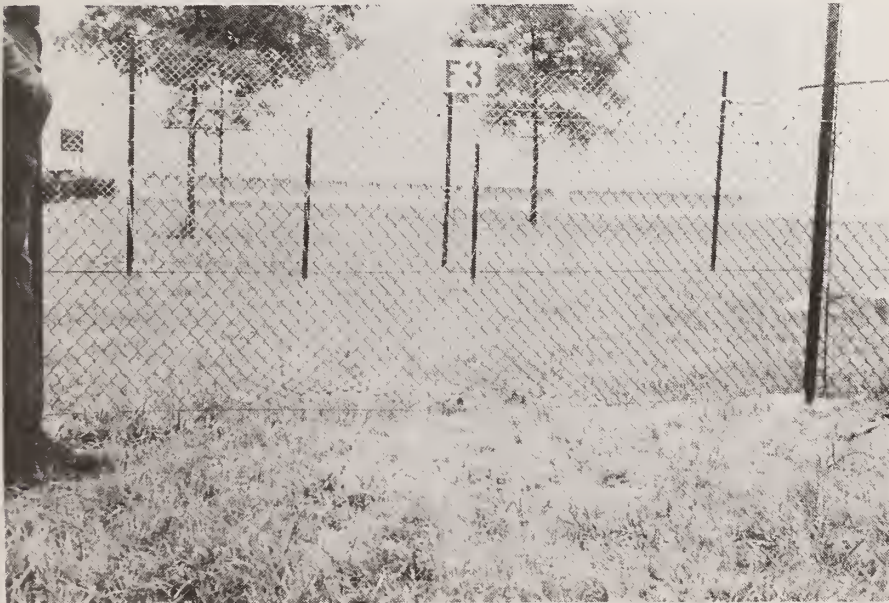
Figure 182. Appearance of Fabric after Dropping ; Test F3
