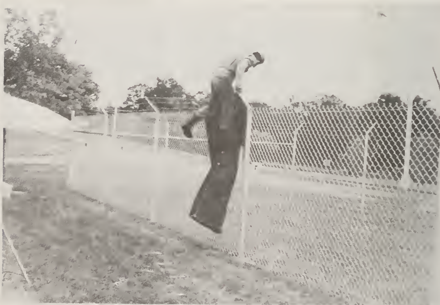
Figure 158. Climb Over Fence Using Tarpaulin as Protection against Barbed Wire; Test F1
