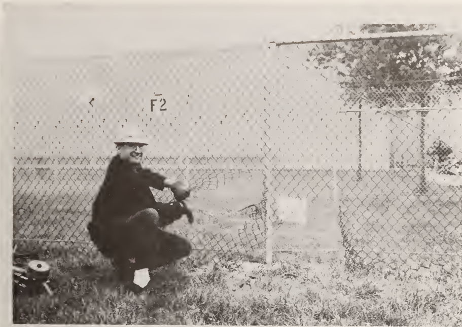
Figure 179. Opening Produced by Abrasive Wheel Saw; Test F2
