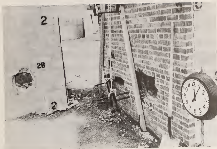
Figure 40. Test 5K. Battering Ram Suspended from A-Frame
