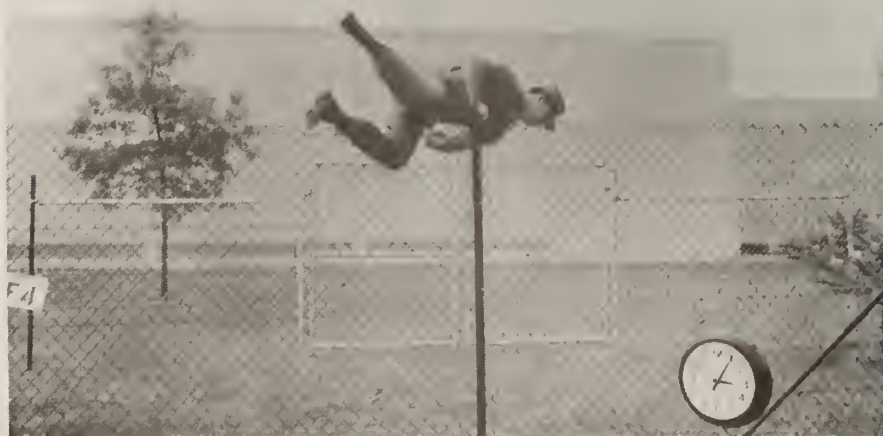
Figure 189. Climb Over Top of Fence; Test F4
