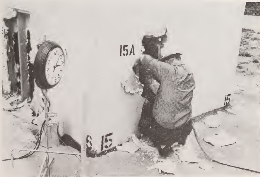
Figure 134. Test 15A. Cutting Steel Plate
