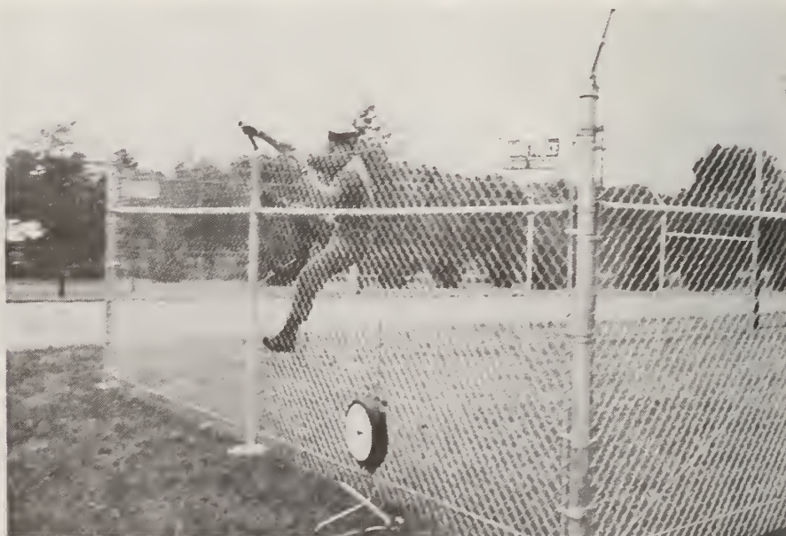
Figure 172. Gloved Hand Climb Over Started from Inside of Fence; Test F1
