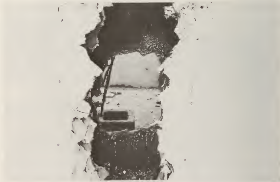
Figure 151. Hole Produced by Burning Bar; Test 16U
