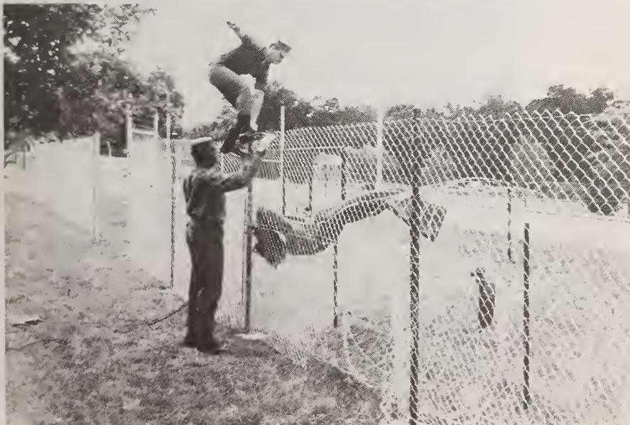
Figure 206. On Top of Fence Getting Ready to Jump ; Test F6
