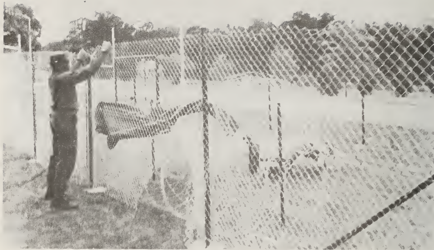
Figure 207. Leap Clearing Concertina Wire Using Tarpaulin as Safety Factor; Test F6
