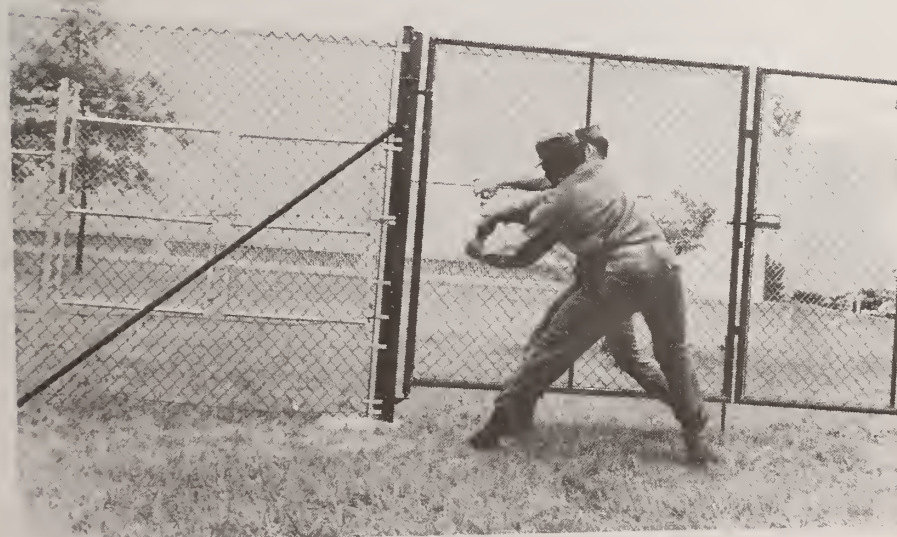
Figure 195. Pulling Metal Fabric Away from Frame; Test F4
