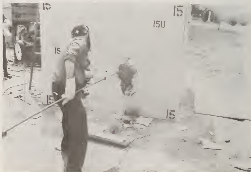
Figure 142. Test 15U. Cutting with Burning Bar
