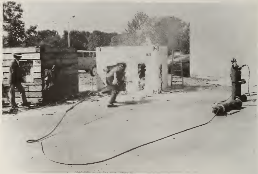
Figure 150. Burning Bar Cutting Through Steel Reinforcing; Test 16U
