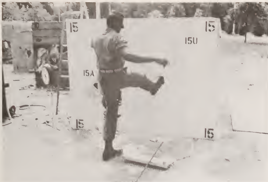
Figure 139. Test 15U. Kicking Out Plasterboard
