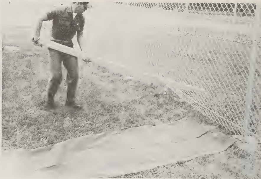
Figure 157. Fence Lifted 12" Using 2" X 4" Timber as Lever; Test F1
