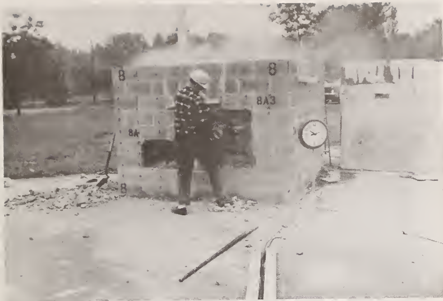
Figure 66. Test 8A3, Abrasive Wheel Saw
