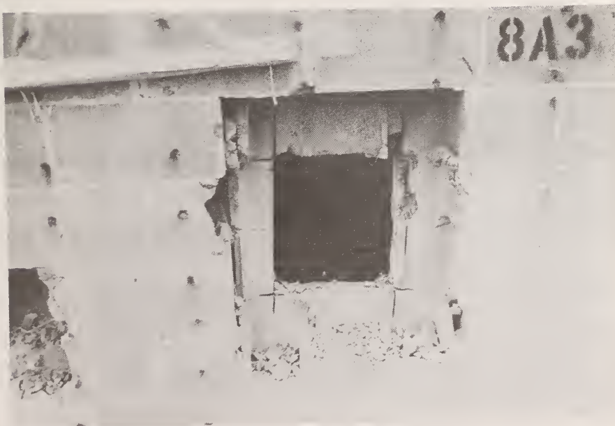
Figure 67. Opening Produced by 14" Abrasive Wheel Saw; Test 8A3
