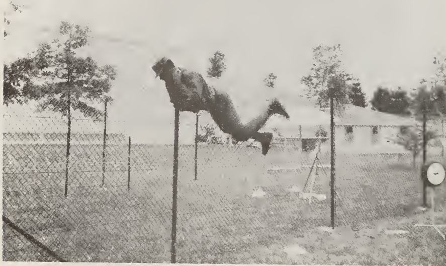
Figure 183. Climbing Fence Bare-handed; Test F3
