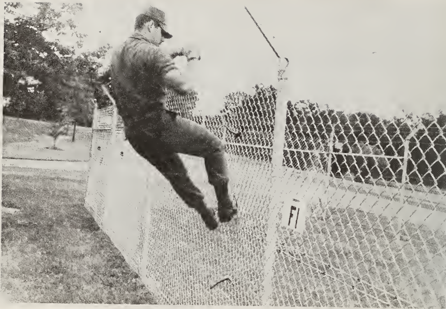
Figure 161. Climb Over Fence Using Linesman's Pliers to Make Steps; Test F1
