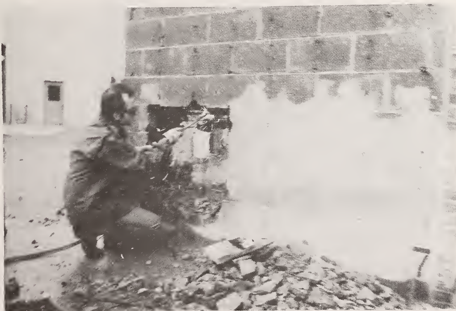
Figure 58. Test 7A. Cutting Wires with Torch for Time Comparison
