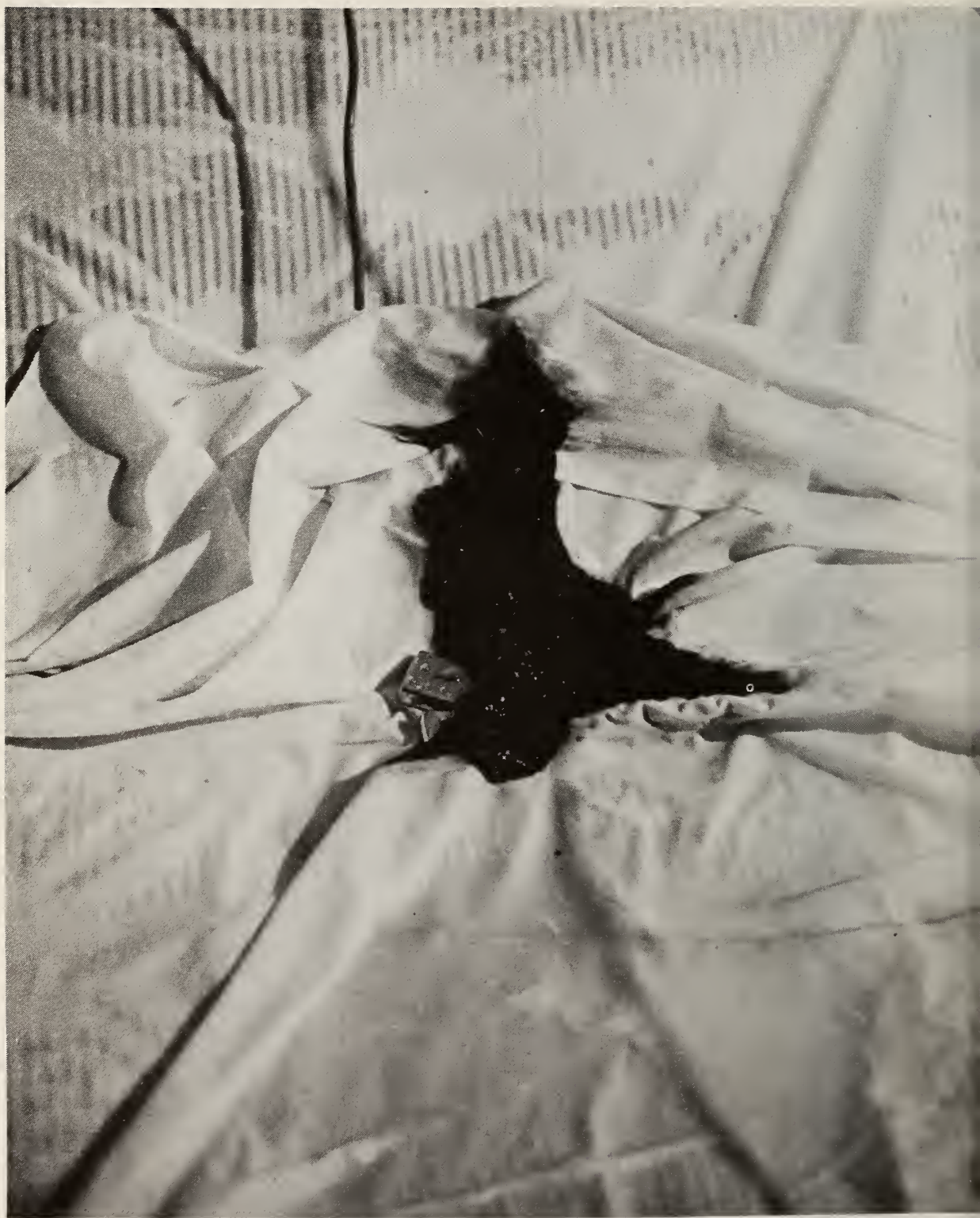
Figure 7. Flaming fire suppressed at 1 minute 45 seconds.
