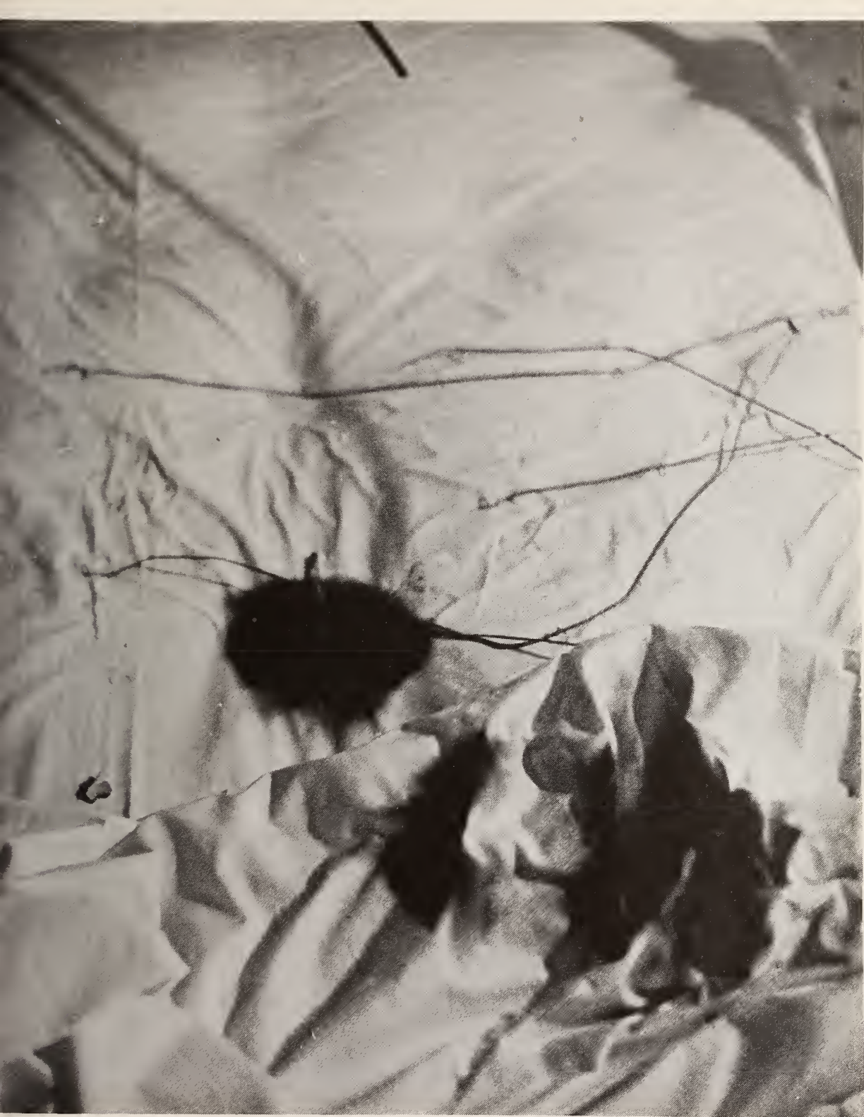
Figure 6. Smoldering fire suppressed at 22 minutes 46 seconds.
