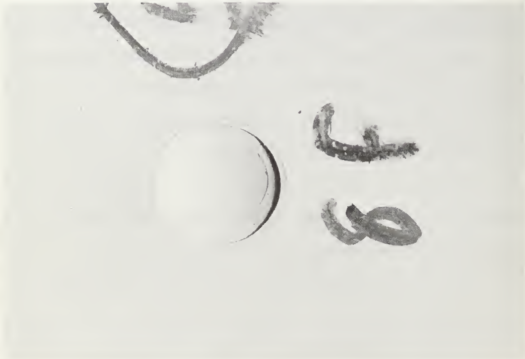
Figure 3. Supported impact test of urethane varnish applied on a painted gypsum wallboard substrate - Failure by cracking through the coating in the impact area at 8 in-lbf after room temperature curing.
