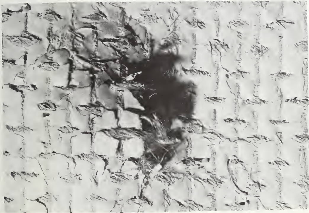
Figure 13. Unsupported impact test of gypsum impregnated jute fabric after room temperature curing (bottom view) - Failure at 1.4 in-lbf by tearing through reinforcement fibers.
