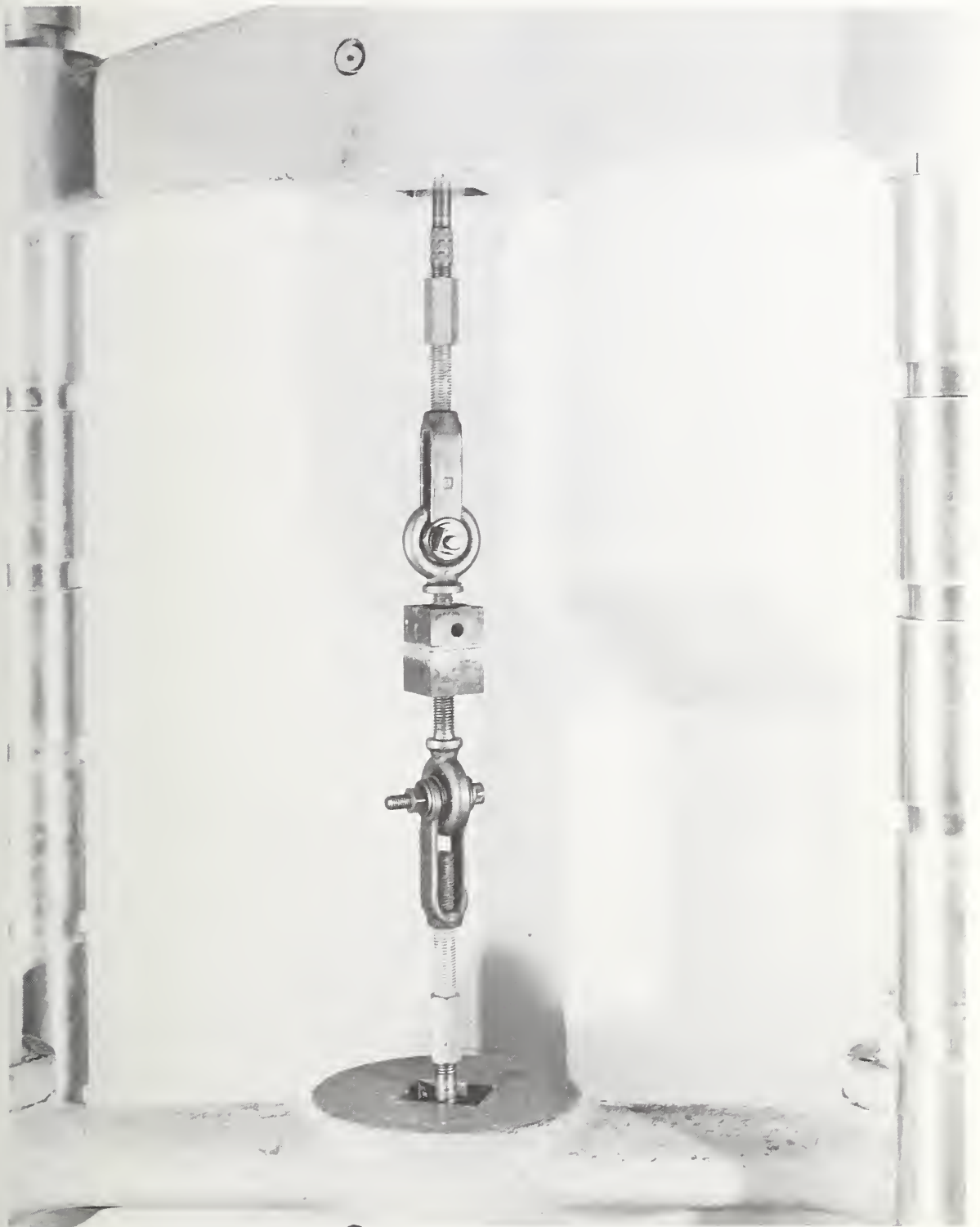
Figure A-2. Tensile bond adhesion test apparatus.
