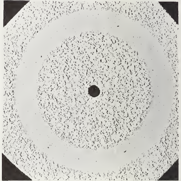
Figure 18. Abrasion wear pattern observed for the medium texture high build spray coating after testing.
