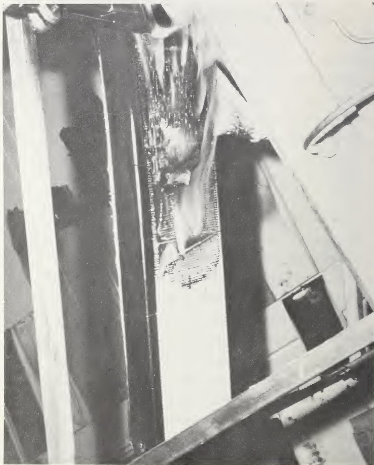
Figure 1. Flame spread test of gypsum impregnated jute fabric on a painted plywood substrate - Open flaming.
