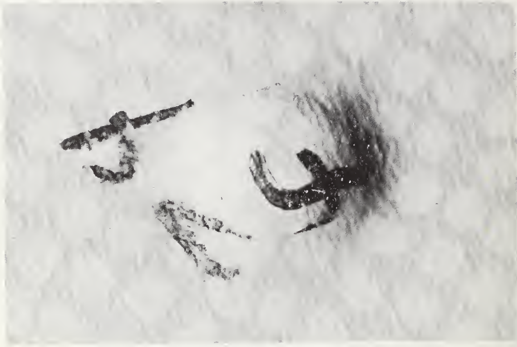
Figure 8. Supported impact test of medium duty vinyl wall covering applied on a painted gypsum wallboard substrate - Failure at 74 in-lbf by tearing through the reinforcement fabric after room temperature curing.
