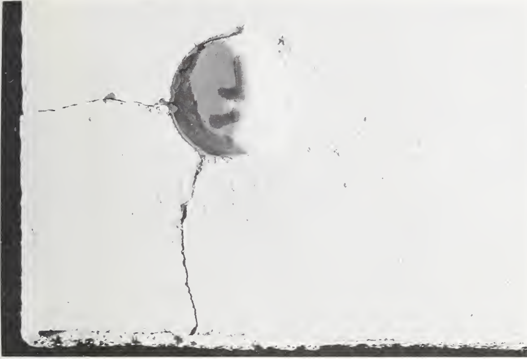
Figure 6. Supported impact test of veneer plaster applied with a bonding agent on a painted gypsum wallboard substrate - Failure by cracking and delamination of the plaster outside the impact area at 80 in-lbf after room temperature curing.
