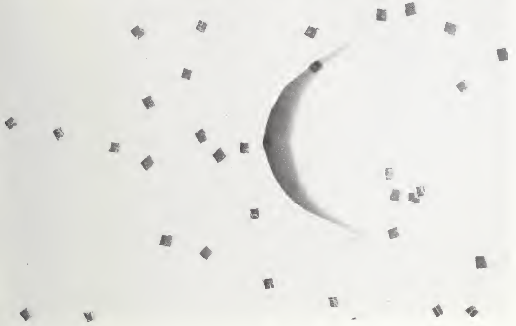
Figure 14. Unsupported impact test of vinyl counter top material after dry heat aging - Failure at 26 in-lbf by tearing through the covering (no stretching).
