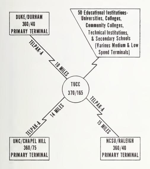
Note: In addition to the primary terminal installation at DUKE, UNC, and NCSU, each campus has an array of medium and low-speed terminals directly connected to TUCC.
