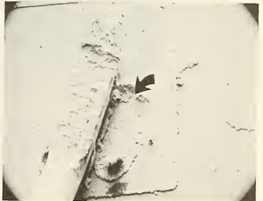
Figure 16. A probe mark on a bonding pad. Note where the probe has completely scraped through the metallization as indicated by the arrow. Magnification: 560X
