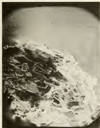
Figure 11 Scanning electron micrographs of set gypsum plasters with: a. 0.8g \text{NH}_4\text{C}_2\text{H}_3\text{O}_2 (X 1100); b. 0.2g succinic acid (X 1330); c. 0.2g tartaric acid (X 2600) d. 0.1g gelatin (X 500).
